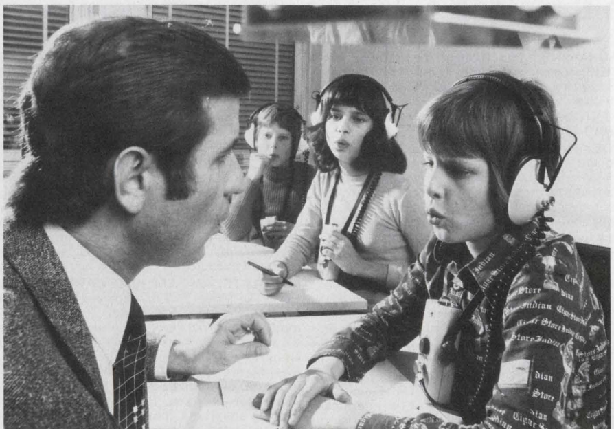
Infrared speech/hearing aids enable hard-of-hearing students to converse with one another. A built-in optical system provides optimum reception.
