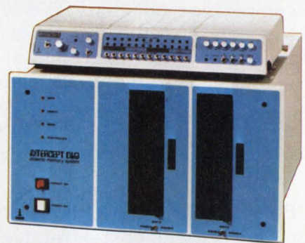
The 6100-based dual-floppy disc system from Intersil offers a file system, monitor, text editor, assembler, binary loader, octal debugger, high-level interpreter and utilities.
