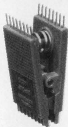
Model 4236 14/16 Pin For Ultra Dense Packaging
