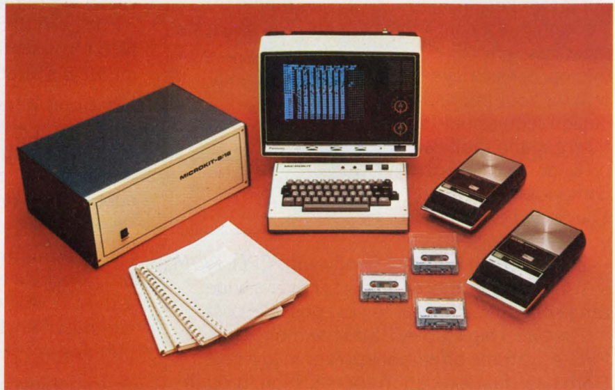
Low-cost cassette tapes and CRT monitors can be used by such development systems as this one from Microkit, Santa Monica, CA. Important to any software-development system, however, is the support literature for the programs.
