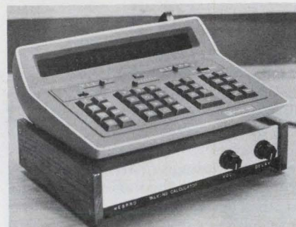
The readouts of a Monroe 1920 calculator are deciphered by a \mu P to control a 35-word vocabulary in this Wespro talking-calculator system.
