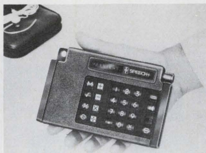
A vocabulary of 24 words is designed into this talking calculator for the blind by Telesensory Systems.
