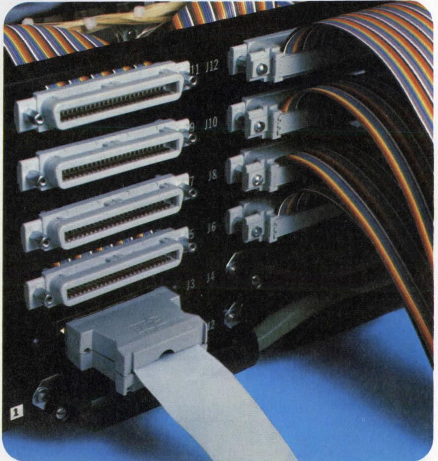
With Scotchflex Delta Ribbon Connectors, no stripping, soldering or other wire preparation is necessary. You can mass terminate a parallel-lay 50-conductor (25-pair) .0425" center-spaced flat cable in less than 30 seconds with one step. That's about ten times faster than other available methods. And thanks to 3M's field-proven, gold-plated beryllium copper U-contacts,
