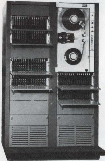
Besides this 28-track model, Bell & Howell's Data-tape Division, Pasadena, CA, supplies 42-track digital instrumentation recorders with packing densities of 33,000 bpi, data throughput rates of 150 Mbits/s, and error rates of one bit in 10-billion.
