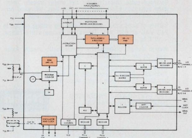
The architecture of the PPS-4/1 devices resembles that of a complete minicomputer—all the necessary circuits are included on a single chip. All chips except the MM77 and 78 have a  $48 \times 4$  bit on-board RAM. The 77 and 78 contain  $96 \times 4$  and  $128 \times 4$  RAMs, respectively. All chips have one 8-bit bidirectional port as well as two conditional interrupt lines, except for the MM75 which has only one interrupt.
