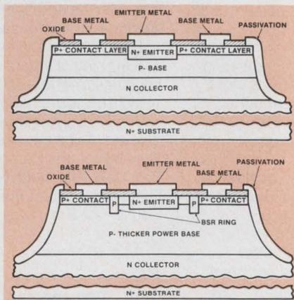
**Power-base transistors** (bottom) are constructed very much like conventional epitaxial devices (top).
