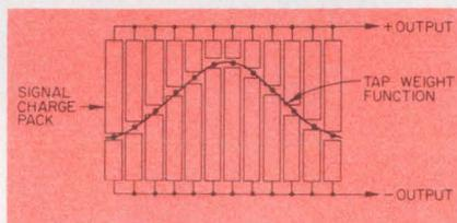
This split-electrode structure forms capacitors that hold the tap-weight function. Analog charges induce product currents that are summed and fed to differential amplifiers.
