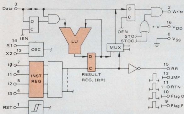
A minimum system consists of the processor, an external memory, program counter, 8-channel data selector and an 8-bit addressable latch. Instruction lines are TTL compatible and the 1-bit bi-directional data line has three-state capability. On-chip there are three 1-bit registers that are directly addressable, and the clock oscillator.
