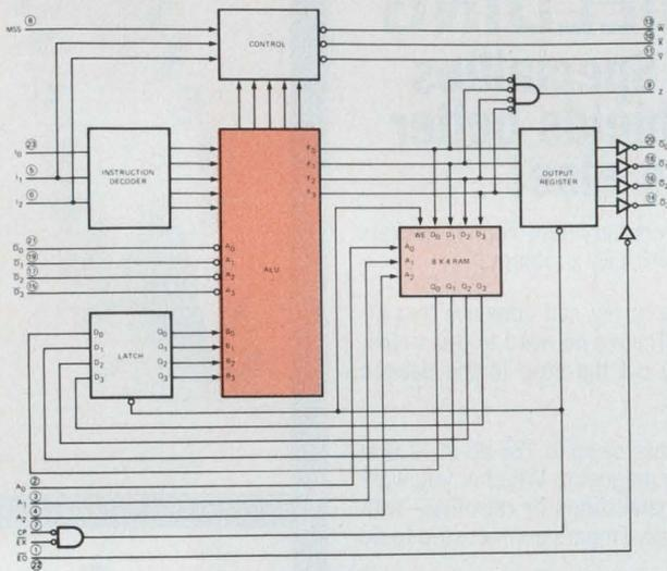
The architecture of the Macrologic slices is such that the chips can be cascaded to make an  $n \times 4$  bit processor. Carry outputs are provided for carry-lookahead operation and three status signals are also available—accumulator zero, negative or overflow. The four data output lines have three-state capability. A minimal system is hard to define, but a typical organization might use 30 to 50 chips.
