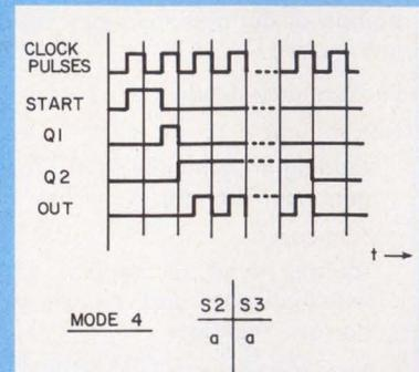
Four modes of testing can be obtained by setting switches  $S_2$  and  $S_3$  in the four possible position
