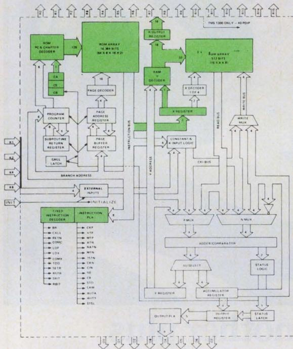
The architecture of all the TMS1000 products is very similar, with the main differences appearing in the size of the RAM and ROM and the number of I/O lines. All processors have an internal clock generator, but can accept a single-phase clock signal if timing must be generated externally. Just the single chip is needed to form a minimal working system.
