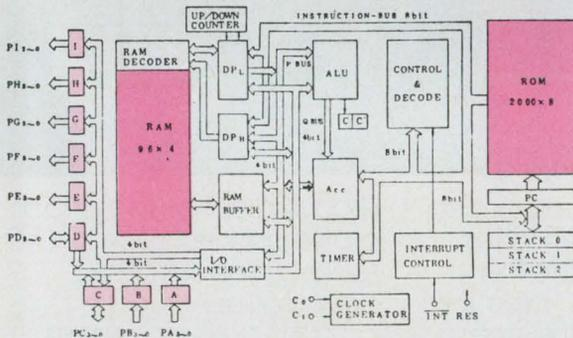
The architecture of the uCOM 43, 44 and 45 all-in-one processors is the same except for varying amounts of ROM and RAM. All chips have an on-board clock circuit and have TTL compatible I/O lines. The largest circuit, the 43, has an on-board programmable timer, a three-level stack, a flag register and six working registers. The I/O ports are divided as follows: two 4-bit input ports, two 4-bit I/O ports, four 4-bit outputs and one 3-bit output.
