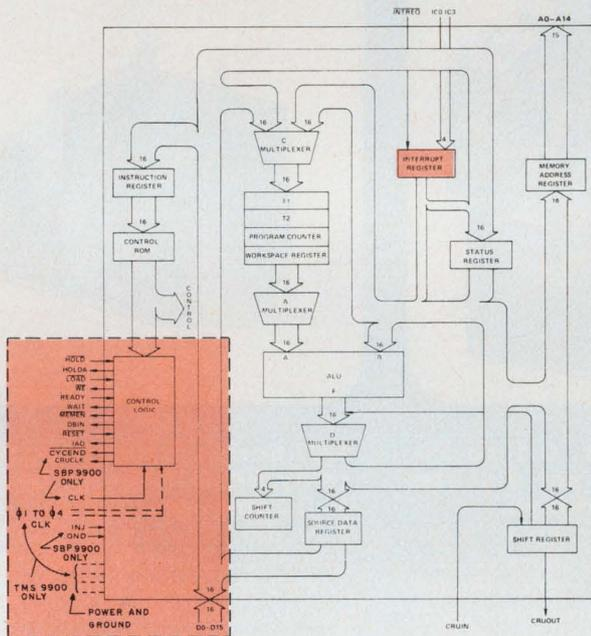
The 16-bit memory-to-memory architecture of the 9900  $\mu$ Ps permits flexible register files to be set up in memory. A minimal system consists of the CPU, a clock generator and the necessary memory.
