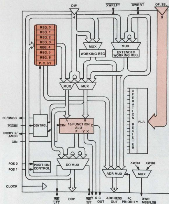
The architecture of the processor slice provides separate data in, data out, address out and control ports, as well as a 16 function ALU. On the chip are an eight-word general register file, two 4-bit working registers, dual scaled-shifters (with on chip handling of end conditions) and a factory programmable logic array that generates on-chip control signals. A minimal system is hard to specify since it depends on word size and control options. A typical system might contain 30 to 50 chips.
