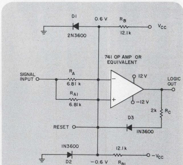
**A positive analog input provides a positive logic-level output that remains after the signal passes. Similarly, a negative input provides a remembered positive-level output.**
