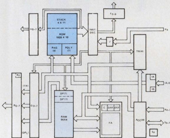
The architecture of the uCOM-42 is designed directly for the electronic cash register market and keyboard controllable appliances. The I/O structure handles an 8 × 4 keyboard, an 8-digit LED display and peripherals. The on-board RAM can also be expanded off the chip. All I/O lines are TTL compatible and all outputs can handle up to -35 V.
