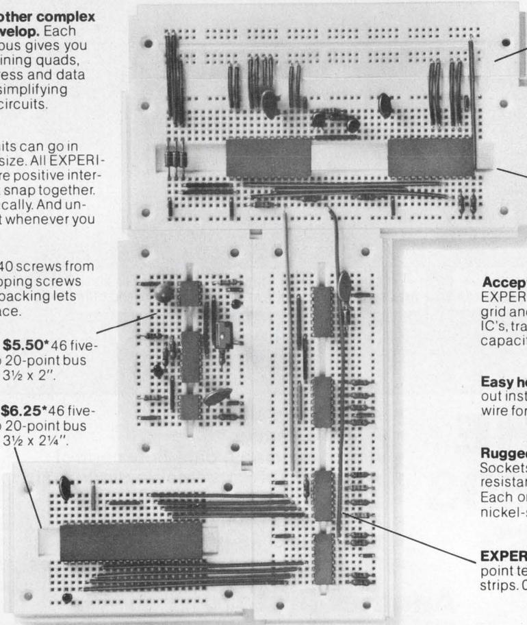
**EXPERIMENTOR QUAD BUS STRIP \$4.00\*** Four 40-point bus strips. 3/8 x 6 x 3/4".
