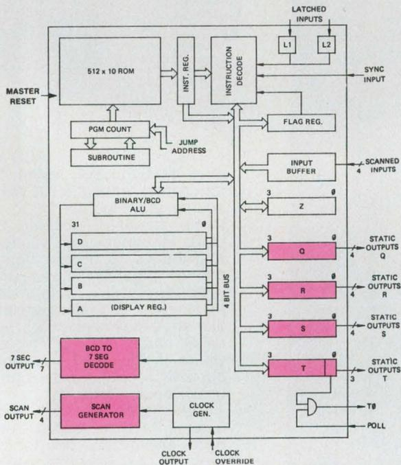
The stand-alone processor has scanned inputs and decoded outputs: seven input lines, 16 output lines, and LED segment driver outputs. All lines are compatible with TTL or CMOS logic families. In addition to the 512 × 10 bit on chip ROM, the 1872 has a 32 × 4 bit scratchpad RAM and on-board clock generator.
