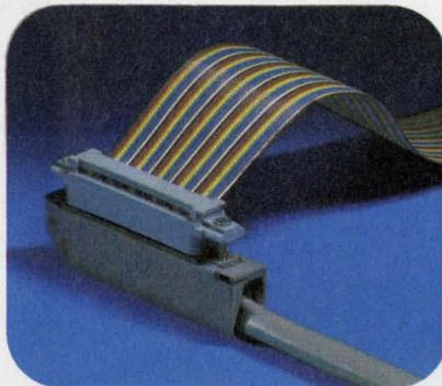
The Scotchflex Delta Ribbon system includes 50-position male and female connectors, plus appropriate bail mount, screw mount and jack screw kits, strain relief clips and dust covers. Color-coded flat cable is available in parallel-lay conductors #28 AWG stranded or #26 AWG solid.
