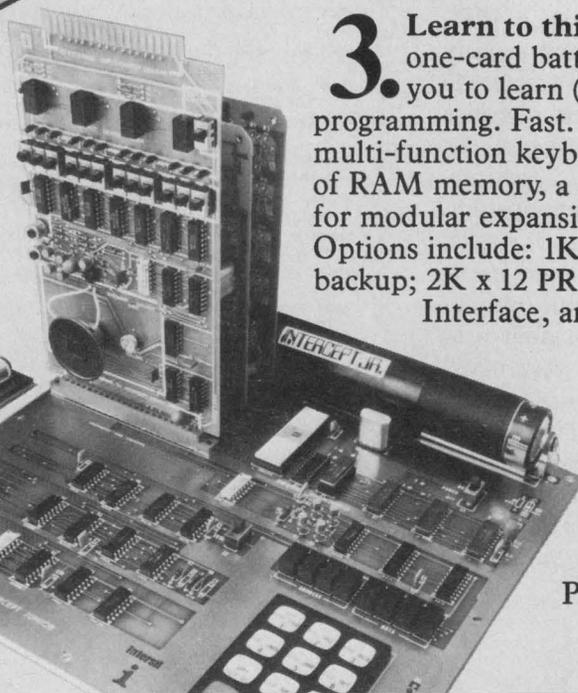
**4.** Prototype your systems in CMOS. \$2,850. With the Intercept Prototyping System. A complete microcomputer development system that includes 4K words of CMOS memory with on board battery backup. Prototype systems. Develop software.
