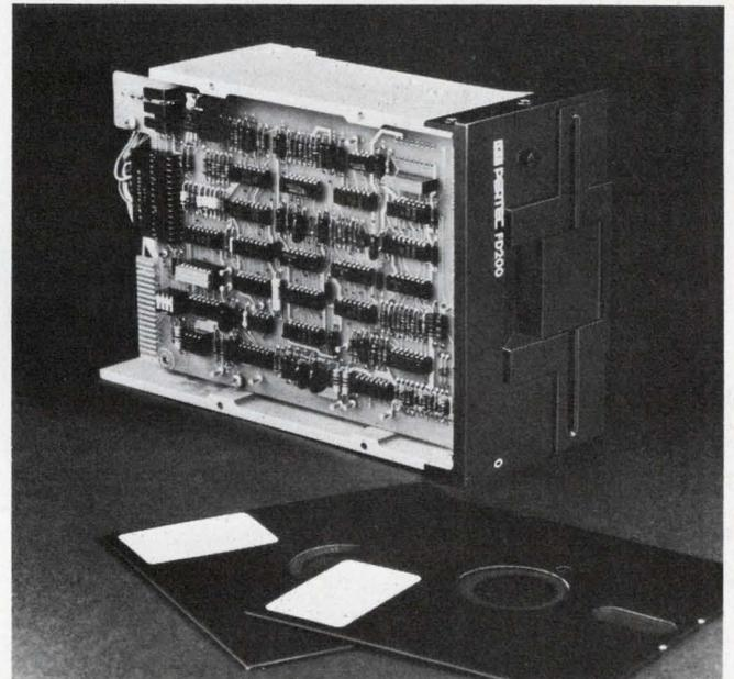
**A micro-sized drive (top)** from MPI is the only minifloppy to use a metal-band actuator. Its track-to-track time is 5 ms. Pertec's micro-sized floppy (bottom) boasts the same dimensions, mounting holes, interface signals, and voltage requirements as the Shugart SA400.
