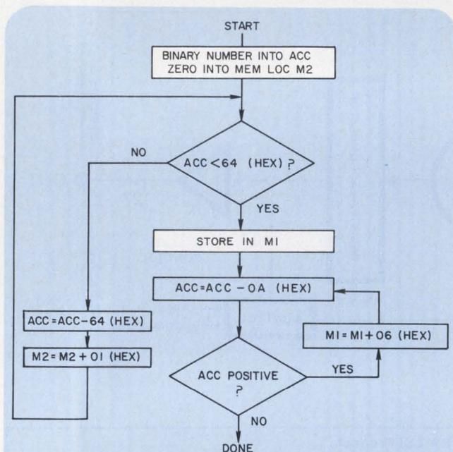
When the binary-to-BCD conversion is complete,  $M_1$  contains the tens and ones digits within a single byte in BCD, while  $M_2$  contains the hundreds digit.
