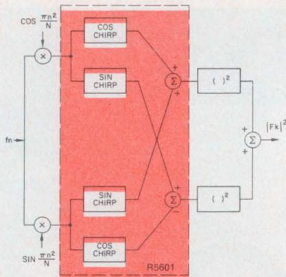
A CZT (chirped-Z transform) algorithm is implemented with external components in addition to the four transversal chirp filters of the R5601.
