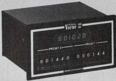
**DUAL PRESET UP/DOWN COUNTER** Two presets, large LED display, and operation from a variety of electromechanical and electronic sensors highlight Vorne's Model 215-DUAL. Plug-in relay or solid state output options are available with the 2-5/8 h x 3-1/8 w x 4-1/4" d, 115 VAC operated unit. Priced from \$208 (25 quantity). Vorne Industries, Inc., 5023 West Belmont, Chicago, IL 60641 (312) 725-3077.
