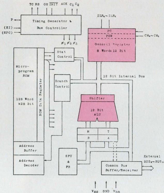
The T3190 has a three-state data/address bus and an eight-word register stack. The minimum system requires a processor, the MM111C RAM, TMM121C PROM, T3416 memory control unit, T3418 I/O control unit, and a 3220 general-purpose I/O register.
