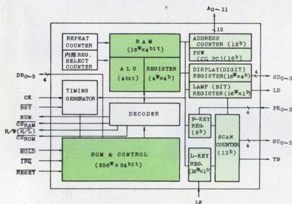
The architecture of the T3472 is oriented for binary and BCD data manipulation and display. All I/O lines are TTL compatible and the data bus has three-state capability. Display control logic and the clock as well as the keyboard scan control circuitry are included on the processor chip.
