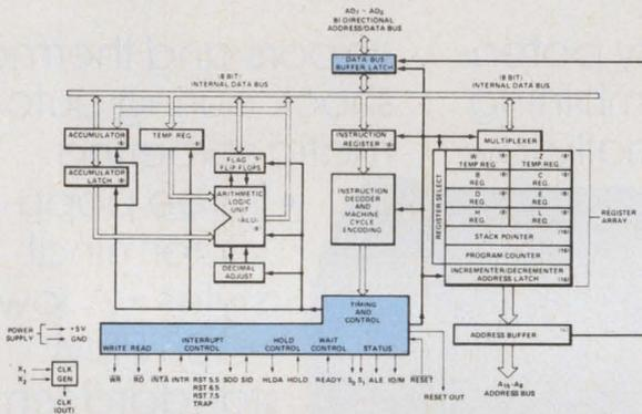
The basic architecture of the 8085 is the same as that of the 8080A. The only differences are the built-in clock generator, the built-in system control circuit and the multiplexed address/data bus structure to make available several pins for additional control.
