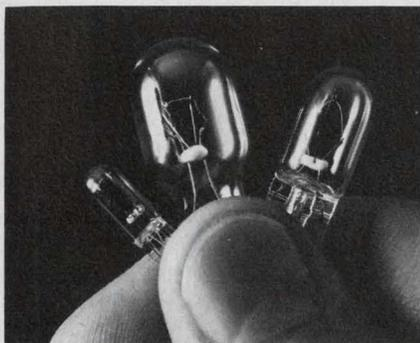
Enjoy new design freedom with this expanded line of GE all-glass wedge base lamps. And keep enjoying the inherent benefits of the line: savings in weight, space, time and costs. GE now offers more than 30 wedge base lamps in three sizes: miniature lamps T-3 $\frac{1}{4}$  (10 mm diam.) and T-5 (15 mm diam.); subminiature lamp T-1 $\frac{3}{4}$  (6 mm diam.). Voltages range from 2.5 V to 28 V. Candlepower from 0.03 to 21 cd.
