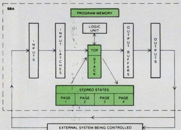
The Sequential Boolean Analyzer consists of a program memory that holds a set of Boolean functions that define system operation as well as 30 input buffers that are latched at the start of the evaluation of Boolean equations, and four pages of 30 stored-state flip-flops which can be grouped to emulate counters and shift registers. Also included are a logic unit that can perform the logic functions and a stack that holds a set of Boolean values used to evaluate the input equation.
