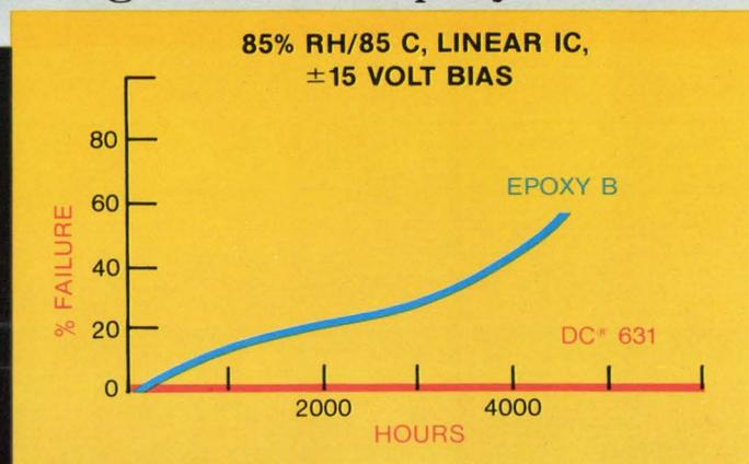
outstanding moisture resistance of silicone. The autoclave resistance of Dow Corning 631 is very nearly as high as that of an all-silicone molding compound. And look what happened on 85°C/85% R.H.-bias testing.
