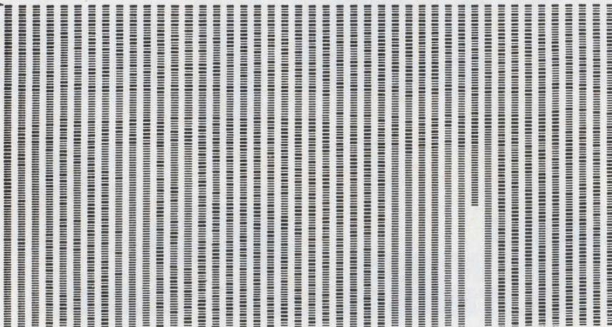
**Computer programs** printed in a bar-code format can be entered directly from a printed page into a computer with the aid of a scanner from Micro-Scan. Sensitivity is so good, that even photocopies of the bar code can be read.
