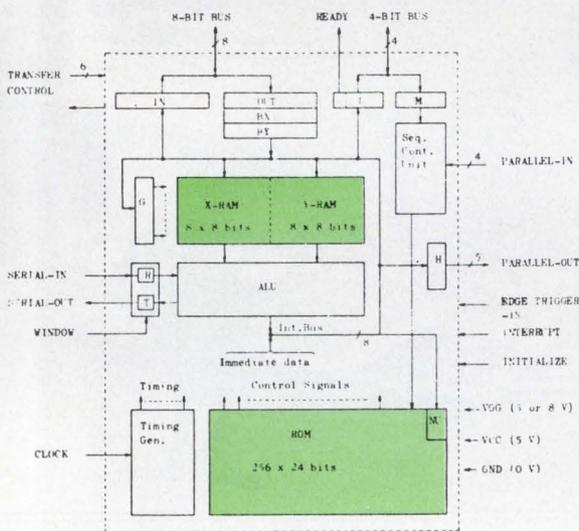
The architecture of the T3444 revolves around two  $8 \times 8$  bit data RAMs that feed in to the ALU. There are 16 lines for dedicated inputs and eight lines dedicated as outputs. The processor also has a separate serial I/O section as well as an on-board clock circuit.
