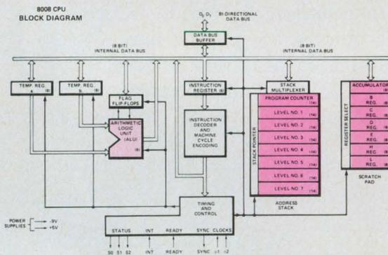
The architecture of the 8008 family parts is similar to the 8080 which has superseded it. On the 8008 chip are a 7-word  $\times$  14-bit stack register, a 6-word  $\times$  8-bit scratchpad register and a parallel 8-bit ALU. An external clock is required along with some RAM or ROM to form a minimal operating system.
