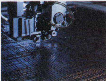
Of the many benefits offered by Multiwire, one of the most important is its simplicity of change and repair. Multiwire boards are normally easier to change after assembly or in the field than multilayer.
