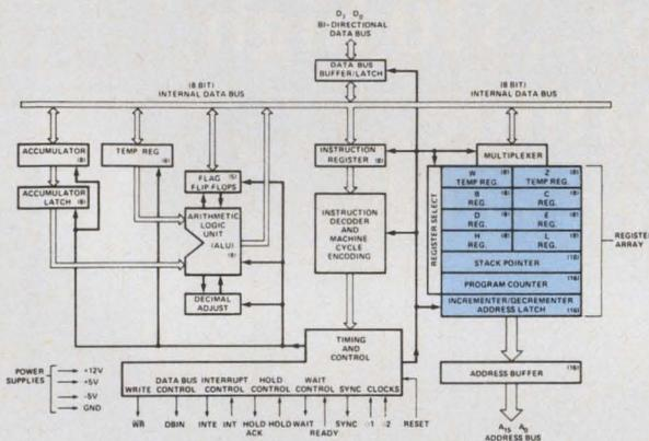
The typical 8080A system consists of a processor, a clock, a bus controller, some memory and a memory decoder. Both the data and address buses are TTL compatible and have three-state capability. All but the clock lines are TTL-compatible.
