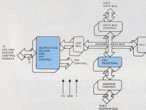
The architecture of the Z80 resembles that of the 8080A, except that there is a second bank of eight 8-bit registers that mirrors the eight registers in the 8080A. All timing generation is on the processor chip except the oscillator, and the Address bus is structured so that refresh addresses appear on the lower half of the bus to refresh dynamic RAMs. A minimal system consists of the processor, a clock source and some memory.
