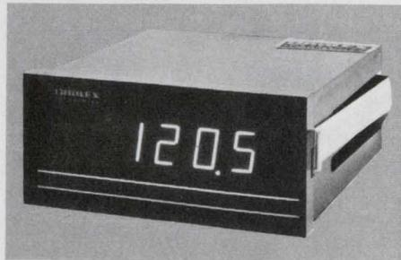
**Digital AC line monitor Model 37DLM** is designed to measure voltages associated with AC power lines or systems. It offers accuracy of  $1/2\%$  and ease of readability at distances to 20 feet. Ranges are 200 or 400 volts with 0.1 volt resolution or 600 volts with 1 volt resolution at frequencies from 45 Hz to 20 kHz. Prices start at \$164 (discounts to OEM). Availability 3-4 weeks. GRALEX INDUSTRIES, 155 Marine Street, Farmingdale, N.Y. 11735 (516) 694-3607
