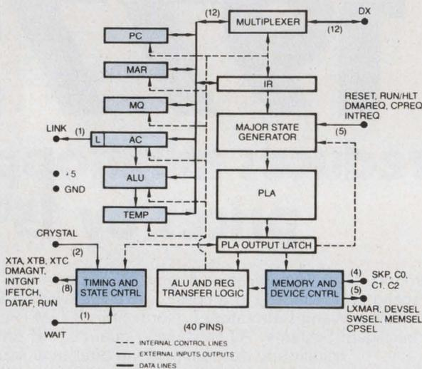
The architecture of the IM 6100 resembles that of the PDP-8 minicomputer. Signals are available that can help create a front panel so that the processor can be manually controlled. The processor's on-board crystal-controlled clock can be driven by an external source.
