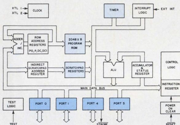
The architecture of the 3870 is identical to that of the original F8, with the extra features of ROM and RAM added to the original chip. Also included on the chip is an 8-bit timer and an 8-bit prescaler. The 3870 can form a complete processor system without any other additional circuits aside from the power supply. All lines are TTL compatible.
