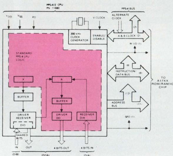
The straightforward architecture of the PPS-4 and 4/2 revolves around the 4-bit accumulator and the three four-bit I/O buses. All lines are designed for direct MOS-level interfaces so to connect to other logic families buffer circuits must be used. The PPS-4 requires an external clock while the 4/2 just needs an external crystal.
