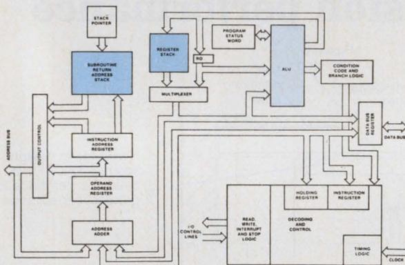
The architecture of the 2650 is centered about the 8-bit ALU and a seven-word register stack. There is also another register stack on the chip to hold subroutine return addresses (it can hold up to eight 15-bit addresses). The 2650 has a single level of interrupt, requires a single-phase external clock and is TTL compatible on all lines.
