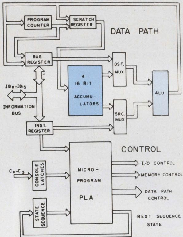
The architecture of the 9440 varies considerably from that of the Nova although the  $\mu$ P can perform the same instructions. The 9440 uses a 4-bit ALU to process data and has an on-board clock generator that just needs an external crystal. Three-state outputs are included on the data/address bus, otherwise all lines are TTL compatible.
