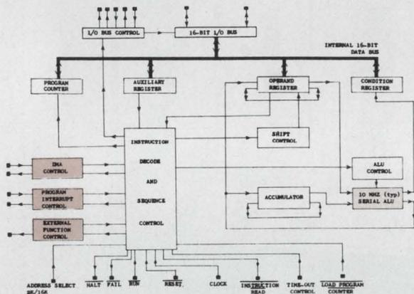
The architecture of the F100-L uses a multiplexed data and address bus. However, to simplify the handling of data many of the bus control functions are handled by support chips. The processor performs all of its ALU operations in a serial mode—the ALU is only 1 bit wide. An external clock is required and a clock rate of up to 20 MHz is possible. All lines are TTL compatible.
