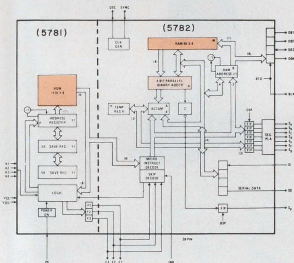
The architectures of the devices in the COPS family of processors are similar. Variations in memory size and I/O capability are the major differences. Most of the processors provide BCD or seven-segment outputs plus all can handle a direct keyboard interface. Only the MM5782 requires an external clock oscillator all other circuits have internal clocks.
