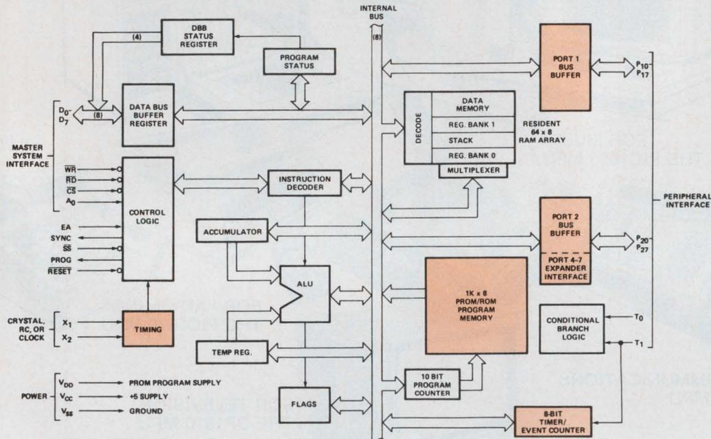
Since the device is a complete microcomputer, it can function as a stand alone unit. Of the 18 I/O lines, 2 are for input only, and 16 are input-output
