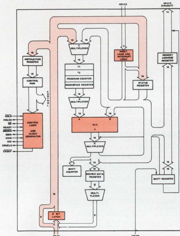
The TMS 9980 is almost identical in architecture to the TMS/SBP 9900. The only difference is that the 9980 uses an 8-bit data bus instead of a 16-bit, a 14-bit address bus instead of a 15 bit and has fewer levels of prioritized interrupt. And, the 9980 has its clock generator built onto the same chip.
