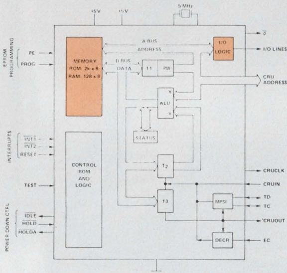
The TMS 9940 is a complete 16-bit computer system on a single chip. On the chip are 2048 bytes of ROM or UV PROM, 128 bytes of RAM, as well as an event counter/timer, a flag register and up to sixteen reconfigurable I/O lines. Even the clock generator is included on the chip. All lines are TTL compatible and the I/O lines are software configurable as either inputs or outputs.
