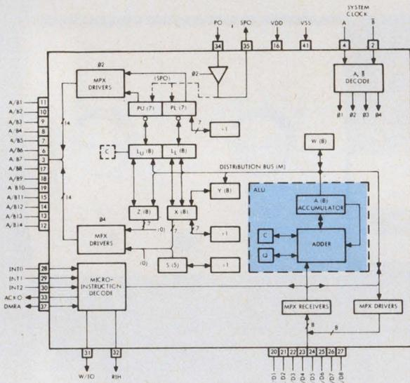
The architecture of the PPS-8 processor is designed to handle both binary and BCD arithmetic. An external two-phase clock must be used, but inside the chip the clock is expanded into four-phase dynamic logic. A minimal system configuration consists of the CPU, a clock and the necessary memory and I/O circuits.
