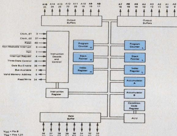
A minimum system for the MC6800 will typically consist of the processor, some ROM and RAM, a clock circuit and some I/O circuits. All lines except the clock lines are TTL compatible and the address bus, data bus and R/W line also have three-state capability. The 6800 has two accumulators, but all stack space is in the user-supplied RAM—there are no auxiliary registers on the processor chip.
