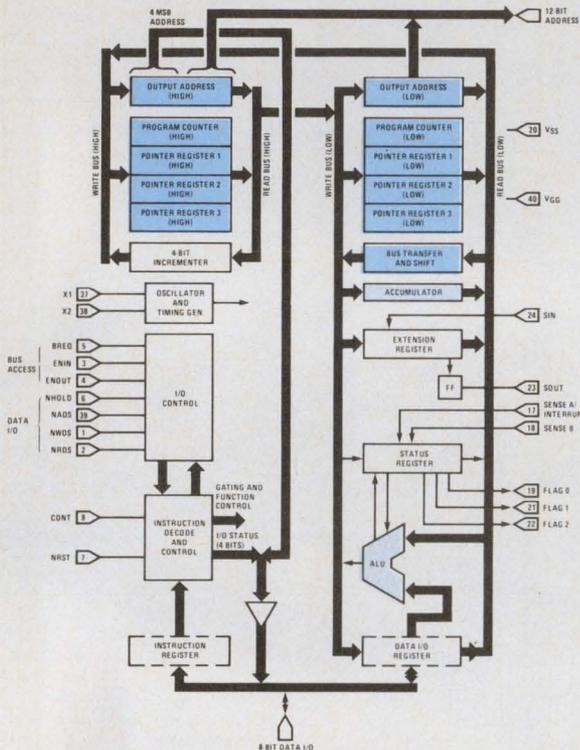
The architecture of the SC/MP provides the processor with DMA capability as well as a simple cascadable structure that is handy for multiprocessing applications. On the chip is the clock circuit to simplify the timing requirements.
