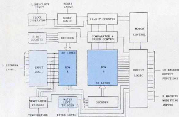
The architecture of the 7150 uses two ROMs to control the various output functions. There is no ALU since no data manipulation is required. However, there are two analog inputs to the processor that are used with an on-chip difference amplifier to form a temperature sensing circuit.
