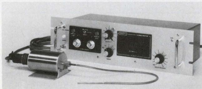
Fiber-optic probes permit infrared signal transmissions over distances that allow Vanzetti IR temperature-monitoring electronics to be removed from high-temperature environments without affecting the accuracy of the measurements.
