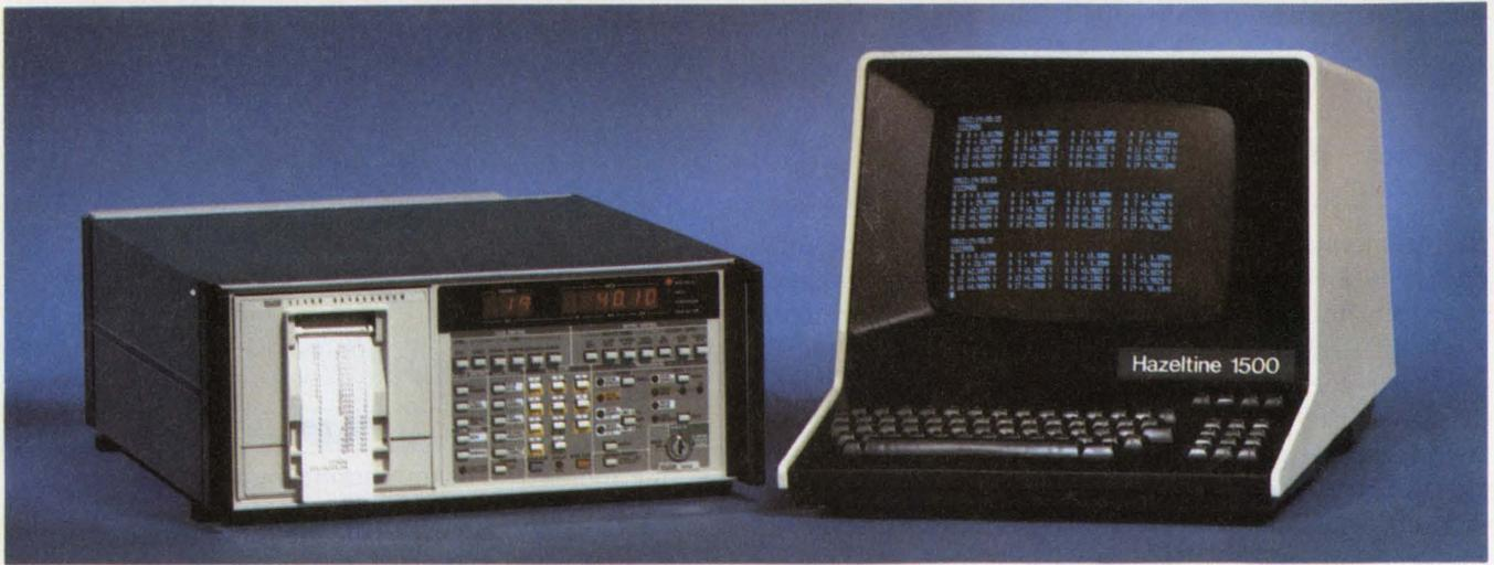
Sixty thermocouples, thermistors, or RTDs can be scanned by the Fluke 2240B microprocessor-controlled Data Logger without special equipment. With it, as many
