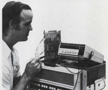
Many companies are streamlining field service of microprocessor-based products by troubleshooting to the component level with the 5004A signature analyzer.
