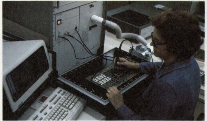
**A software simulator generates programs capable of testing 360 points** on a UUT approximately 10,000 times a second on the DTS-70 from HP. Boards containing 220 MSIs can be tested with programs that an experienced person can prepare in about two weeks.
