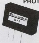
The SLP protectors were expressly designed to protect signal/data/telephone lines from transient overvoltages caused by lightning, heavy machinery, elevator motors, generators, etc. The SLP interfaces between the signal lines and the sensitive circuit to provide a sophisticated blend of high speed (nanoseconds) voltage limiting and brute force protection. The SLP's recover automatically to standby when the need for protection has passed.
