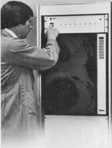
**W**ith Dylon's new GPIB (IEEE-488) tape recorders, you can now transfer data directly from the Bus to 1/2" magnetic tape. With NO interfacing. Just plug it in.
