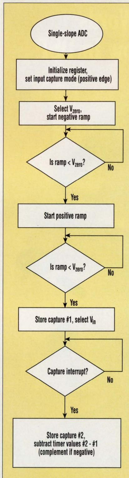
**3. THE INPUT capture method uses logic that's similar to the polling method. But for a given resolution, it generates less jitter. Input-capture measurements also have quicker conversions because overcounting and averaging aren't used.**
