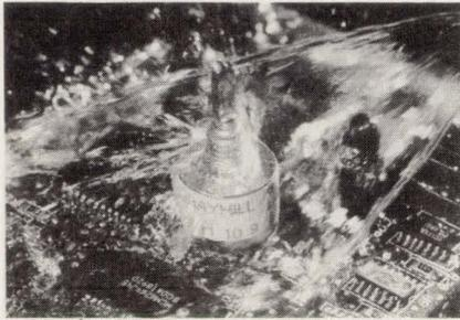
A 1.2-in.-diameter rotary switch is capable of withstanding wave soldering and board-cleaning techniques. The slight premium for the Series 50/51T switch is more than offset by the savings in assembly costs. Solder-lug terminals and water-tight panel seals are optional. Pricing is \$7.50 in lots of 100 for a 1-deck, 1-pole switch. Delivery is in four weeks.
