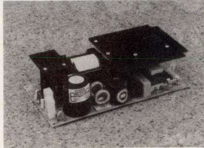
dc. An onboard input-line filter exceeds the requirements of VDE/FCC Class B by an average margin of 10 dB. Pricing is \$159 in quantities to 24. Call for delivery.
