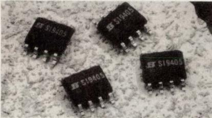
require the extra drive circuitry typical of n-channel high-side switches and has an extremely low on-resistance (0.12  $\Omega$ ) even when operating from logic signals. The low on-resistance means more power is available to the load. Pricing is \$0.95 in large OEM quantities. Samples are available now with production quantities in eight to 12 weeks.
