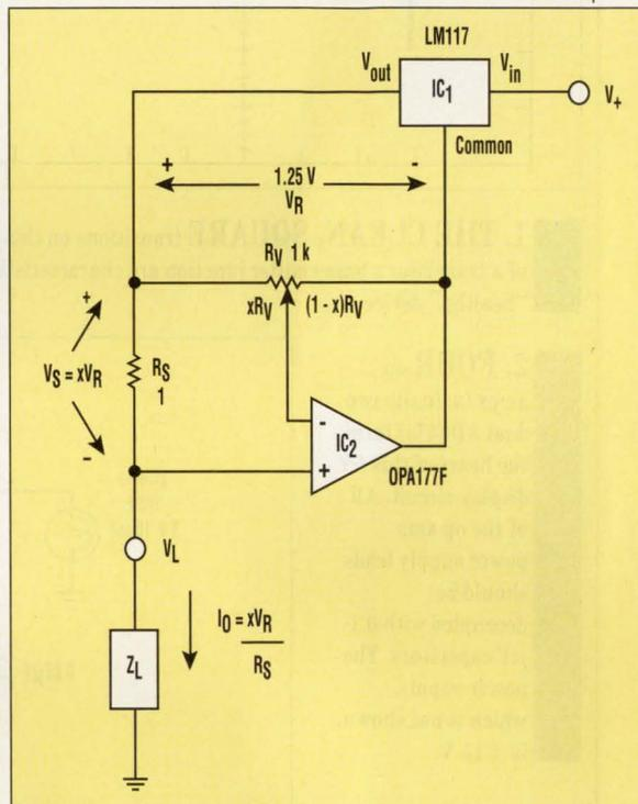
**LINEAR CURRENT CONTROL** results from bootstrap feedback, which redefines the control characteristic. This circuit has a current range of 0 to 1.25 A, an output resistance of 8 kΩ, and a maximum drift of 0.025% per °C.
