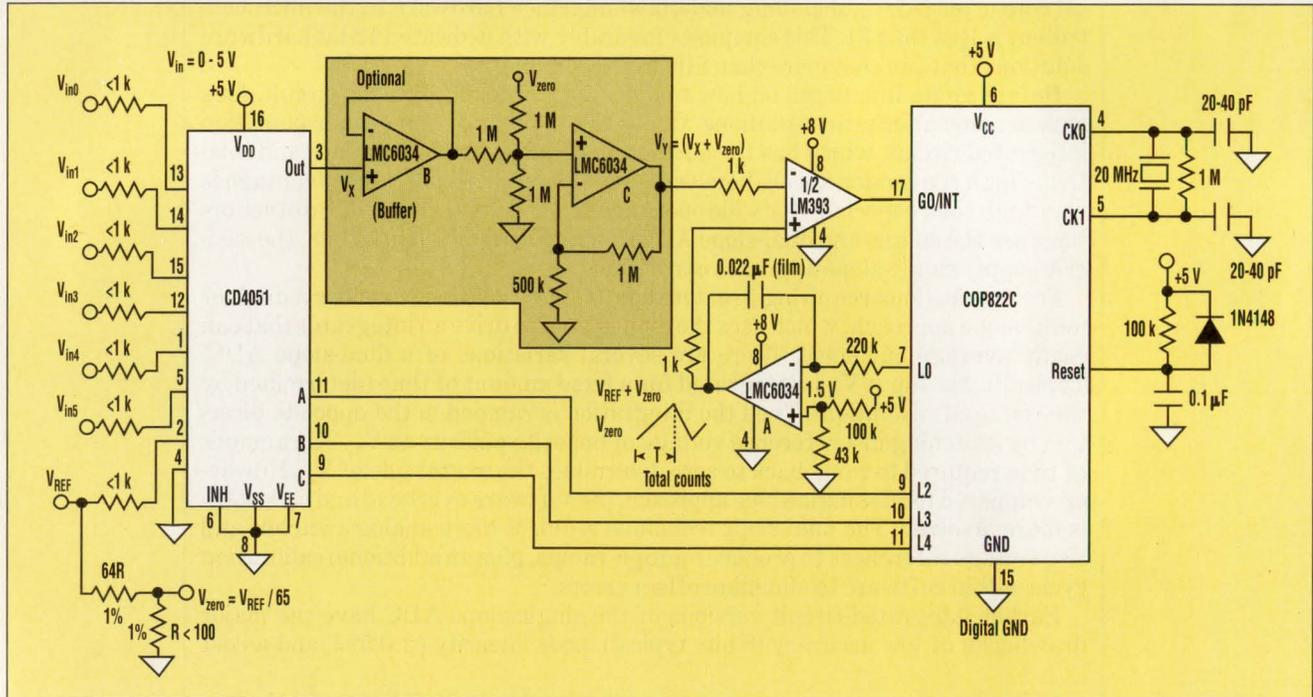
**1. A MULTICHANNEL ADC** with 12-bit accuracy can be designed with an 8-bit microcontroller, a voltage comparator, a multiplexer, and an op amp. The LMC6034 op amp configured as a voltage-integrating ramp generator, A, is the heart of the ADC. Optional buffer op-amp B may be required to offset errors caused by the multiplexer input resistors. Op-amp C isn't mandatory for limited measurement ranges.
