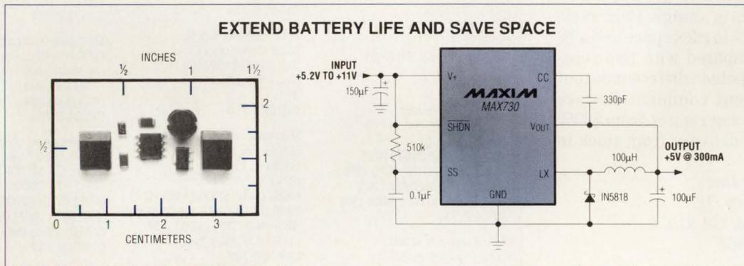
The MAX730 application circuit fits into 1.125in<sup>2</sup> (7.25cm<sup>2</sup>) of board space.
