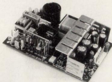
board assembly with a 1.25-in. profile. The triple-output supply has no minimum load requirements. Suggested retail price is \$55. Small quantities are delivered from stock.
