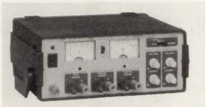
supplies in one. Included within the unit are two variable 24-V, 0.5-A supplies and a fixed 5-V, 4-A unit. The two 24-V supplies are switch-selectable for series operation, which doubles the output to 48 V; parallel operation, which delivers up to 1 A of output; or independent operation. Suggested pricing is \$395 and delivery is from stock.
