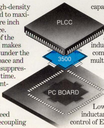
capacitors around the perimeter of the IC package. This "stacking" technique also helps to lower inductance and impedance compared to conventional multi-layer capacitors.
