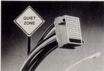
The Quiet Zone SC modular coaxial cable assemblies offer the highest signal fidelity available in 0.025-in. square post packages. Over 90%  $V_p$  signal speeds and 0.5% crosstalk at sub-nanosecond rise times is featured. A patented 360° shielding technique completely shields the signal line, both within the cable and through the connector. This keeps insertion loss to around 2 dB at 1 GHz for 10-ft lengths. Call for pricing.
