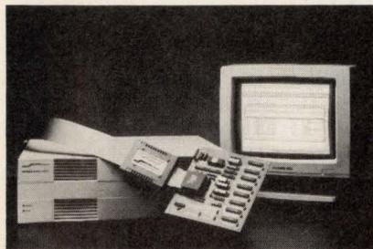
debugger. The Express III includes features to selectively store execution cycles from cached operation, identify conditions that are in and out of cached execution range for transition to other trigger levels, and measure system performance with the cache on. The Step Express III is priced from \$35,000 and is available 30 days after receipt of an order.
