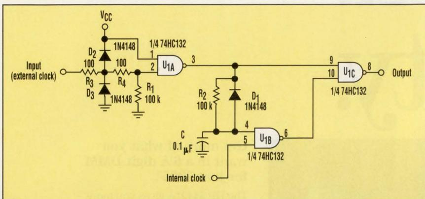
**AUTOMATIC CLOCK DETECTION** is provided by  $U_{1A}$  in combination with  $R_1$ . Resistors  $R_3$  and  $R_4$  and diodes  $D_2$  and  $D_3$  protect the input of  $U_{1A}$ .
