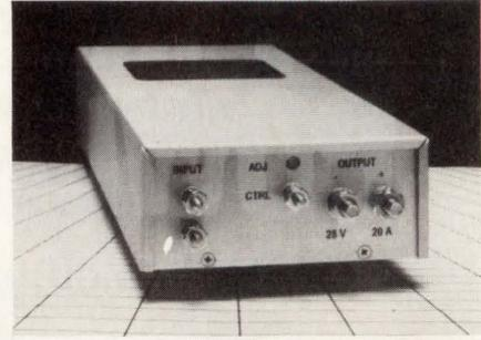
A line of ruggedized ac-dc conditioned power sources is well suited for use with distributed-power dc-dc converters and systems. The PB Series is available with single- or three-phase ac input and dc outputs from 24 to 300 V, including 28, 48, 155, and 270 V. True N+1 current sharing as well as 0.99 power-factor correction is featured. Call for pricing and delivery.
