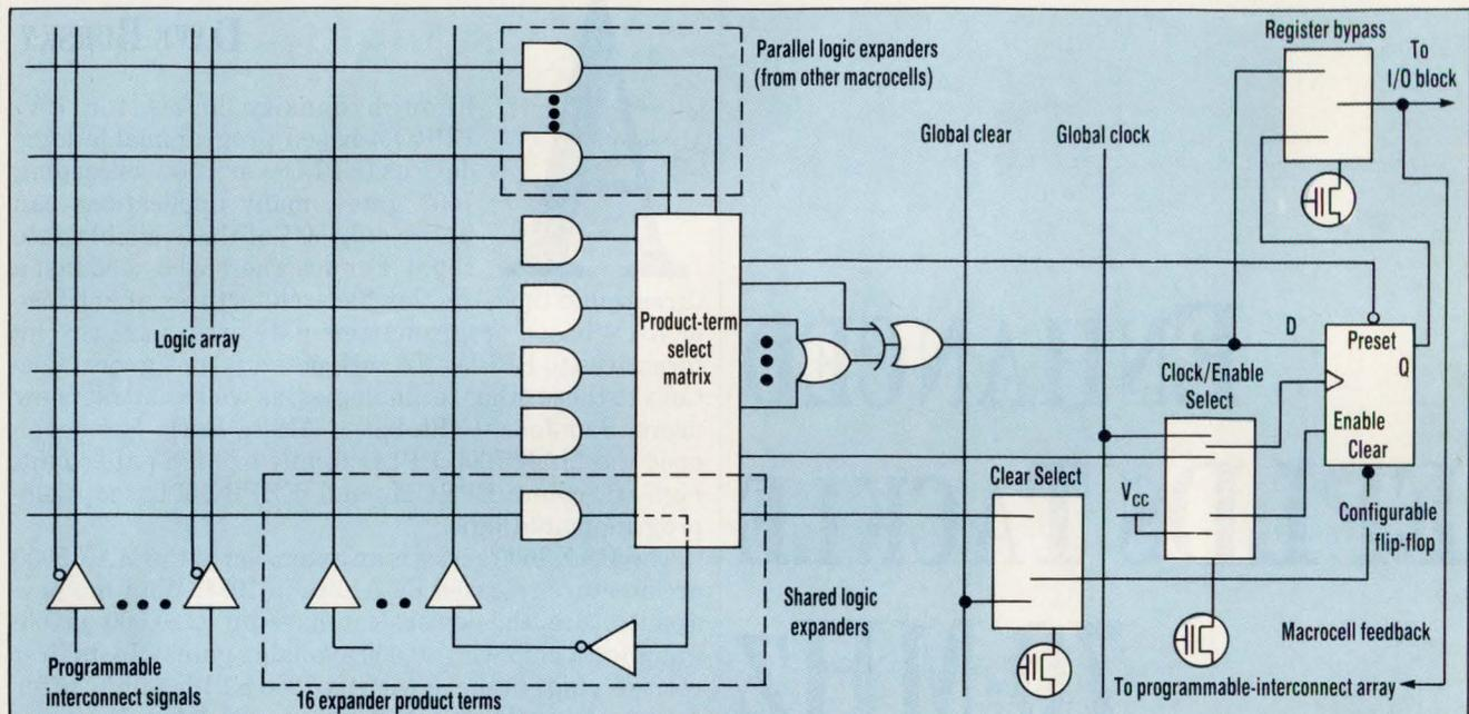
**THE ENHANCED MACROCELL** in Altera's EPM 7000 series of EPLDs includes a new parallel-logic expander block that locally expands the number of product terms available to the macrocell, while adding just 2 ns to the signal delay. The macrocell can also use 16 shared expander-product terms. They add about 6 ns to the signal delay, but can be distributed across all logic blocks on the chip.
