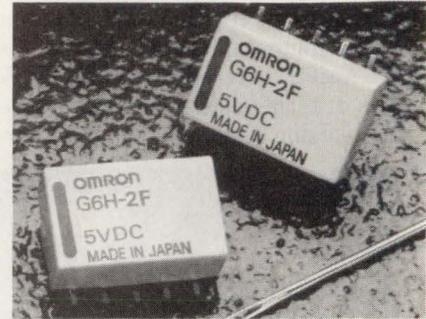
With 140 mW of nominal power consumption, the G6H-2F submini surface-mounted relay needs less power to energize than earlier models. The 2 Form C unit comes in coil voltages of 3, 5, 6, 9, 12, and 24 V dc and can switch up to 1 A. It also conforms to FCC Part 68 surge-withstand requirements of 1.5 kV. List price is \$2.45 in lots of 1000.
