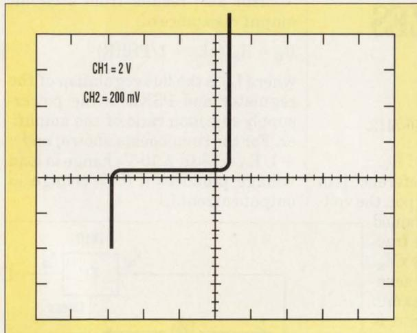
**1. THE CLEAN, SQUARE** transitions on this display of a transistor's base-emitter junction are characteristic of a "healthy" device. □
