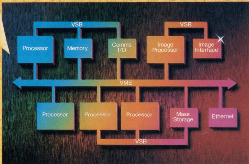
***A multiple systems-within-a-system architecture forming tightly coupled sub-systems capable of independent and parallel operation.***
