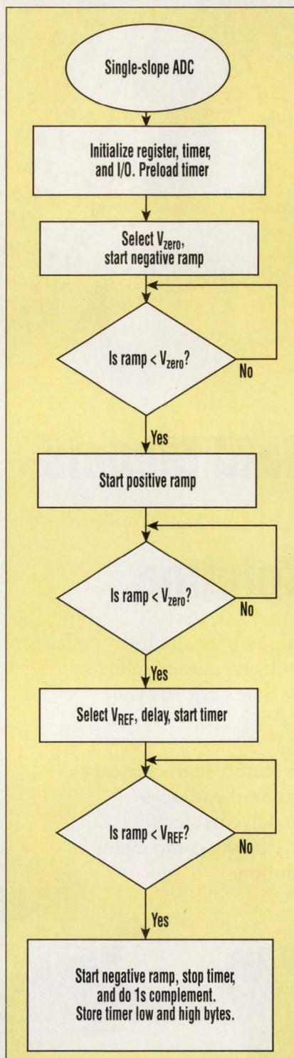
**2. CODE FOR** the polling method in single-slope analog-to-digital conversion starts with initializing the I/O to control the integrator and multiplexer. For maximum accuracy, the length of the polling loop during the measurement of  $V_{in}$  should be as short as possible.
