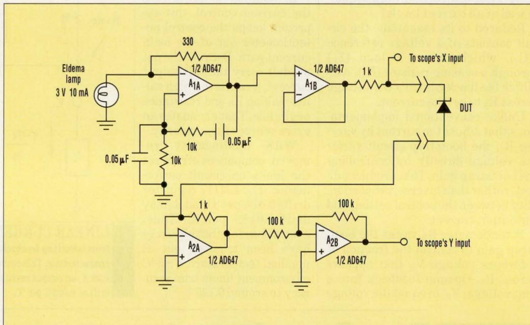
nents, this circuit can be used to isolate faulty components in circuit boards. The idea is to compare the scope display across various points of the unit under test with the display for the corresponding points on a board that's known to be good. With a bit of practice, it should be possible to recognize at least some common faults on sight.
