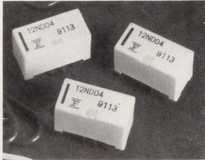
long, the unit offers a 43% size reduction in pc-board area compared with earlier telecom relays. Coil power has also been reduced to 140 mW compared with the typical range of 200 to 500 mW. Maximum switching voltage for the 12-pin DIP unit is 150 V dc and 125 V ac. Maximum current is 1 A. List price is \$6. Volume production is scheduled for the first quarter.
