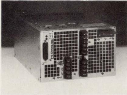
Total harmonic distortion of less than 5% is featured in the model HC1010 1000-W switching supply. The unit also offers 0.99 power-factor correction as standard and meets the proposed IEC 555-2 specification. Other features include current-mode control, absolute current sharing, and shut-down current limiting. Call for pricing and delivery.
