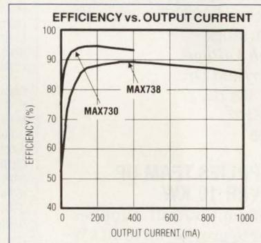
The MAX730 and MAX738 deliver high efficiency over a wide load range.
