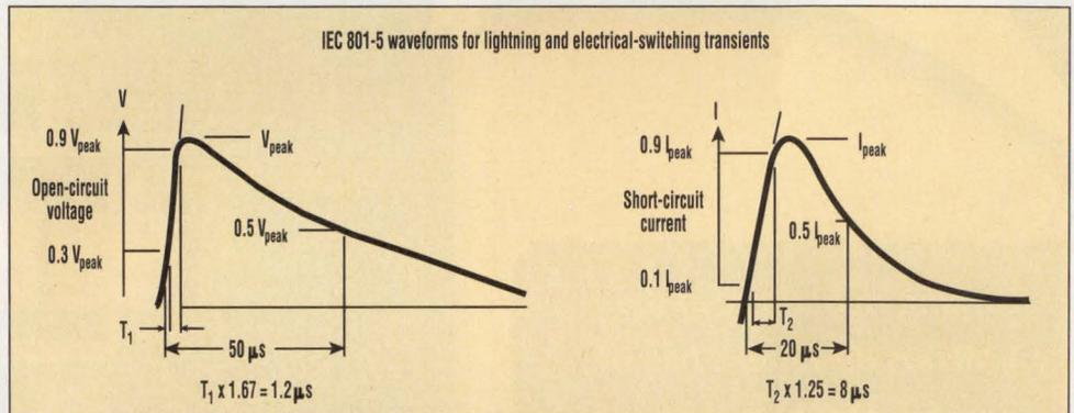
1. As defined by IEC 801-5, the short-circuit current waveform is for power-line applications. The current waveform for signal-line applications approaches that of the voltage waveform.
