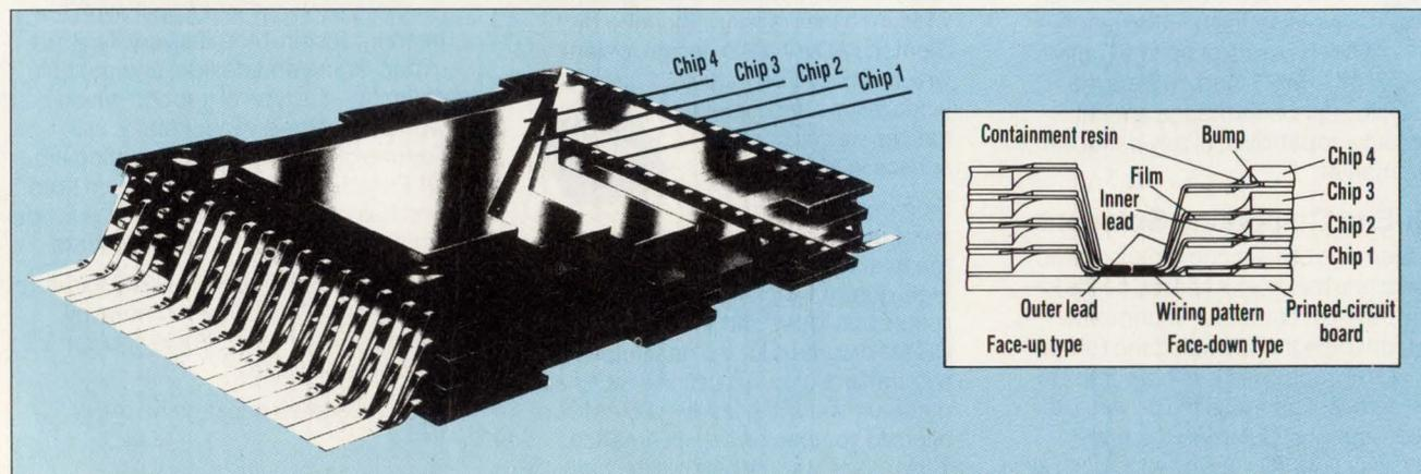
**3. BY STACKING CHIPS** one on top of the other and in a rightside-up, upside-down configuration (called multilayered bonding), Panasonic can achieve a mounting density four times greater than conventional packaging methods.
