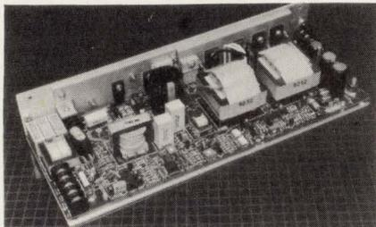
handles 10 A/16 A peaks for spin-up loads associated with hard-disk drives. Pricing in lots of 100 is \$339. Small quantities are delivered from stock to three weeks with 12-week leads for large lots.
