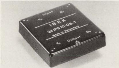
±5, 12, or 15 V dc. Packaged in a 2-by-2-by-0.41-in. metal case, the converter delivers 80% efficiency with 500-V rms input-to-output isolation.
