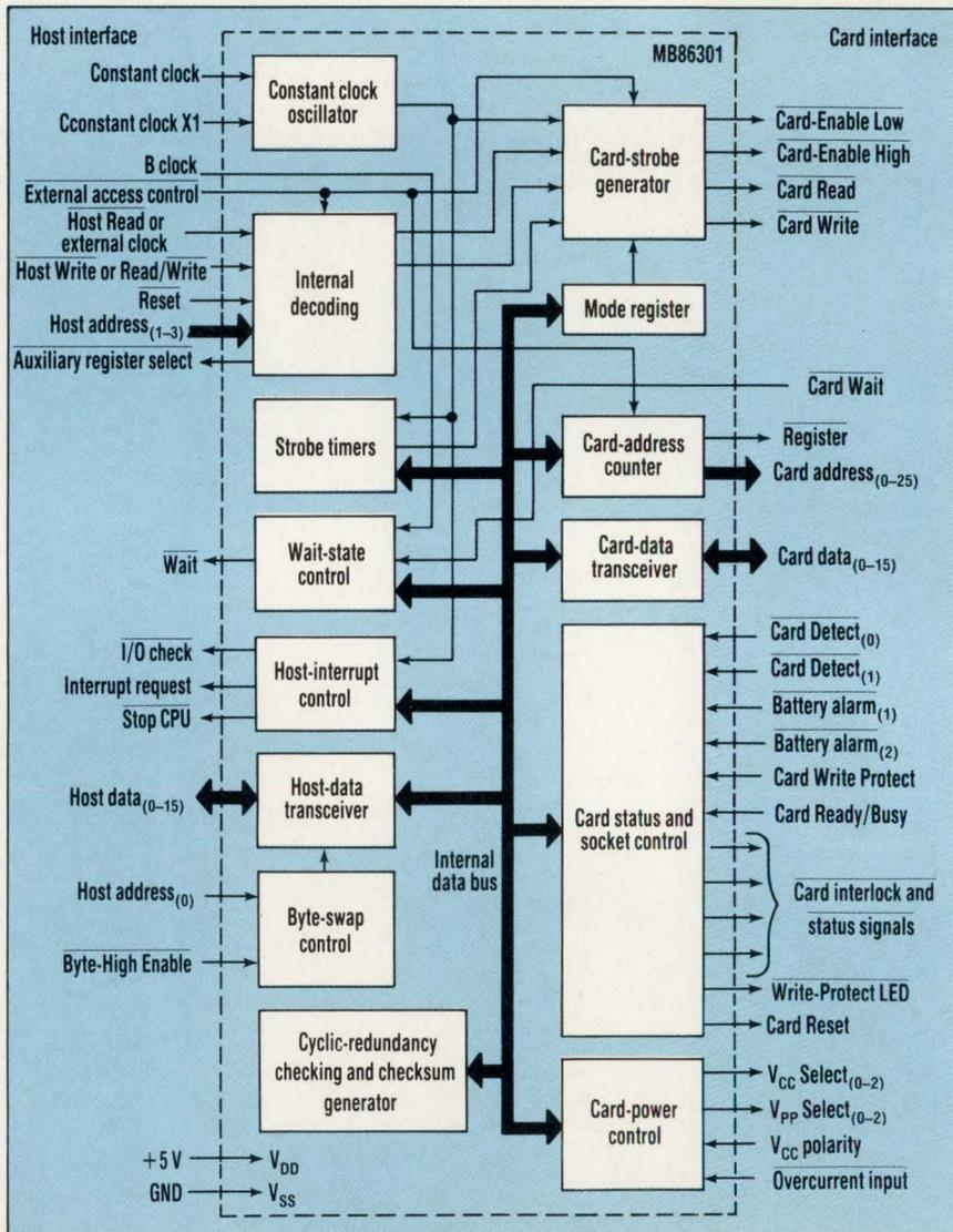
**2. THE MB86301 MEMORY-CARD CONTROLLER** from Fujitsu sits between the 68-pin connector of the PCMCIA memory card and the host microprocessor. The internal card-address counter ensures rapid data transfer.
