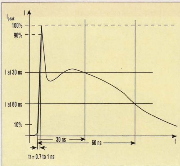
duce intense localized radiation that may not be present with contact discharge. Therefore, in a practical sense, the contact method may fail to adequately test for certain aspects of radiation immunity.
