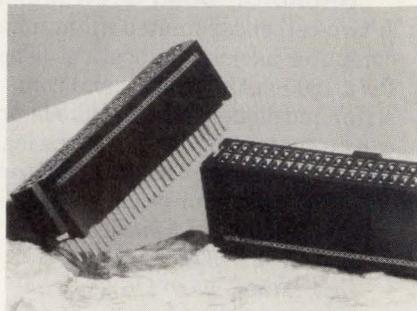
A micro IDC system for mating with terminal strips on 0.050-by-0.100-in. centers is available. Socket (female) strips in the FCSD Series feature a dual-beam, tuning-fork-style BeCu contact. Terminal (male) strips in the FCMD Series also feature BeCu contacts. Both male and female strips come in from five to 40 positions per row. Each three-prong contact makes two gas-tight links with each wire. Pricing starts at \$0.06 per contact. Delivery is in two weeks.
