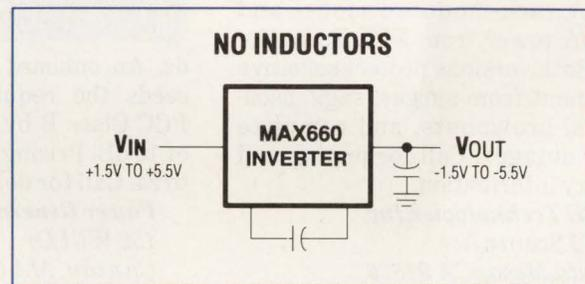
The MAX660 uses only 2 external components and is available in space-saving 8-pin DIP and SO packages.
