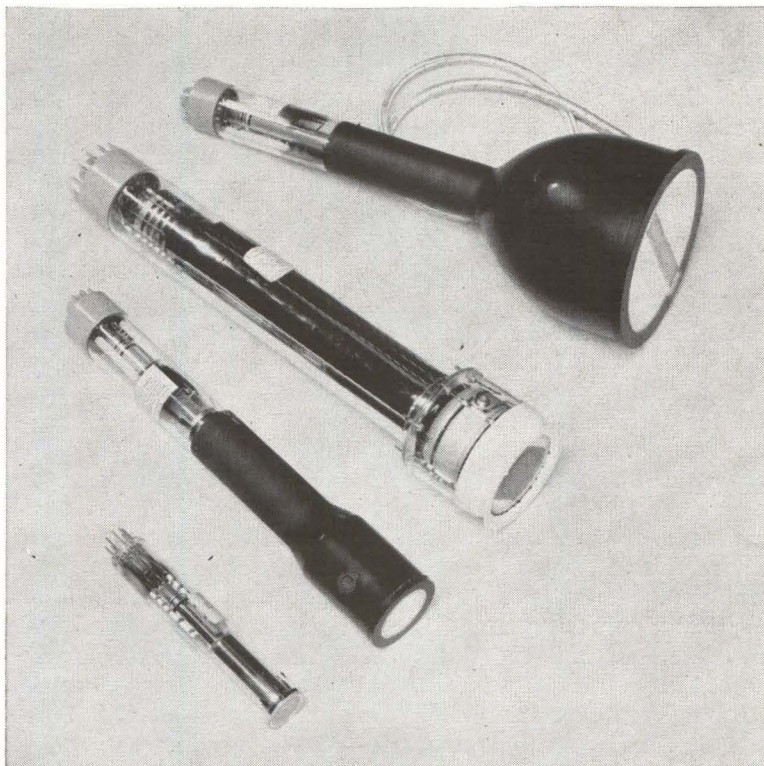
FIG. 6—Video tubes using fiber-optic faceplates, from top to bottom, cathode-ray tube, two image orthicons and a vidicon, all by RCA
