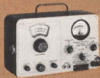
Solid State Model 127 A-Y Special feature: Solid state with rechargeable battery pack. Carrier rack fast patch for use with Western Electric Type O and N carrier Frequency range: 2 KC to 350 KC Selectivity: 250 cps Frequency accuracy: \pm 1 KC Measuring accuracy: \pm 1 db Size: 7\frac{1}{2} " x 7\frac{1}{2} " x 12\frac{1}{2} ", 16 lbs., including batteries Price: $945.00 with battery pack. Rechargeable batteries and charger optional at extra cost
