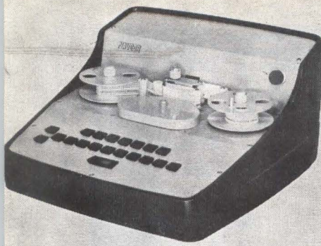
VISUAL PRINTOUT , magnetic key-board, remote programming ability feature Navigation Computer's tape-puncher for numerical machine control
