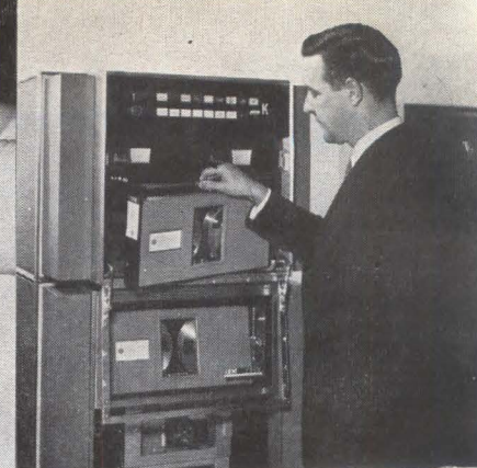
CARTRIDGE-LOADING tape-drive system introduced by IBM has an instantaneous data rate of 170,000 8-bit characters a second
