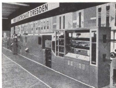
WESTERN OBSERVERS were surprised by the quality of this East German line for automatically producing resistors. Three people run it
