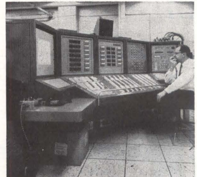
GROUND STATION console provides digital gimbal angle and 366 analog status readouts to Walter Muench, OAO test director, shown giving instructions to spacecraft controllers during a test
