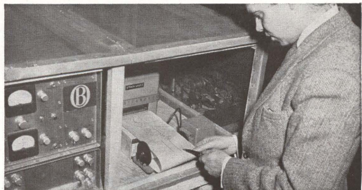
The Honeywell Model 906 Visicorder Oscillograph—with a Honeywell Model 119 Amplifier—record circuit bushing tests for Ohio Brass.
