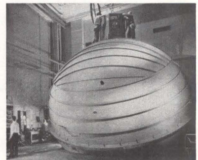
BUTTONED-UP CHAMBER. Men at top adjust solar simulator, while those at left control simulated space phenomena
