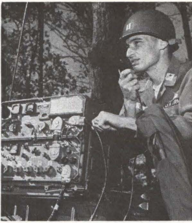
ARMY'S AN/GRG-106 mobile ssb radio (p 7, Feb. 1) will have a range of at least 50 miles, can use any one of 28,000 1-Kc channels. Contractor is General Dynamics
