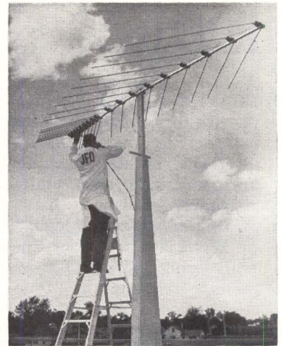
TEST MODEL of all-channel log-periodic antenna
