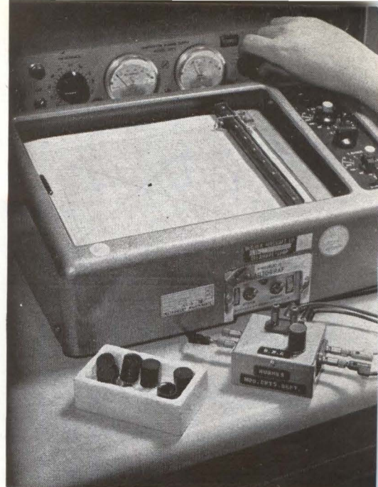
FAMILY of negative resistance elements are checked on a plotter to determine characteristic curves
