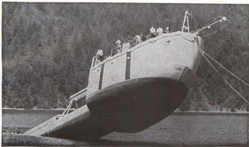
FLIPPING into vertical position is Flip (Floating Instrument Platform), an important tool for making accurate measurements of sound transmission in the ocean and for other tests important for ASW work. Total Navy spending for oceanography in 1964 will be $106.9 million. Other government agencies will spend an additional $82.5 million
