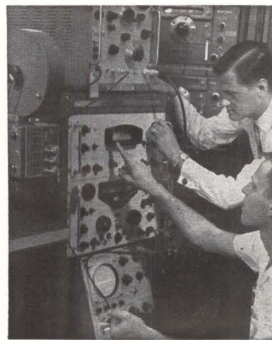
TEEPEE radar can detect missiles at 5,000 mile ranges, seconds after launch, by h-f ionospheric backscatter. Cro shows different patterns for missile firings and explosions
