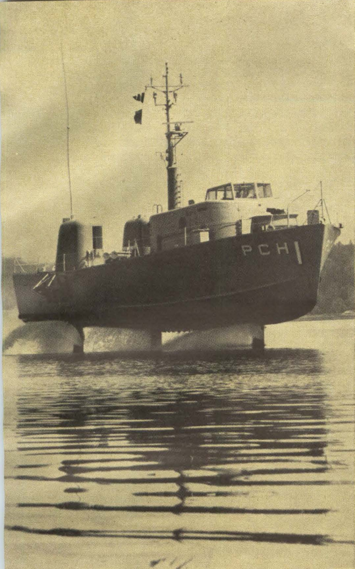
ANTISUBMARINE DUTIES may evolve for a class of hydrofoil boats designed to "fly" above the surface at speeds over 100 knots. Boeing developed this craft, which uses electronic stabilization of submerged foils
