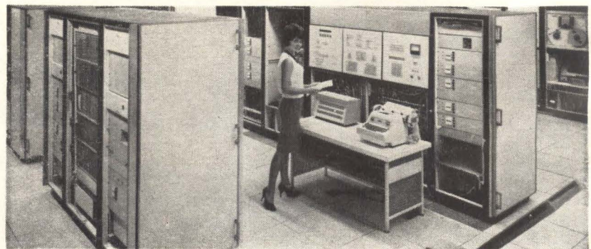
THIS IS FIRST PHOTO released for publication of data-processing system that Librascope is building for Air Force's 473L command and control system. System includes mass-memory disk file (left), central computer (center) and magnetic tape consoles (left and right). This system is to be used in the Pentagon
