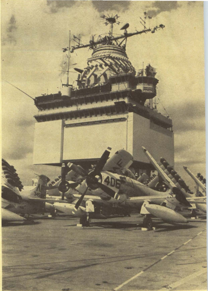
NAVY'S NUCLEAR powered aircraft carrier, Enterprise . Electronic scan radar including rows of diagonal bars, encircle a portion of the island. Other radar, communications, and navigation gear bristles from the control center
