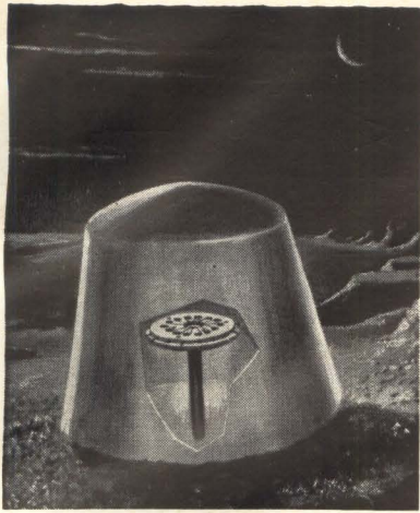
MULTIVATOR would try to get an enzyme reaction in dust samples, thus producing detectable fluorescence
