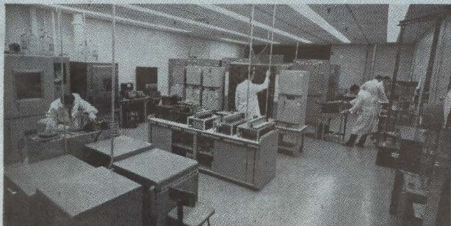
The TRIMPOT Division Environmental Laboratory is capable of performing tests to MIL-R-27208, MIL-R-22097 and MIL-R-12934.
