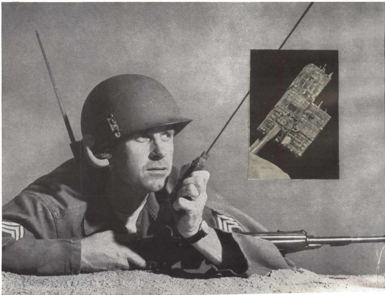
ARMY TESTS field radio, one of a series developed by RCA. Transmitter-receiver uses micromodule packaging technique, similar to sample displayed in inset
