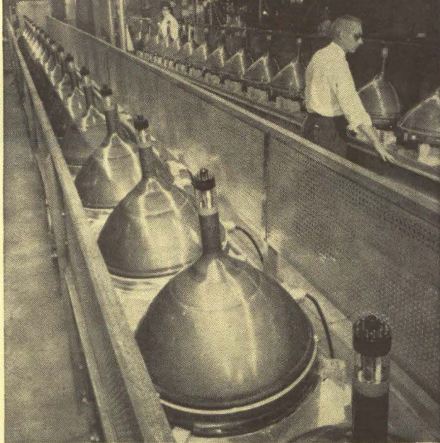
COLOR PICTURE TUBES move along conveyor at RCA plant. Glare-proof windows are bonded to face in this operation
