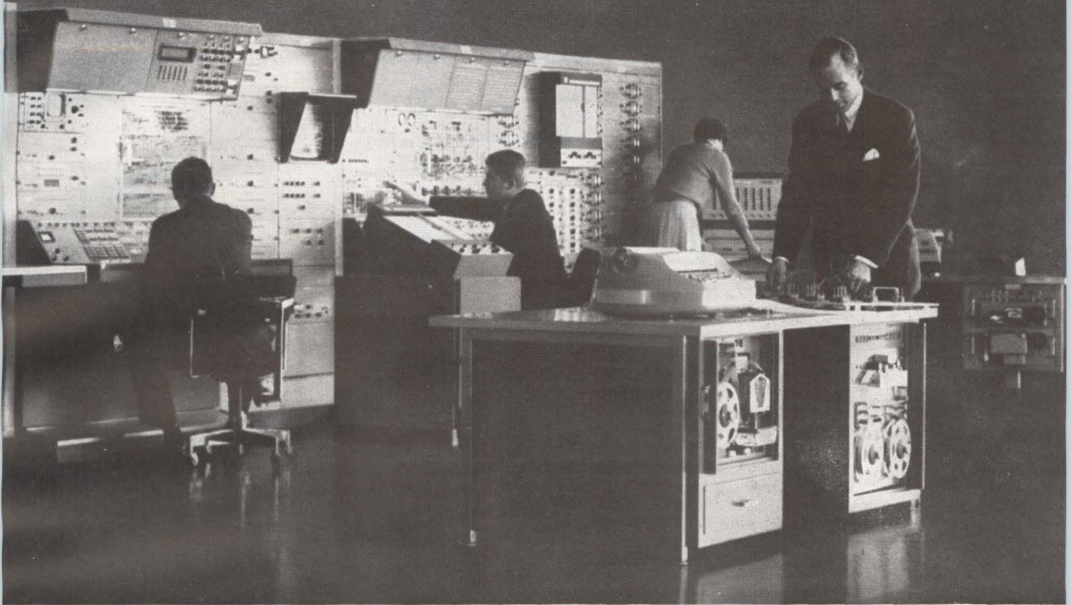
HYBRID COMPUTER developed by Electronic Associates, Inc., performs both analog and digital operations. Inclusion of digital aids in analog computers is emerging trend in large-scale simulation systems
