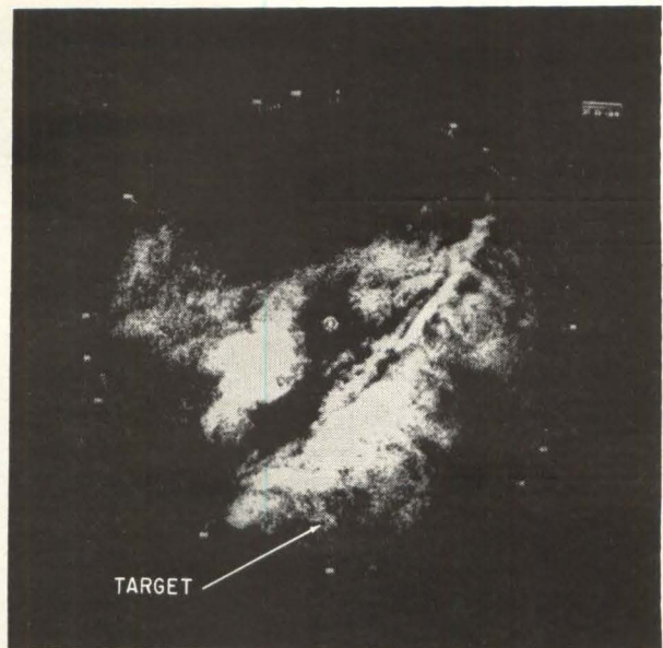
Typical PPI presentation of a radar video signal in heavy clutter. Target at 180° is lost in the weather return.
