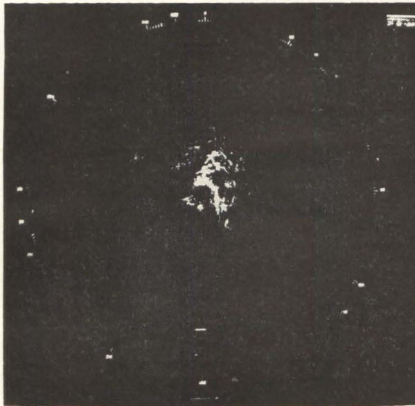
Typical PPI presentation of a radar video signal in heavy clutter. Target at 180° is lost in the weather return.
