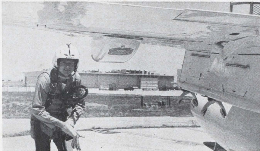
Tucked under the wing of a fighter plane is Bendix Corp's highly accurate radar altimeter. The instrument is being installed on many Navy fighter planes.
