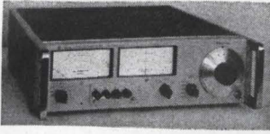
Direct reading of magnitude and phase is provided by two large meters on Vector Impedance Meter.
