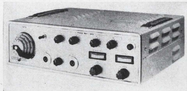
All controls, including the bolometer connecting points, are on the front panel of the model 1500. It requires only two additional instruments to measure insertion loss.
