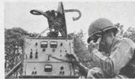
Portable MP-7 microwave unit for tactical use.
