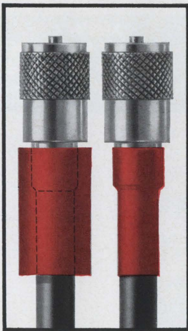
New ITT Heat Shrink Tubing easily fits over coax connector, yet, because it shrinks to 50% of its original size with the application of heat, the tubing forms a tight insulating bond around both the coax and the connector.
