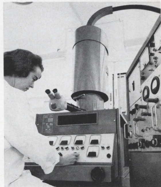
Electron-beam welder used by Autonetics for experimental production. The welds are made in the vacuum chamber, left.
