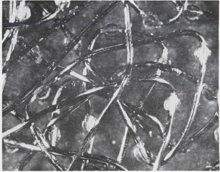
A very compact form of point-to-point wiring is welded magnet wire. The joints in the Sylvania wiring plane (left) correspond to flatpack lead positions. The posts in the Jet Propulsion Laboratory matrix (right) are 50 mils apart.
