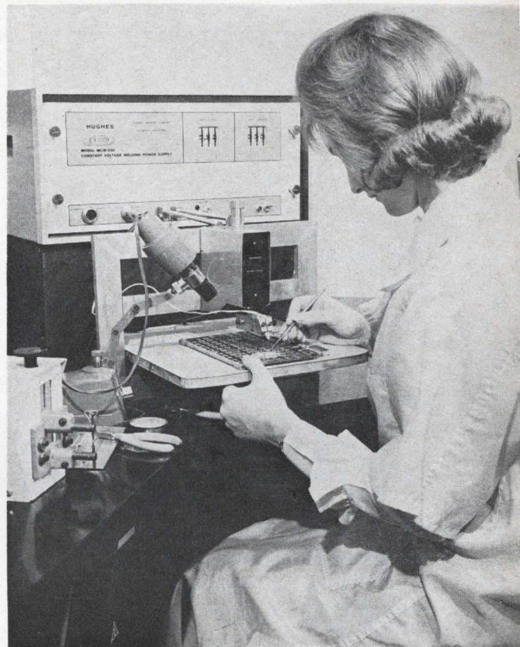
Parallel-gap soldering machine is similar in operation to the parallel-gap welder shown on the facing page. The electrodes of both are placed atop the flatpack leads. However, the joints are made by reflow of solder rather than by fusion of flatpack lead and printed-circuit metals.
