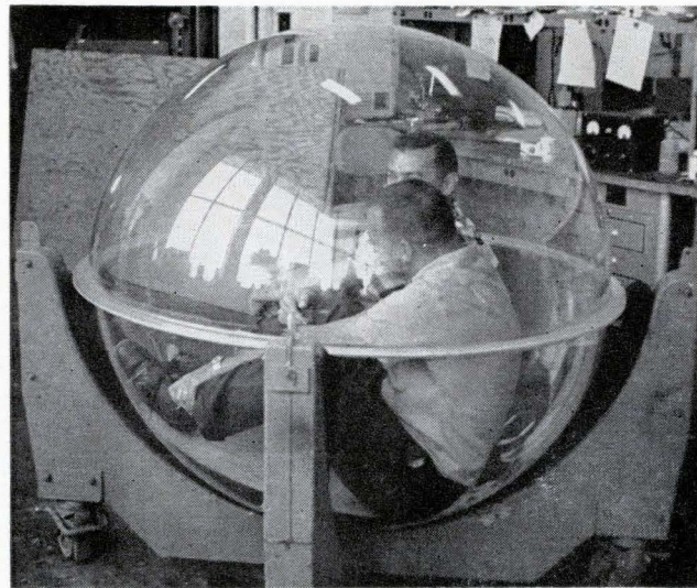
Model of glass bubble that will descend to the bottom of the sea. Unique light-modulating technique will be used to communicate between the deep-sea bubble and a separate electronics package.
