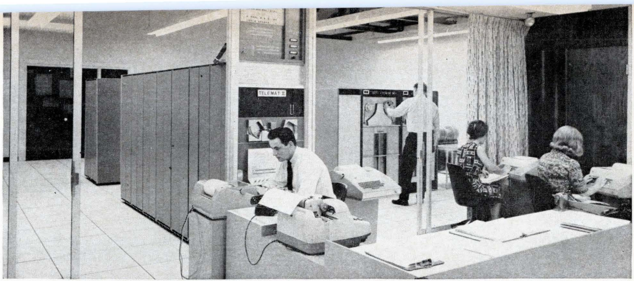
Massachusetts General Hospital's computer system for medical record-keeping and research. The computer, installed at Bolt Beranek & Newman Inc.'s laboratory in Cambridge, is about seven miles from the hospital. The computer can be seen immediately behind the operator's panel to the right of the man at the teleprinter. Behind the computer are the memory banks; in the extreme rear is one corner of the drum storage unit; tape drives are visible at the right.
