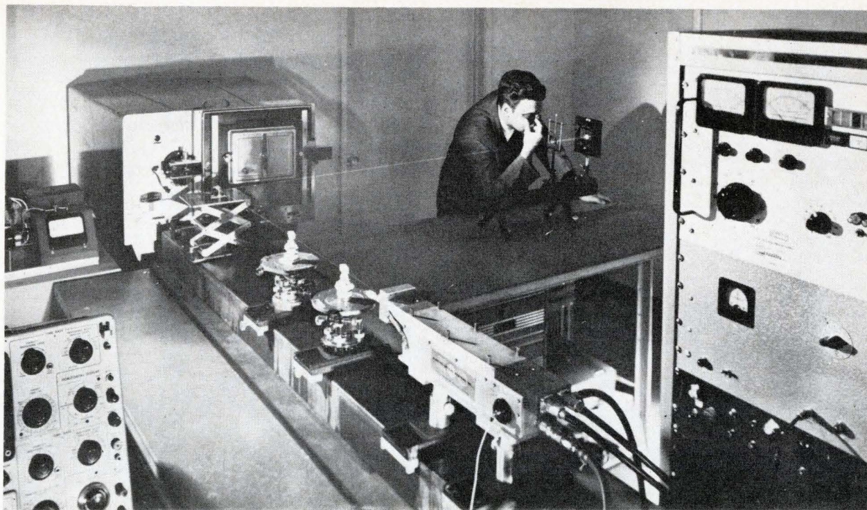
Q-switched neodymium laser and associated nonlinear crystals, used for frequency doubling. Ten megawatts of green laser light are generated by doubling the 1.06-micron output with a KDP crystal.
