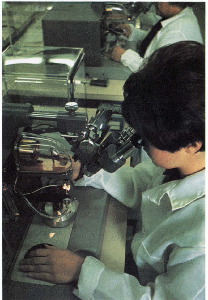
Operator steers integrated circuit chip in x-y plane using controls on either side of work station preparing for die bonding.
