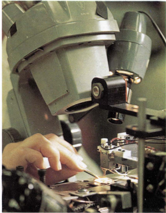
Fine gold wires are bonded to integrated circuit under microscope by assemblers at Westinghouse.
