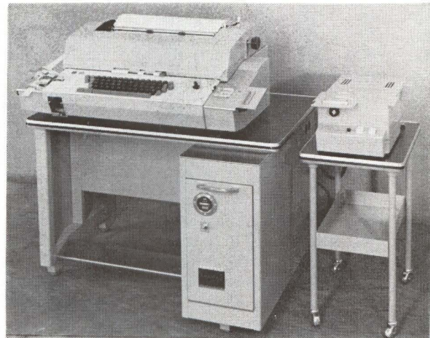
Parallel data transmission unit reads standard eight-hole paper tape and transmits the data in parallel over eight telephone lines. Two more telephone lines transmit control signals between the transmitter and receiver. This unit is a prototype.
