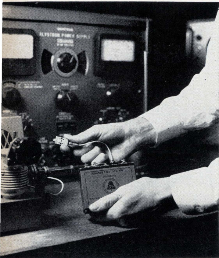
Size advantage of the LSA oscillator is evident in this comparison of it with an air-cooled, low-power klystron and its power supply.
