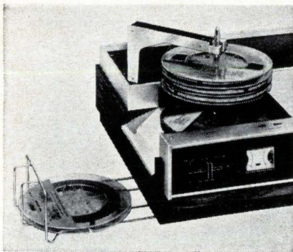
Reeling on. Sony tape deck plays stack of five tape reels automatically.
