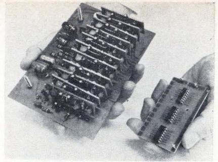
**Simplicity in IC's.** Subsystem (right) built with MOS IC's, which are packaged in plastic, takes only one-tenth the space of an equivalent unit (left) built with discrete devices.
