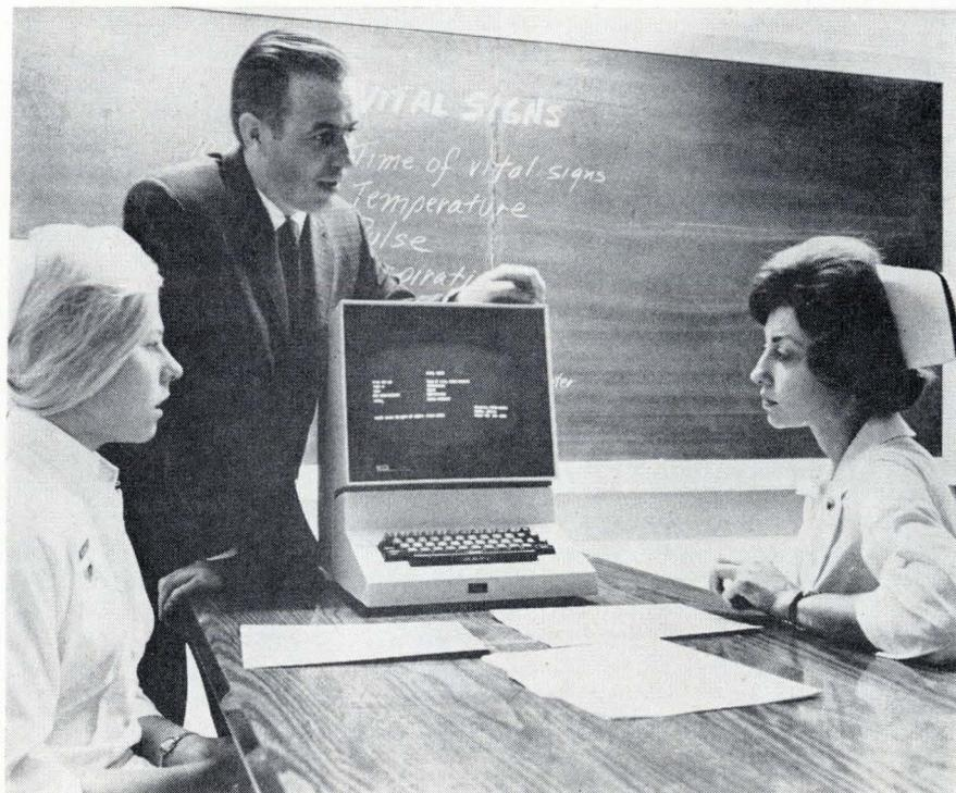
The medical knowledge stored in the computer will be available to hospital doctors through a keyboard-and-cathode-ray-tube arrangement or typewriter readout. After a patient's symptoms have been matched to this stored data, the system will display its diagnosis, any special tests required, and recommend treatment for the physician's consideration.
