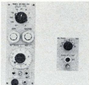
Model 8806B is a phase-sensitive demodulator. It is a solid state plug-in preamp for acquiring accurate amplitude and phase information. It has a carrier frequency range of 50 hz to 40 khz, gain stability of better than 0.25%/10° from 0° to 40° C, and response 3 db down at 1/5th of reference frequency. Hewlett-Packard Co., 175 Wyman St., Waltham, Mass. [386]
