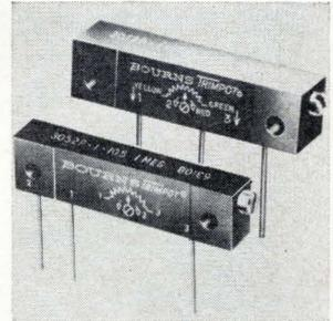
Standard resistance range of the models 3012 and 3052 Palirium cermet adjustment pots have been expanded from 10 ohms to 1 megohm. Operating temperature range is  $-65^{\circ}$  to  $+175^{\circ}$  C; contact resistance variation, 2.5%; and power rating, 1 w at 70° C. The Palirium cermet provides infinite resolution. Bourns Inc., 1200 Columbia Ave., Riverside, Calif. 92507. [356]
