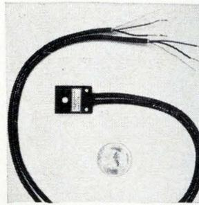
Hall-effect transducers measure steady-state, pulse, or transient currents without connection to the conductor under test. The CT-7W offers a rise time less than 1  $\mu$ sec, dynamic range of less than 1 ma to 30 amps peak, and frequency response flat to over 1 Mhz. It measures  $1\frac{3}{4} \times \frac{3}{8}$  in. with a  $\frac{3}{16}$ -in.-diameter opening. Ohio Semitronics Inc., 1205 Chesapeake Ave., Columbus, Ohio. [363]
