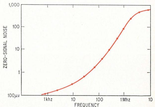
**Shifting center frequency.** As  $f_o$  increases, the zero-signal noise increases rapidly.
