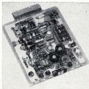
Video amplifier VA1367 is a d-c coupled, 10 Mhz, solid state plug-in unit featuring a gamma-corrected transfer function to produce a linear relationship between crt light output and input-video drive. It employs feedback and temperature compensation to provide optimum gain stability and temperature independence. Beta Instrument Corp., 377 Elliot St., Newton Upper Falls, Mass. [383]
