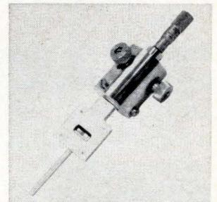
Model 410-A09 automatic frequency control and monitor cavity has a stability of  $\pm 1$  Mhz from  $-30^\circ$  to  $75^\circ$  C. It can be used to stabilize klystrons in discriminator circuits. The cavity offers a tuning resolution of  $\pm 0.5$  Mhz from 5.9 to 7.4 Ghz. A locking device protects the frequency setting against accidental change. Microlab/FXR, 10 Microlab Rd., Livingston, N.J. [416]
