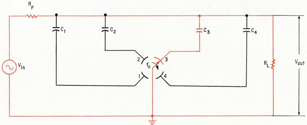
A simple shunt-switched digital filter is formed by connecting several capacitors in parallel to segments of a rotary switch. The circuit is returned to ground through a series resistor,  $R_F$ , and the switch. Output is the voltage developed across the grounded capacitor,  $C_n$ . Color indicates grounded capacitors in all diagrams.
