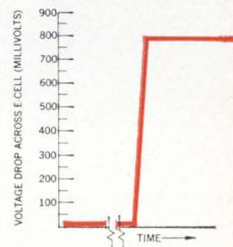
\* The Bissett-Berman E-CELL™ is a unique "liquid state" electrochemical timing and integrating component now being manufactured in high volume on fully automatic production lines. E-CELLs are designed for single use or re-cycling, can be set or re-set in the field, and are furnished in wire-lead or plug-in versions. A multiple-electrode E-CELL enables complex functions such as two-phase timing — or subtotaling and totaling — with
