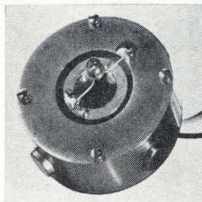
A solid state pulser provides up to 250 amps for driving laser diodes at room temperature. It uses avalanche-transistor techniques to produce 70-nsec pulses with 7- to 10-nsec rise times. Pulse repetition is adjustable from 300 hz to 10 khz. Volume of a 150-amp unit with a 10-khz driving oscillator is 1 cu. in. Austron Inc., 10214 N. Interregional Highway, Austin, Texas. [394]
