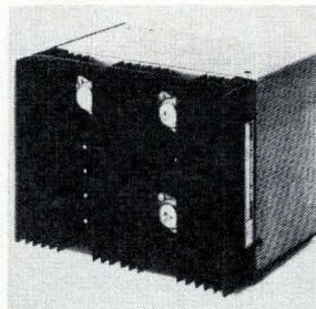
High-voltage d-c power supply modules include units to 410 v. Voltage regulation of 0.01% is provided in the BX series and 0.5% in the BC series. Both have plug-in p-c board construction, automatic overload and short-circuit protection, remote sensing, and remote voltage adjustment or programing. ACDC Electronics, 2979 N. Ontario St., Burbank, Calif. [387]
