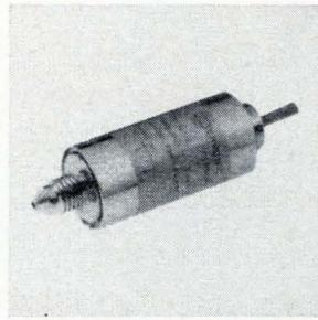
Potentiometric transducer 2101 operates in the ranges of 0 to 350 through 0 to 20,000 psi. It has an over-all accuracy of  $\pm 1\%$  at vibrations of 50 g. Normally used for control and telemetry, the unit will measure and monitor air, fuel, lubricants, and hydraulic fluids. It weighs 2 oz. and measures 0.75 x 1.5 in. Servonic Instruments Inc., 1644 Whittier Ave., Costa Mesa, Calif. [366]
