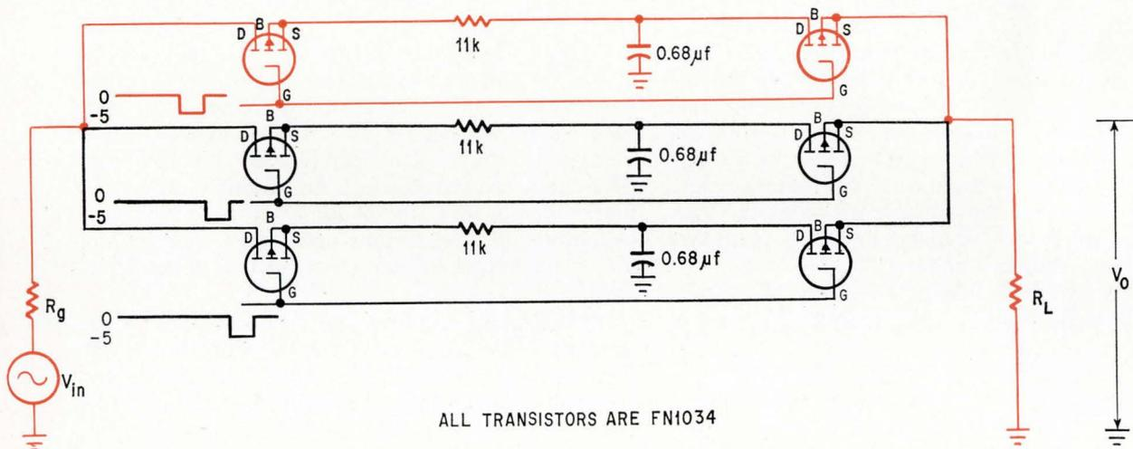
**Two field effect transistors** replace the pair of rotary switches used in the mechanical arrangement. Switching is controlled by a chain of delayed pulses applied to the coupled gates and the output is taken across the grounded capacitor.
