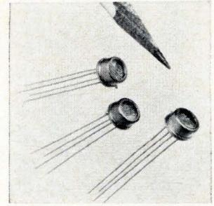
Each unit of the type 4610 photo-cells has 2 independent, isolated photoconductors. Use of 1 enclosure assures equal illumination for the 2 elements. Both elements are processed at the same time on a single substrate to yield equal response characteristics. Lighted resistance changes less than 1.5 from  $25^\circ$  to  $65^\circ$  C. Hewlett-Packard Co., 1501 Page Mill Rd., Palo Alto, Calif. [344]
