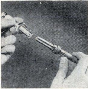
Precision connectors assure rated voltage standoff in mated or unmated condition. Recessed center contacts and precontact grounding are for safe handling. Maximum leakage across the interface is less than  $1 \mu\text{A}$  at 20 kv d-c and sea level pressures. The rated voltage is for limited pulse use. Reynolds Industries Inc., 2105 Colorado Ave., Santa Monica, Calif. [341]
