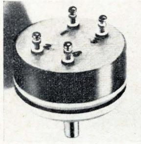
Custom-engineered pots made of conductive plastic, have 0.5% absolute linearity in the centers of their operational range, tapering to 0.15% in their end regions. Model 14C-1 offers a resistance of 100 to 20,000 ohms  $\pm 10\%$ ; power capability, 1.3 w at  $25^\circ$  C; torque, 0.2 oz maximum; minimum life, 5 million cycles. Gamewell division, E. W. Bliss Co., 1238 Chestnut St., Newton, Mass. [346]
