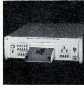
Analog measurements are made of digital IC's automatically by instrument 133. It can do up to 10,000 parameter measurements in 1,000 steps in  $\frac{1}{100}$  sec. Up to 15 readings can be made at a 10- $\mu$ sec logical step. Programming is by two 5 x 6 in. circuit cards; one covering all devices in a family, the other the type to be tested. Teradyne Inc., 183 Essex St., Boston. [367]
