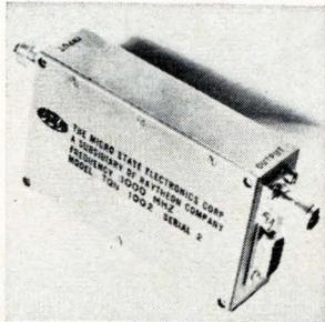
An L-band transistor amplifier is stable in an airborne rocket environment under all conditions of vswr and phase at the input and output. It has a gain of 17 db, 3-db bandwidth of 40 Mhz, and dynamic range of 60 db. With a center frequency of 1 Ghz, it includes a 10-db image reject filter at 1,120 Mhz. Micro State Electronics Corp., 152 Floral Ave., Murray Hill, N.J. [409]
