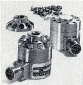
Suited for the chemical and aerospace fields where high pressures are to be monitored, series 250 transducers are available in 6 ranges from 0 to 5,000 to 0 to 20,000 psig. Housing and pressure cavity are of stainless steel and electrical components are sealed from the pressure media by stainless steel diaphragms. Taber Instruments, 455 Bryant St., North Tonawanda, N.Y. [361]
