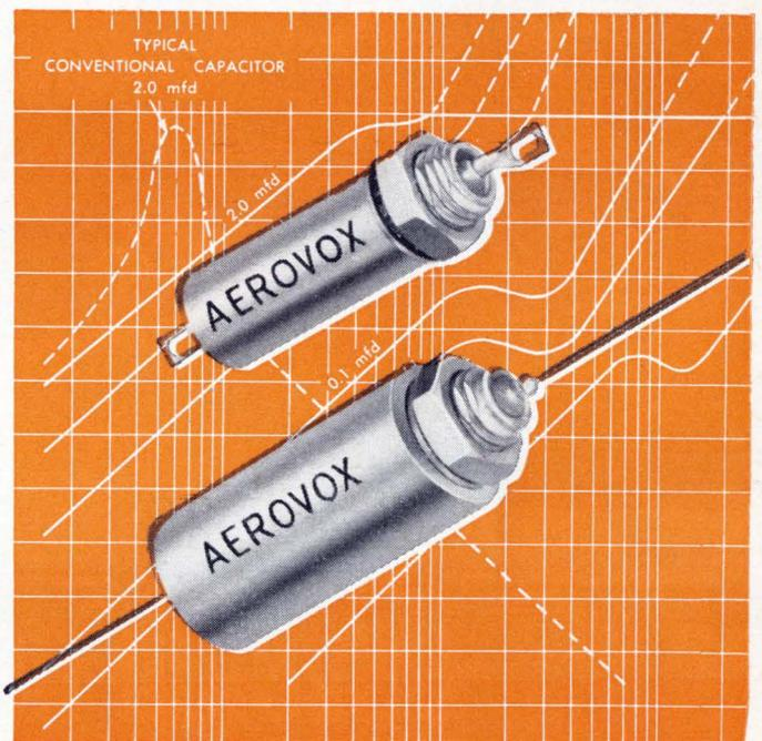
Present military specifications require that electronic equipment be kept free of interference from 150 KHz to 10 GHz. Aerovox type FC low pass, miniature ceramic RFI suppression filters will meet or exceed the applicable requirements of MIL-F-15733. These new units have been life tested for 250 hours at  $1\frac{1}{2}$  times the working voltage. After test, insulation resistance of units is greater than 50 megohms.
