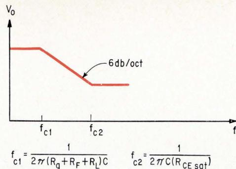
**Limiting the attenuation.** By including the transistor's saturation resistance into the equivalent circuit of the digital filter, the designer obtains an additional break point in the filter's response curve. Thus, he is able to limit the maximum attenuation.
