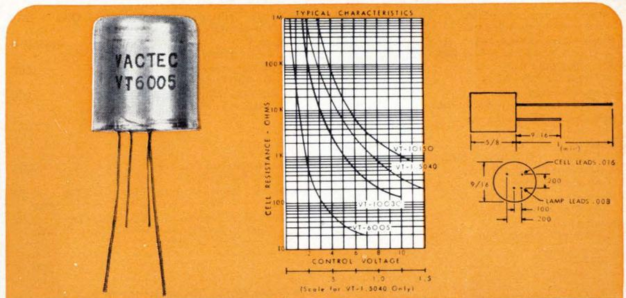
Now 1.5v, 6v, and two 10-volt Vactrols are available for electronic amplifier applications. Combines a dependable Vactec photocell with the proper long-life incandescent lamp in a complete low-cost module.
