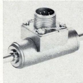
An electromagnetic switch provides a sharply rising electrical output voltage at a specified core position. It may be used to energize an indicator light at the switching point directly, to actuate a relay, or to trigger an electronic switch. Input is 26 v, 400 hz; output 6 v, 400 hz. Kavlico Electronics Inc., 20869 Plummer St., Chatsworth, Calif. 91311. [355]
