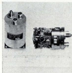
Model 15-400 aircraft transducer is a quick-reacting sensor that determines rate of altitude change and provides a linear d-c output voltage proportional to the rate of climb or dive at rates up to 6,000 ft/minute over an altitude range from sea level to 70,000 ft. Accuracy is  $\pm 5\%$  to 50,000 ft and  $\pm 10\%$  to 70,000 ft. Ed-cliff Instruments, 1711 Mountain Blvd., Monrovia, Calif. [375]
