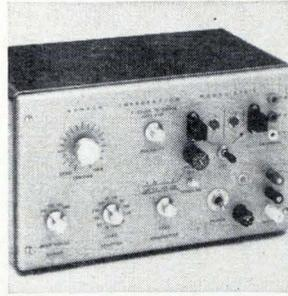
Transistor curve tracer CTA-2 displays a family of curves for both bipolar and field effect devices when used with any general purpose d-c scope. Base current steps of 20, 100, and 200  $\mu$ a are provided with 4 ranges of sweep voltage to 240 v. Voltage steps for FET testing are continuously adjustable. Price is \$435. Rameco Corp., Box 580, Deerfield Beach, Fla. [362]
