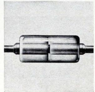
Whiskerless, voltage-variable capacitance diodes cover 3 to 18 pf. The Q's exceed 500 at 50 Mhz. Inductance is less than 0.5 nh; package capacitance, 0.2 pf. The diffused planar silicon units offer leakage under 100 na at 20-v reverse voltage. Double-plug construction gives reliability; the DO-35 package, high density. MSI Electronics Inc., 34-32 57th St., Woodside, N.Y. [443]
