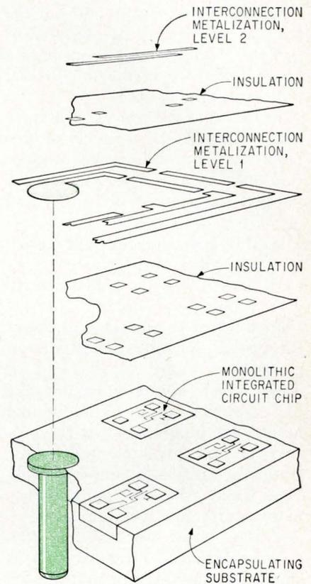
the Singer Co., says the process, called coplanar integration, casts chips in the ceramic substrate so that their faces are up and on the same level as the substrate surface. Friden inverts the package by placing the interconnecting grid of microscopic wires and two insulating silicon dioxide layers over the face-up chips.
