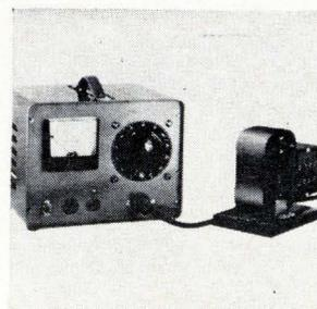
Portable a-c field demagnetizers are designed and built to user's specifications. The laminated core structure permits continuous-duty operation without heating. Peak field strengths are from 0 to 10,000 oersteds, infinitely adjustable. Units are available for 115-v or 230-v operation. Instrumentation division, Thomas & Skinner Inc., 1120 E. 23rd St., Indianapolis 46207. [384]
