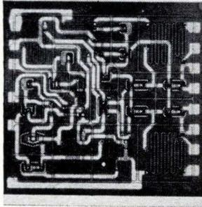
Silicon planar IC operational amplifier UC4000 has an offset voltage adjustable to 0 with external pot. Common mode voltage is  $\pm 10$  v; differential input offset current, 15 nanoamps; differential input offset current drift, 175 picoamps/ $^\circ\text{C}$ ; and input offset voltage drift, 10  $\mu\text{V}/^\circ\text{C}$ . Prices start at \$17. Union Carbide Electronics, 365 Middlefield Rd., Mountain View, Calif. [441]
