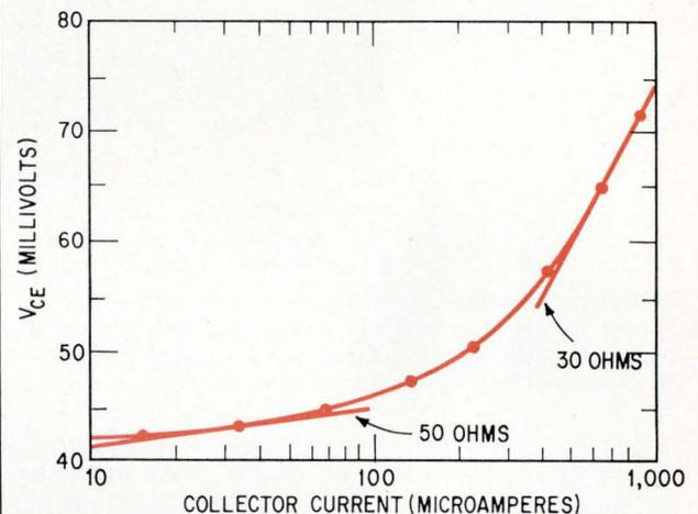
**Voltage-current plot.** Saturation resistance of the transistor varies from 30 to 50 ohms as the collector-to-emitter voltage is increased from 40 to 70 millivolts. The collector current through the transistor is in the microampere range.
