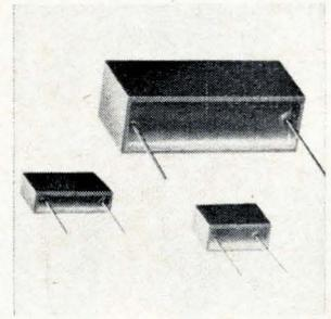
Epoxy-encased metalized mylar capacitors in a molded thin-rectangular configuration with radial leads are designed for high-density circuits. Series 17N is available in 100-, 200-, 400-, and 600-v sizes in capacitance values from 0.001 to 5  $\mu\text{f}$  with 20% to 1% tolerances. Operating temperature is from  $-55^\circ$  to  $+125^\circ$  C. SEI Mfg. Co., 18800 Parthenia St., Northridge, Calif. 91324. [348]
