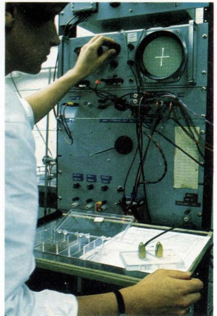
**Final test.** Symmetrical scope pattern tells the operator that there is a good switch in the test contacts on the table.
