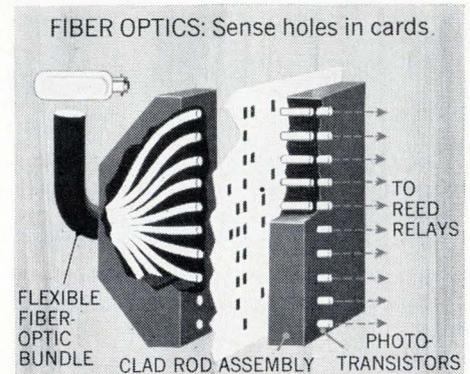
Electro-optical systems incorporating fiber optics are operating at up to four times the speed of electro-mechanical systems. When a combination of fiber optics, phototransistors, and reed relays is used, reading of basic data is not controlled by mechanical limitations. The use of fiber optics allows wide design freedom to increase system operating speed.
