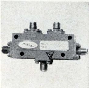
Solid state switch S001350, single pole, double throw, has a switching speed of 100 nsec. Its guaranteed high isolation value is 50 db to 2 Ghz, 46 db to 4 Ghz and low insertion loss of a maximum of 2 db to 2 Ghz, 2.8 db to 4 Ghz. R-f handling capacity is 2 w c-w. The switch weighs under 2 oz. Price is \$375 each. American Electronic Laboratories Inc., Colmar, Pa. [413]
