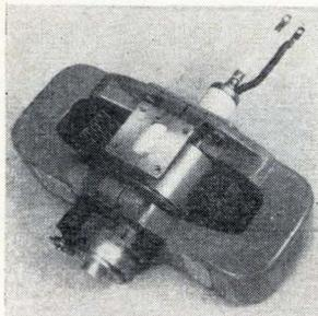
Mechanically tuned, coaxial magnetron model 304 is for use in airborne and ground-based radar systems. It develops 250 kw peak power across the 8.5- to 9.6-Ghz range. The 19-lb, air-cooled tube can be used in existing systems using the 6249 family of tubes. Dimensions are  $9\frac{3}{4} \times 10\frac{1}{4} \times 4\frac{1}{2}$  in. SFD Laboratories Inc., 800 Rahway Ave., Union, N.J. [401]
