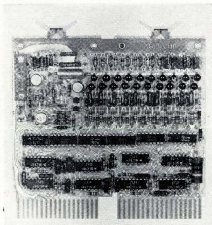
**Machine built.** Entire A/D converter is built on a double-sided board, using plated-through holes. Most components are inserted by machine.
