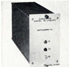
A digital-to-synchro converter accepts a parallel 10-bit binary angle and delivers a synchro signal equal to the digital input. Inputs of the DS800 are compatible with IC logic levels at updating speeds to 10,000 words/sec. Accuracy, no load to full load, is better than 0.5°. The unit's front panel is  $5\frac{1}{2} \times 3\frac{1}{2} \times 8$  in. AstroSystems Inc., 6 Nevada Dr., New Hyde Park, N.Y. [393]
