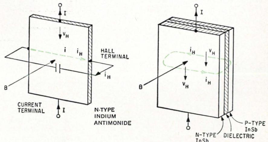
**Inductive slab.** Basic solid-state inductor (left) consists of InSb slab with external capacitor connected to two of its four terminals. Dielectric sandwiched between two slabs gives device internal capacitor.
