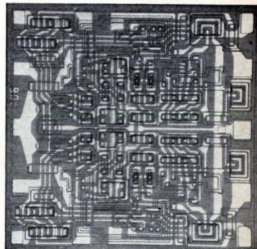
Compatible. DTL flip-flop fits TTL pins.
