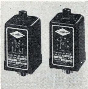
Trans-O-Netic time-delay relay has an interval repeatability of  $\pm 2\%$  at 70° F and 115-v a-c that isn't affected by line variations from 100- to 135-v a-c. Standard time for the delay-on-make model is 1 to 60 sec; for the delay-on-break unit, 1 to 30 sec. Prices range from \$20 to \$26 for sample units. Heinemann Electric Co., 252 Magnetic Dr., Trenton, N.J. 08602. [349]
