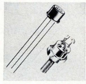
Triple-diffused, planar npn silicon transistors, designated 2400-6 (TO-5 case) and 2800-6 (TO-59 case), are rated 7.5 amps. They range from 30 to 150 v with a typical frequency of 25 Mhz. The TO-5 units, at 10 w, cost from \$6.60 to \$21.40 each on orders of 100. Prices of the TO-59's range from \$8 to \$24. Silicon Transistor Corp., East Gate Blvd., Garden City, N.Y. [439]
