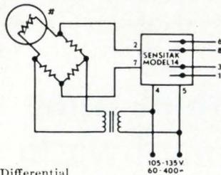
Differential Thermistor (temperature controller)
