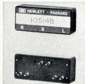
Double-balanced mixer 10514B, measuring  $1.63 \times 0.70 \times 0.43$  in., mounts on p-c boards. Range is 0.2 to 500 Mhz at l-o and signal ports; third port is d-c coupled. Conversion loss is less than 9 db over full range. Uses include pulse modulators, and current-controlled attenuators. Price is \$150. Delivery is from stock. Hewlett-Packard Co., 1501 Page Mill Rd., Palo Alto, Calif. [408]
