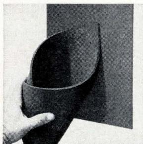
A thin, flexible microwave absorber based on silicone rubber, Eccosorb FGM has an average reflectivity of 12 db down from 2 to 12 Ghz over a wide range of incidence angles. It is usable up to  $425^\circ\text{F}$  continuously, and up to  $500^\circ\text{F}$  for short times. It weighs less than 2 lbs per sq ft. Price is in the \$50 per sq ft range. Emerson & Cuming Inc., Canton, Mass. [407]
