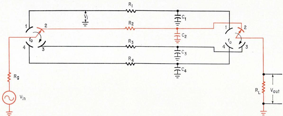
In the series-switched digital filter both the input and output signals are sampled by a pair of rotary switches revolving at a frequency  $f_0$ . Each time a pair of switches close, a quarter of a sine wave appears across the RC filter arm of the circuit. The output is the voltage developed across the grounded capacitor,  $C_n$ .
