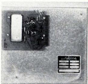
Fully compatible with IC's, the RZ-90 recirculating memory module accepts a variety of delay lines to provide storage capabilities between 20 and 10,000 bits and delays between 20 and 15,000  $\mu$ sec. Applications include sequential information storage for crt displays and programing for numerically-controlled machines. Sealectro Corp., 225 Hoyt St., Mamaroneck, N.Y. 10543. [382]
