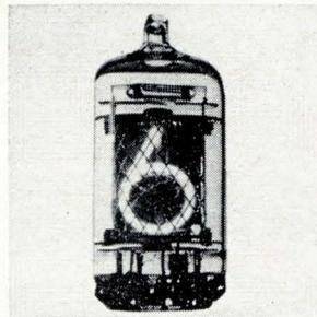
Side-viewing numerical indicator tube CK8650 has conventionally shaped  $\frac{9}{16}$ -in. numerals from 0 to 9 that can be read from distances up to 30 ft and at angles up to 60° from horizontal. Tube diameter is  $\frac{7}{8}$  of an inch. Seated height is 1.8 inches maximum. The indicator tubes are available from stock. Raytheon Co., Industrial Components Operation, 465 Centre St., Quincy, Mass. [351]
