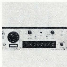
Frequency counter 5247M counts directly from 10 hz up through the communications bands to 135 Mhz. With frequency converter plug-ins, the range can be extended to 18 Ghz. The instrument has a time-base oscillator with short-term stability of better than  $5 \times 10^{-11}$  rms for a 1-sec averaging period. Price is \$3,000. Hewlett-Packard Co., 1501 Page Mill Rd., Palo Alto, Calif. [374]
