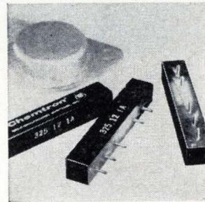
Reed relay series 325-12-1A measures 1.4 x 0.25 in. sq. with 0.1-in. pin spacing for standard p-c layout techniques. Direct p-c mounting eliminates changes in reed characteristics caused by cutting and bending of axial-lead types. The spst contacts switch in less than 1 msec, and are rated at 4 v-a into a resistive load. Self-Organizing Systems Inc., Box 9918, Dallas. [356]
