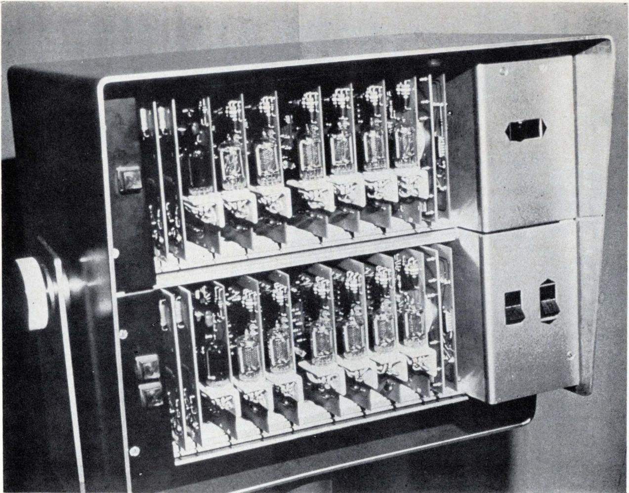
**Inside look.** With front panel removed, each circuit board with its numerical readout tube can be seen.
