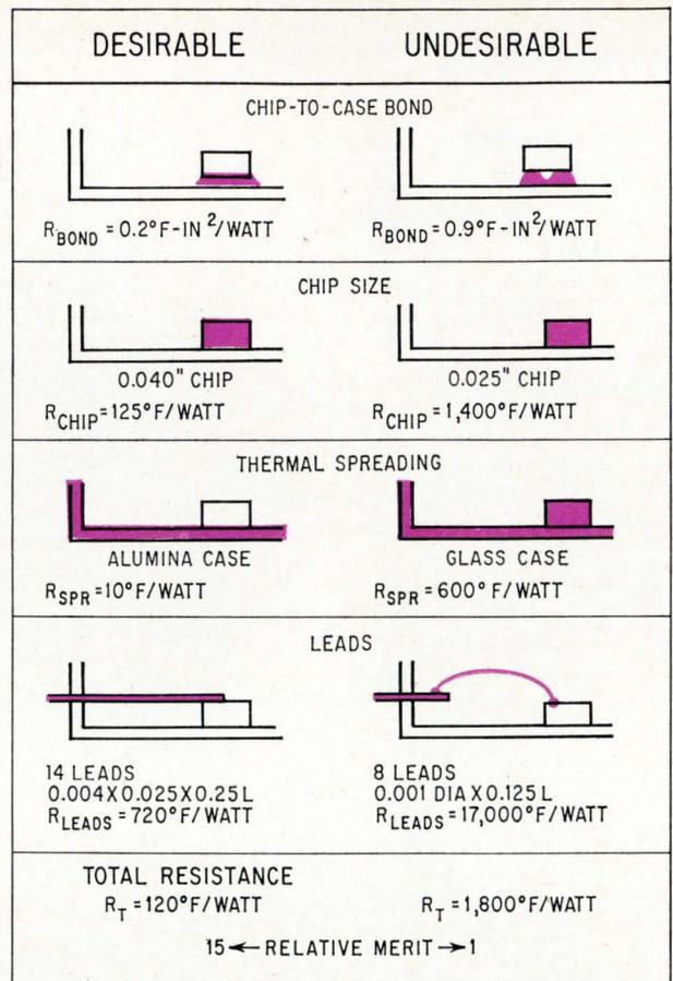
**Package problems.** Thermal characteristics of integrated circuit flatpacks can vary as much as 15:1 because of differences in construction, processes, materials, and dimensions. In each illustration, color shows the part responsible for the thermal resistance value given.
