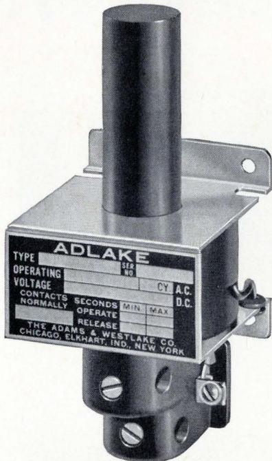
Varying ambient temperatures have little or no effect on Adlake Mercury Displacement Time Delay relays. From the graphic illustrations, ambient temperatures up to 200° F or down to -37.8° F (freezing point of mercury), the change in timing is less than 10%.
