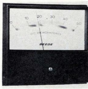
The Centurion line of electrical meters has easy-to-read scales, recessed glass window to minimize marring, and glare-free scale illumination. D-c current sensitivities are available from 5  $\mu$ a through 50 amps with self-contained shunts. D-c voltage sensitivities are from 3 mv through 500 v with self-contained multipliers. Beede Electrical Instrument Co., Penacook, N.H. [362]
