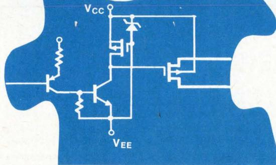
Analog switching got you puzzled? Here's the answer — an integrated circuit with drivers and FET switches all in one package. Drive the input with almost any integrated logic — only 0.8 volt swing is required. The output FET with ON resistance as low as 80 ohms and leakage less than 1 nA can switch plus or minus 20 volt signals.
