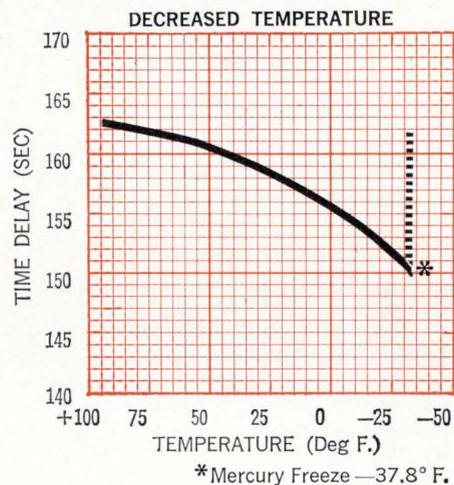
Effect of decreased temperature on time delay characteristics. Curve is typical for a normally open, slow make relay having nominal delay of 160 sec.
