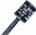
Electrostatically & magnetically shielded output transformer 3/4 D. x 1/4" H. Pri. 15K CT, Sec. 8K CT; max. level 50 mw; audio range response. To MIL-T-27B, grade 4.
