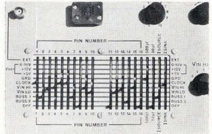
**Programmer.** Operator sets up test conditions with contacts that are pushed by hand over printed circuit program boards.
