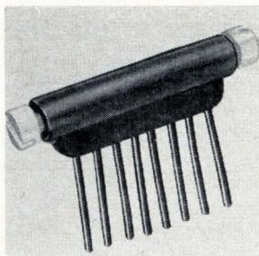
Double tuned i-f transformers, with average dimensions of 0.097 x 0.75 in., can be mounted between hybrid amplifier cans. Operating frequency is 1 to 100 Mhz. Typical temperature coefficient is  $\pm$ 65 ppm/°C from -55° to +125°C. The transformers can contain up to 4 windings, and are suited for r-f and i-f strips. Piconics Inc., North Billerica, Mass. 01862. [347]
