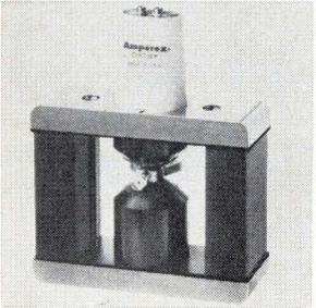
A rising sun magnetron that delivers 5-nsec pulses of 95-Ghz energy at 10 kw has a 3.2-mm wavelength output. Output figure of the DX287 lies in the center of an atmospheric window where the attenuation is much lower than that at other frequencies in the mm region. Duty cycle of 0.002 allows repetition rates to 40 khz. Amperex Electronic Corp., Hicksville, N.Y. [405]
