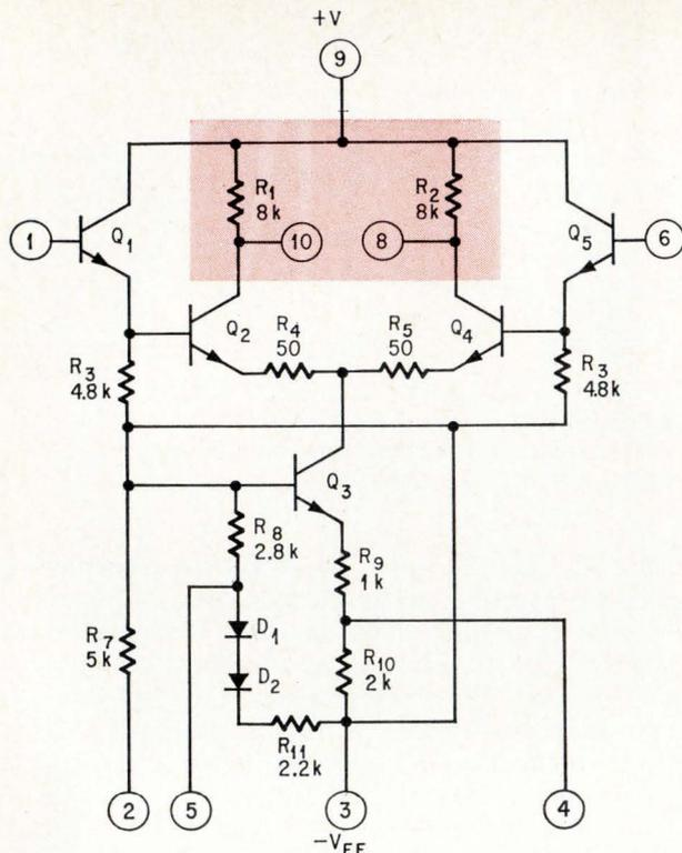
**Video.** Presence of diffused resistors,  $R_1$  and  $R_2$ , in collector legs of the amplifier marks video-type IC.
