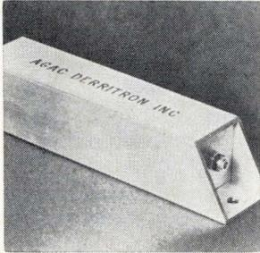
Battery-operated preamplifier series PA uses a noise-canceling circuit and features an rms-integrated broadband noise level below 10  $\mu\text{V}$ . Input impedance is 1,000 megohms; frequency range, 0.2 hz to 100 khz. Models are available in fixed gains of 0, 10, 20, 40, and 60 db, and variable gains of 0 to 20 and 20 to 40 db. Agac-Derritron Inc., 600 N. Henry St., Alexandria, Va. [385]
