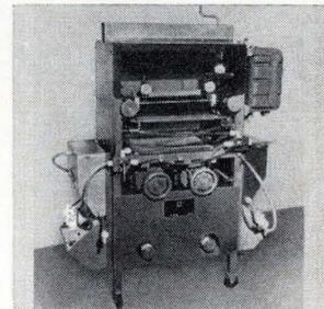
Roller coater for applying thin-film photoresist materials to p-c boards has a double-pumping system for automatic cleanup, ground rolls, dial indicators for thickness adjustment, and separate drive systems for doctor roll and coating roll. Coater operates at any speed from 3 to 9 ft per minute. The unit will accept boards up to 1 in. thick. Union Tool Corp., Warsaw, Ind. [428]
