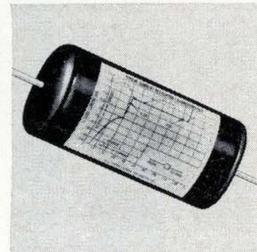
Current-regulating diodes with working currents from 0.22 to 4.7 ma come in a 32-device series. The 1N5283 through 1N5314 are field effect diodes that provide constant currents independent of voltage. Devices offer a peak operating voltage of 100 v, 600 mw power dissipation. Prices are from \$4.90 for 100 units. Motorola Semiconductor Products Inc. Phoenix, Ariz [439]
