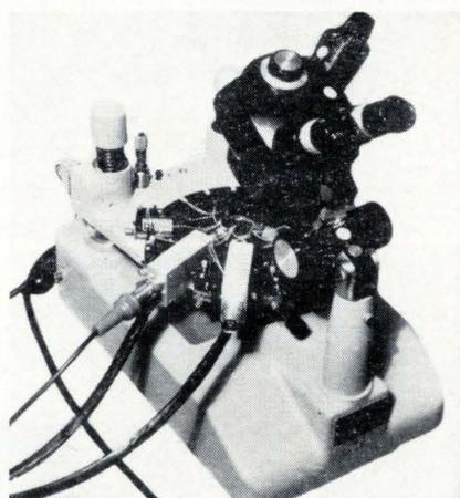
**Wafer probe.** Tester's discriminator heads are attached directly to a standard semiconductor-wafer probe.
