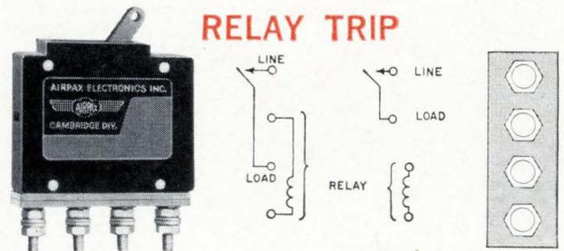
In protector Types APL-4 and -5, coil and contacts terminate at separate pairs of terminals. With this configuration, you can control current in one circuit by a different current in a separate circuit.
