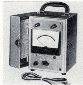
Portable ohmmeter 244 has 0.5% accuracy at center scale. It makes direct readings of resistances from 0.05 to 50,000 ohms. It is calibrated in 4 ranges: 0 to 50, 0 to 500, 0 to 5,000, and 0 to 50,000 ohms. Accuracy is assured by a built-in standard that compensates for battery condition and lead resistance. Associated Research Inc., 3777 W. Belmont Ave., Chicago. [363]
