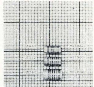
Molded chokes come in 3 types. Models 3710-1 through -7 cover inductances from 47 to 150  $\mu$ h in a 0.250 x 0.560-in. package. Q values range from 18 to 75. Models 3711-1 through -5 cover 180 to 390  $\mu$ h, are 0.310 x 0.560-in. with 80 to 75 Q's. The 3712-1 through -5 cover 470 to 1,000  $\mu$ h and are 0.375 x 0.625 in. Cambridge Thermionic Corp., 445 Concord Ave., Cambridge, Mass. [348]
