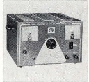
Heavy-duty, solid state supplies series PSR-500 deliver continuously variable 500-w outputs with regulation of line or load to less than 1%, no load to full load. Ripple is less than 1% at max. rated current. Three models are available: 2-32 v d-c, 0-15 amps; 2-55 v d-c, 0-10 amps; and 2-125 v d-c, 0-5 amps. Electro Products Laboratories Inc., 6125 Howard St., Chicago. [388]
