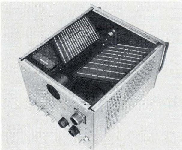
**Chevron.** Air stream cools more efficiently when circuit cards are placed at 120° angle rather than the usual 90°.
