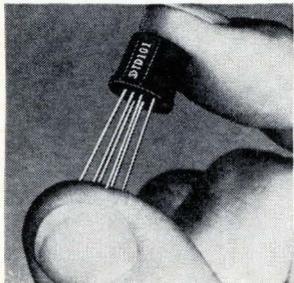
Plastic complementary silicon transistors rated at 360 mw with a maximum operating junction temperature of 150°C can be used to replace the standard 2N2222 series. The TD100 meets MIL-S-19500/255E, with a noise figure of 0.5 db and a minimum gain of 100 at 10  $\mu\text{a}$ . Base-to-emitter voltage is matched within 2.5 mv. Sprague Electric Co., North Adams, Mass. [440]
