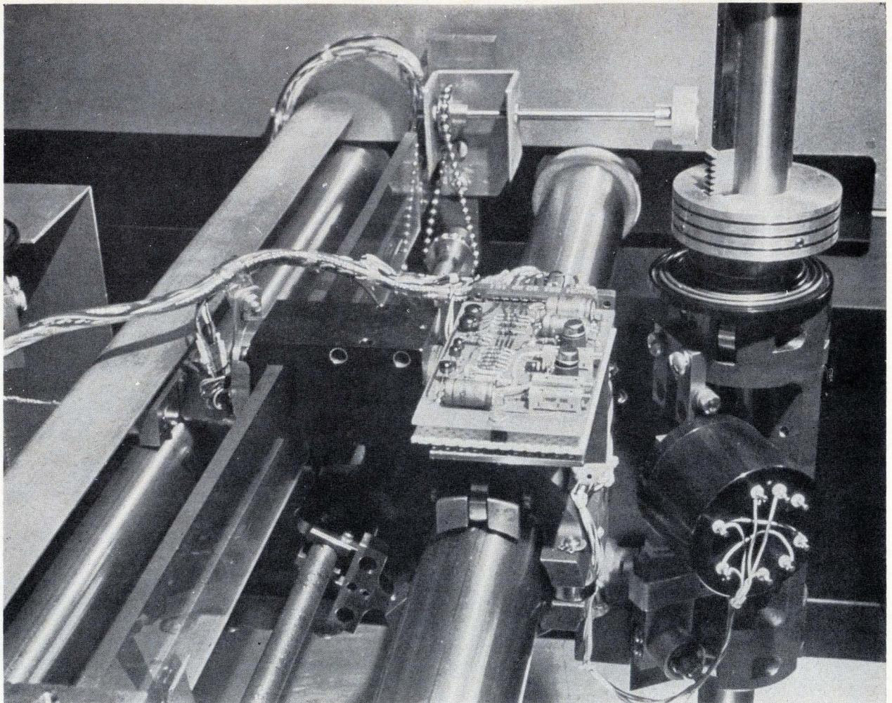
**On location.** D-c amplifiers are so small they can be mounted on the bridge inches from the optical transducers.
