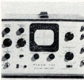
Dynamic flutter analyzer 720 provides precise analysis and measurement of tape recorder flutter. The built-in oscilloscope identifies and measures all flutter-contributing components from 0.2 hz to 10 khz. The analyzer includes a crystal-controlled reference-frequency oscillator. Both sine- and square-wave outputs are provided. Vidar Corp., 77 Ortega Ave., Mountain View, Calif. [369]
