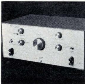
Portable transient generator model 4881 determines the ability of equipment and systems to withstand sudden changes in a-c or d-c power supply sources. Pulse amplitude is variable from 0.1 to 300 v; peak pulse power is 43 kw, 0.5-ohm load; and synchronous pulse positioning, 0° to 360° on power line waveform. Honeywell Inc., P.O. Box 391, Annapolis, Md. 21404. [365]
