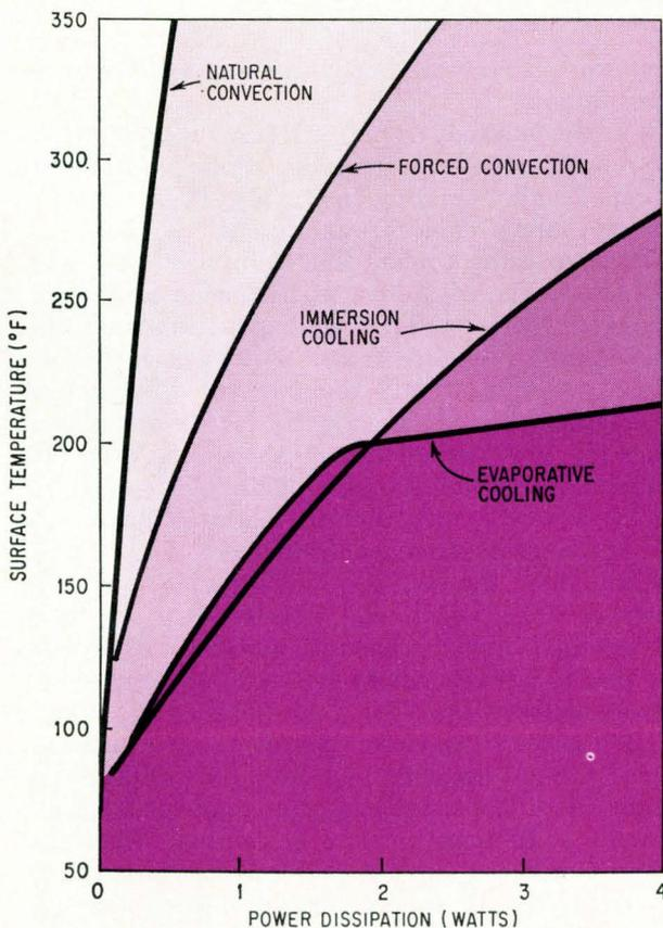
**Tradeoff curves.** Quick comparisons between alternate cooling techniques can be made with families of curves. Efficiency rises and size decreases from left to right in this comparison of methods for cooling TO-5 packages.
