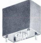
Primary 10 ohms, secondary 530K ohms, 230:1 ratio, response from 1/2 cycle to 25 cycles. 120 db magnetic shielding, plus full electrostatic shielding.
