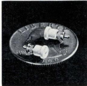
A semi-assembled feed-through terminal is for installation in a 0.040-in.  $\pm$ 0.02-in.-thick chassis, mounting in a 0.136-in. hole. Designated FT-2-SM-1200, the terminal's 0.040-in. diameter gold-plated brass lug extends 0.100 in. above and below the Teflon bushing. The unit handles 5.5 amps and can be used from 65° to 200°C. Sealectro Corp., 225 Hoyt St., Mamaroneck, N.Y. [342]
