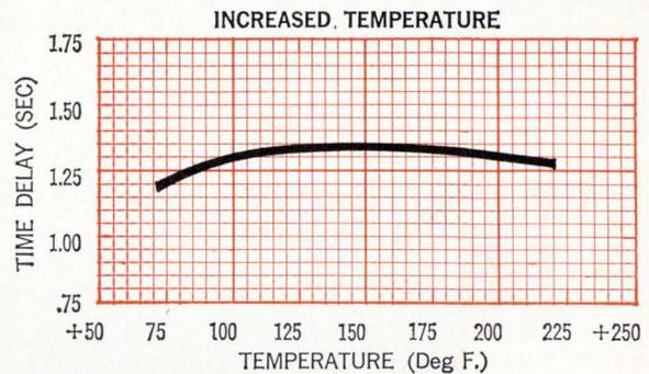
Effect of increased temperature on time delay characteristics. Curve is typical for a normally open, slow-make relay having nominal time delay of 1.25 seconds.
