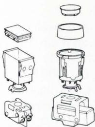
**Series 2** offers both rectangular and round display, permitting shape-coding of stations or group functions. Snap-in mounting. Solenoid pull-in and/or hold-in coil for remote control.
