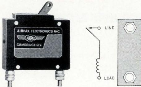
Airpax APL circuit protectors are manufactured in five circuit configurations. Each is available in any of 10 time delays, in any of 16 standard trip levels, and rated for a maximum of either 50 vdc, 250 vrms at 60 Hz, or 250 vrms at 400 Hz.
