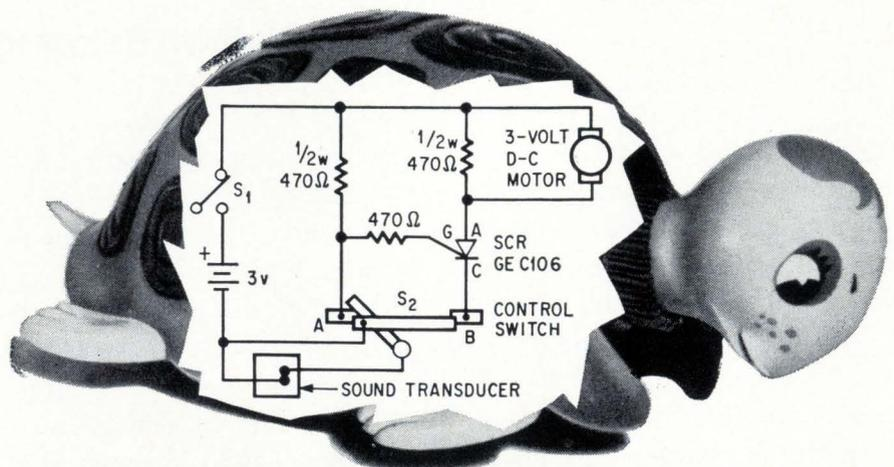
**Shell game.** Here's how Remco Industries is using an SCR to start and stop a battery-operated motor inside a toy turtle.
