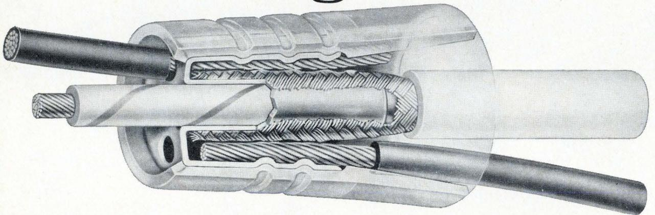
Uniring combines inner and outer ferrules in unitized construction. Simply insert a stripped conductor and tap wire, then crimp. One crimp does it. No heat. No burnt cables.
