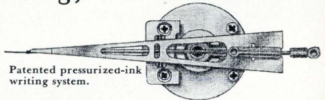
protected from overloads as high as 500 volts. Pressurized writing puts smudge-proof traces into paper, and there's enough ink in the throwaway cartridge to last for about
