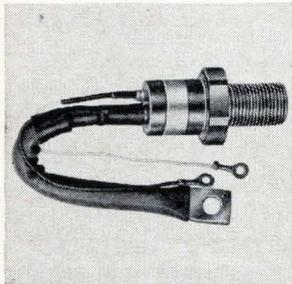
Series NL-C180 are silicon controlled rectifiers with voltage ratings from 100 to 1,300 v. Devices are all-diffused, shorted-emitter types with 235 amp rating. Minimum  $dv/dt$  rating is 200  $v/\mu\text{sec}$ ; maximum  $di/dt$  ratings, up to 100  $\text{amps}/\mu\text{sec}$ . Peak on-voltage is 1.8 v. Hard solder construction yields low thermal fatigue. National Electronics Inc., Geneva, Ill. [436]
