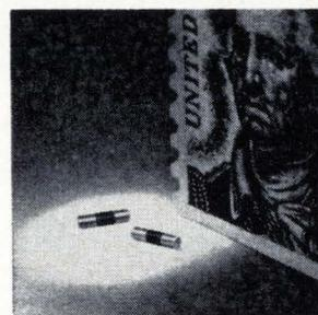
A resistor 0.040 in. in diameter and 0.130 in. long operates from  $1 \times 10^8$  to  $1 \times 10^{12}$  ohms with a tolerance of  $\pm 25\%$ . It handles temperatures to  $100^\circ\text{C}$  and with a compatible epoxy can be readily encapsulated. The ends of the resistor serve as terminals for direct soldering to terminal board and circuit component connections. Pyrofilm Resistor Co., 3 Saddle Rd., Cedar Knolls, N.J. [355]
