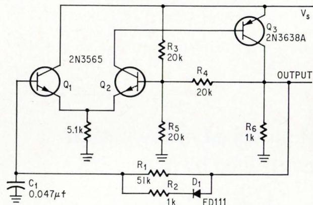
**Nonsymmetrical multivibrator.** Capacitor  $C_1$  is charged through  $D_1$  and  $R_2$  until  $C_1$ 's potential reaches  $\frac{2}{3} V_s$ .
