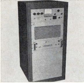
Frequencies from below 200 khz to above 220 Mhz are amplified linearly more than 50 db to power levels up to 400 watts by the M404A laboratory amplifier. No tuning is needed. Applications include communications systems, rfi tests, antenna research programs, and nuclear magnetic resonance work. Instruments for Industry Inc., 151 Toledo St., Farmingdale, N.Y. 11735. [381]
