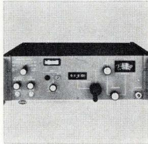
L-band signal generator model 1105 covers the 0.95 to 2.4 Ghz range. The manufacturer's Unidial control system provides single-band continuous tuning with digital frequency indication accurate to  $\pm 0.5\%$ . Frequency stability is 0.0008% per volt change in line voltage and 0.005% per  $^{\circ}\text{C}$  change in ambient temperature. Polarad Electronic Instruments Inc., 34-02 Queens Blvd., L.I.C., N.Y. [407]
