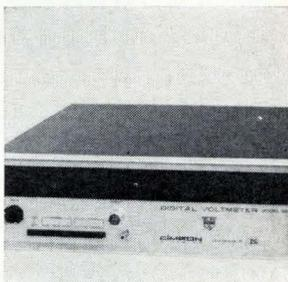
Programable, digital volt-ratio meters series 6600 handle 1,000 samples per sec. Accuracy is within  $\pm 0.01\%$  of full scale  $\pm 0.017\%$  of reading for 6 months over a temperature range of  $10^\circ$  to  $40^\circ\text{C}$ . With the optional millivolt preamp accessory, the 6600 automatically ranges from  $+10.999$  mv to  $\pm 1099.9$  v d-c full scale. Lear Siegler Inc., 1152 Morena Blvd., San Diego, Calif. [376]
