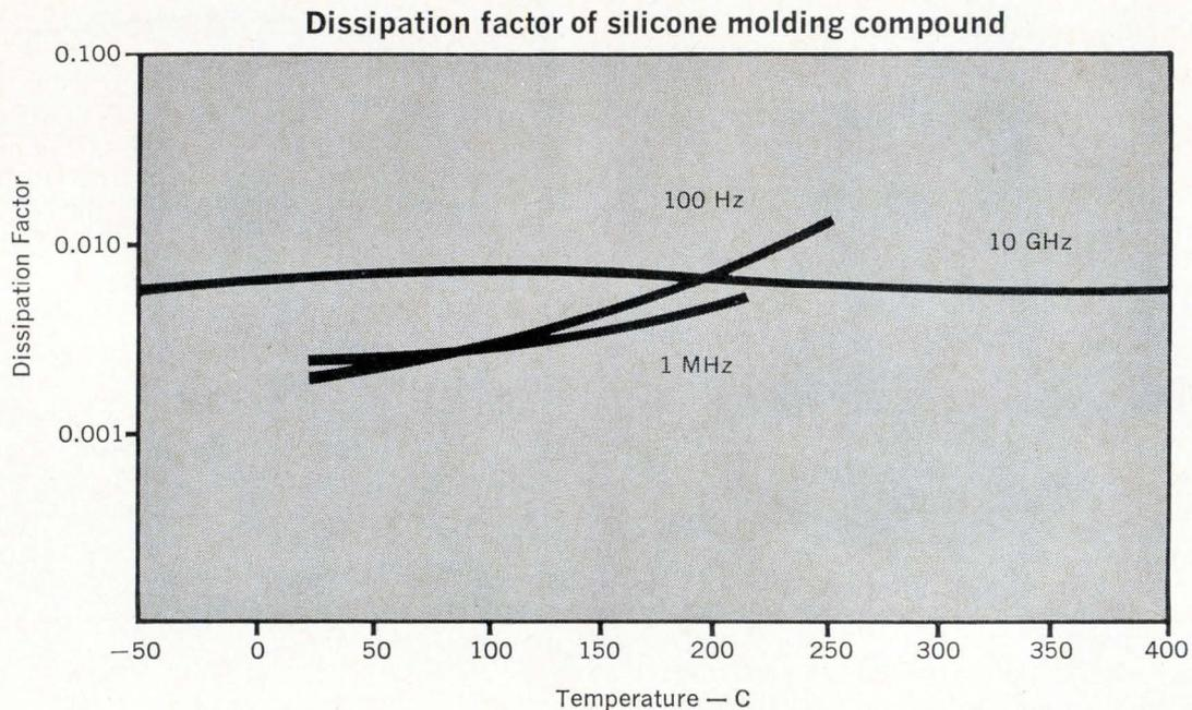
Why the big swing to silicone molded devices? . . . Electrically stable materials over a wide range of temperatures from low to high frequencies—as shown graphically above. Silicone molded packages do not limit the design or performance of high frequency semiconductor devices. Design characteristics will not drift due to changing electrical properties of the molded package.
