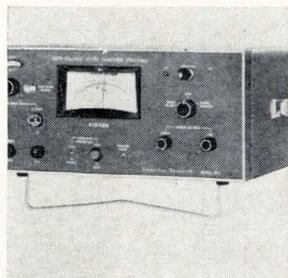
Automatic transfer standard model ATS is a true rms to d-c converter that makes a measurement in 10 seconds for frequencies from 2 hz to 10 Mhz. Accuracies are: 0.1% for a-c signals up to 1,000 v and to 20 khz; 0.02% up to 500 v and to 50 khz; 0.05% up to 16 v and to 1 Mhz; 0.5% up to 8 v and 10 Mhz. Singer Co., 915 Pembroke St., Bridgeport, Conn. [370]
