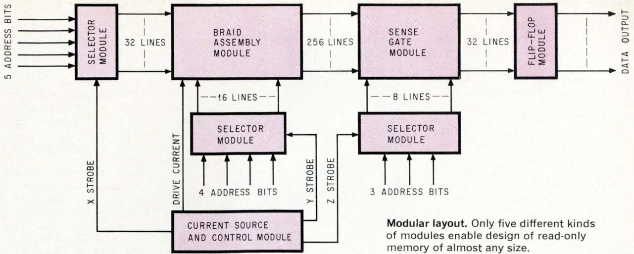
**Modular layout.** Only five different kinds of modules enable design of read-only memory of almost any size.
