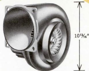
**CENTRIFUGAL BLOWERS** — Unique "centrifugal" impellers. Far more efficient and economical than squirrel cage blowers of similar capacity. For high quality commercial equipment ranging from office copiers to large capacity computer disc memories. • 14-545 cfm • Wheel sizes from 2" to 7". • Convenient mounting options • Working pressures to 3" wg. • 115 VAC, 60 CPS, single phase; 230 VAC, 50 CPS, single phase; 208-230 VAC, 50-60 CPS, three phase. • No maintenance. • Lubricated for life.
