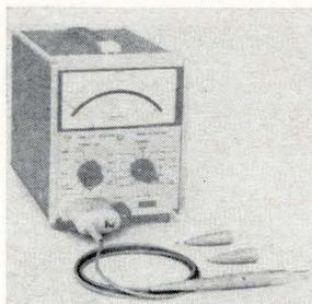
H-f probe 11096A converts d-c voltmeters into a-c instruments that measure signals from 100 khz to 500 Mhz. Accuracy in this range is better than 1 db. Input impedance is 4 megohms shunted by 2 pf. The probe works with analog or digital voltmeters that have input resistances of 10 megohms  $\pm 10\%$ . Price is \$45. Hewlett-Packard Co., 1501 Page Mill Rd., Palo Alto, Calif. [371]
