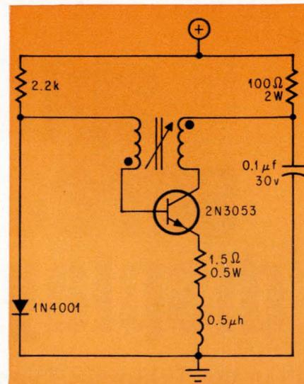
**Service free.** Breakerless trigger would end point resetting and retiming.
