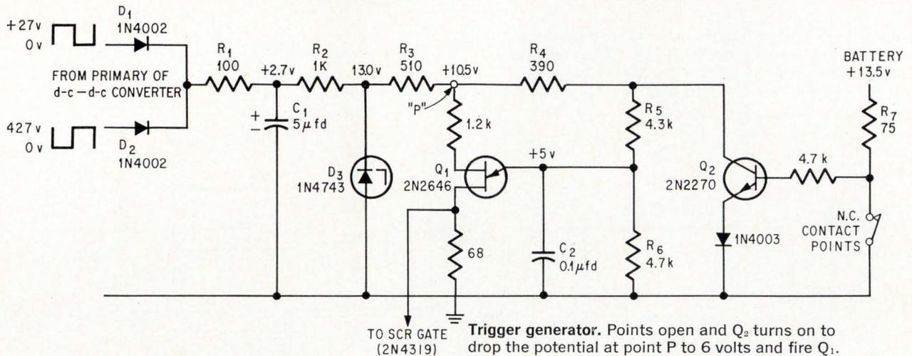
**Trigger generator.** Points open and  $Q_2$  turns on to drop the potential at point P to 6 volts and fire  $Q_1$ .
