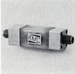
Miniature d-c block, model 754, has a capacitance in series with both the center and outer conductors preventing a flow of d-c current while permitting an uninterrupted flow of r-f power. Typical specifications at 6 Ghz include a vswr of 1.20 max; insertion loss, 0.25 db max; impedance, 50 ohms; and d-c voltage, 100 v. Kevlin Manufacturing Co., 24 Conn St., Woburn, Mass. [406]
