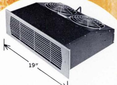
**CABINET COOLING PANELS** — For flushing 19" rack mounted equipment, these panels offer Rotron standards of quality and reliability in 5 1/2" & 7" heights. Large capacity, washable filters insure clean air • 155-400 cfm • Ball bearing induction motors • MIL spec or commercial quality • 50/60 Hz or 400 Hz, single or three phase • Quiet operation.
