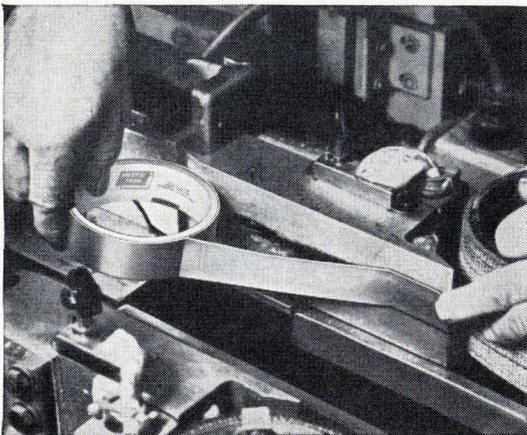
Mystik's Teflon tapes combine the advantages of TFE Teflon film with a silicone pressure-sensitive adhesive. As a result, they offer high dielectric strength, low coefficient of friction, and high performance within a temperature range from  $-100^{\circ}\text{F}$  to  $+450^{\circ}\text{F}$ .
