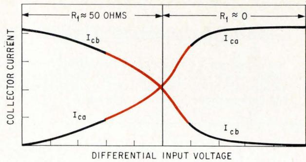
**Shaping.** Emitter degeneration, introduced by placing a resistor component in the emitter circuit, alters the shape of the transfer characteristic and the linear range.
