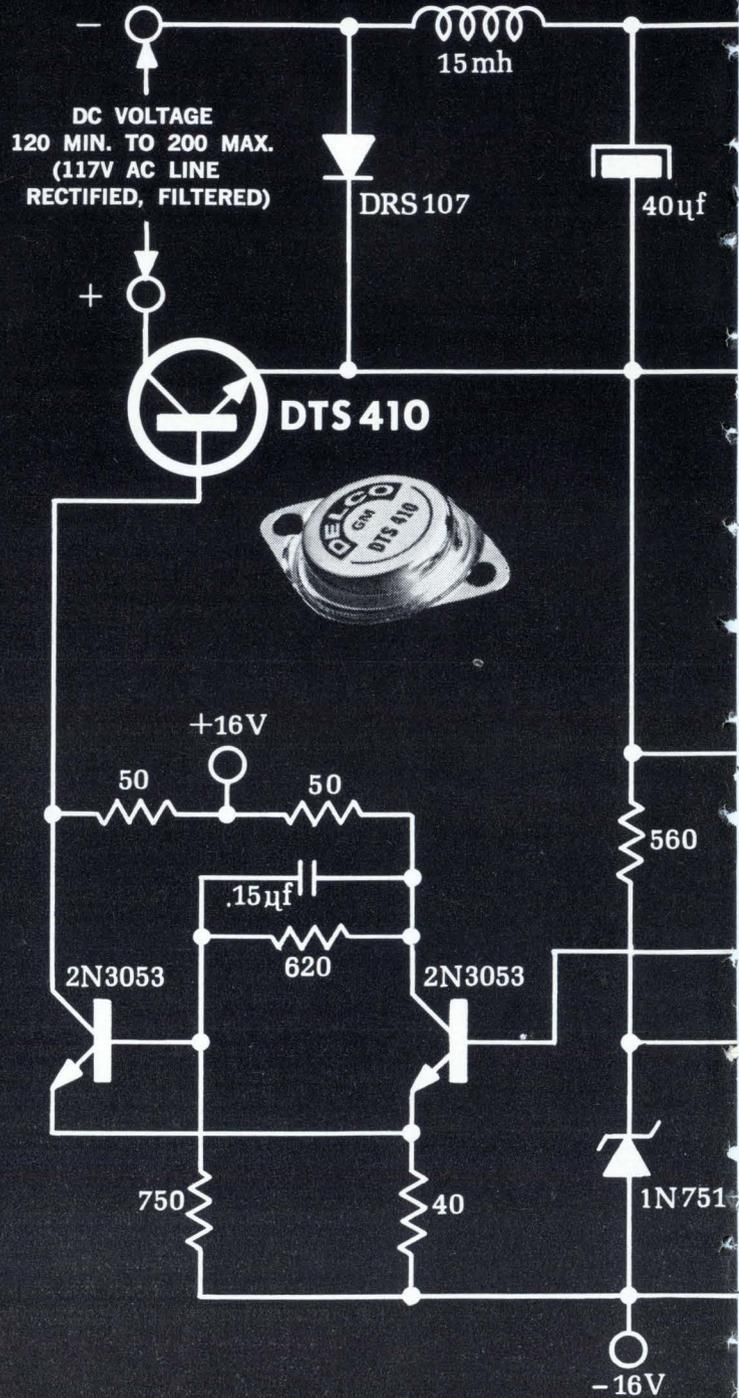
**Application of Delco high voltage silicon power transistors**
