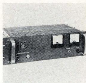
Frequency converter CRS-150A converts 50 or 60 hz single-phase input power to precision, low-distortion 400 hz single-phase output. It delivers 150 v-a, with continuous duty in ambients of  $-20^\circ$  to  $+60^\circ\text{C}$ . Its sine-wave output has less than 1% total harmonic distortion. Frequency regulation is  $\pm 0.25\%$ . CML Inc., 350 Leland Ave., Plainfield, N.J. 07062. [372]
