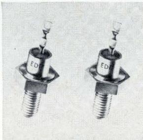
Fast recovery 12-amp silicon rectifiers designated JAN 1N3889 through 1N3893 meet MIL-S-19500/304(EL) specs. The series is for high-reliability military equipment using high-frequency sine wave, square wave or pulsed inputs. Applications include inverters, modulators, converters, and accelerators. Electronic Devices Inc., 21 Gray Oaks Av., Yonkers, N.Y. 10710. [442]
