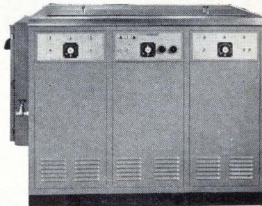
Gives you a combination of solvents, time, power control and unlimited processing sequences to handle both oil and mineral salt cleaning problems. Available with two ultrasonic cleaning tanks (of 5, 10 or 20 gallon capacities) and a vapor rinse tank. 0 to 100% power control with 0 to 15 minute timers on each of the generators.
