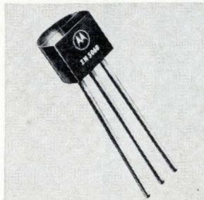
Sensitive gate scr's 2N5060-2N5063 are rated at 800 ma (forward current rms) with voltage ranges from 30 to 150 v in a TO-92 Unibloc plastic package. Gate current requirement is 200  $\mu\text{a}$ . Uses are in fractional h-p motor controls, sensing and detection circuits. Prices range from 51 to 85 cents (100 and up). Motorola Semiconductor Products Inc., Box 13408, Phoenix, Ariz. [441]
