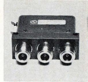
A remote coaxial switch, with  $10^6$  cycles minimum lifetime, is a spdt unit with a range of d-c to 12.4 Ghz. Isolation is 60 db minimum over entire range. Insertion losses as low as 0.3 db from d-c to 7 Ghz and 0.6 db from 7 to 12.4 Ghz are claimed. SR-2 series switches are available with N, TNC, BNC, or RSM connectors. RLC Electronics Inc., 25 Martin Pl., Port Chester, N.Y. [404]
