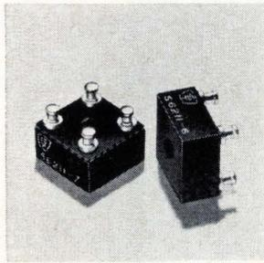
Miniature single-phase bridge rectifier assemblies with ratings up to 2,500 piv mount to p-c boards with one screw; terminals are silver-plated brass for easy soldering. Devices offer piv's of 1,500, 2,000, or 2,500 at current ratings of 1.2, 0.8, or 0.6 amps respectively. Price is \$3.27 each in lots of 1,000. Sarkes Tarzian Inc., 415 N. College Ave., Bloomington, Ind. [350]
