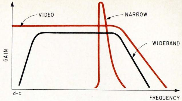
**Delineation.** Gain-versus-frequency characteristic of differential amplifiers is used to distinguish major types.
