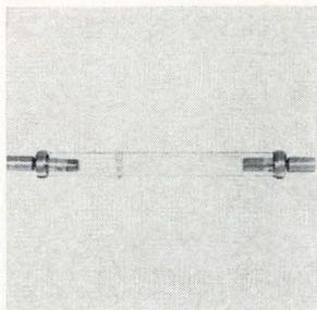
Linear xenon flashtube model FX 81-4 has a 4-in. arc length. The 10 x 12 mm quartz device handles an energy input of 3,000 joules per flash with a pulse duration of 1.4 msec. Units can be used in environments ranging from ocean depths to outer space. Applications include laser stimulation, medical research, and satellite flashers. EG&G Inc., 160 Brookline Ave., Boston, Mass. [346]
