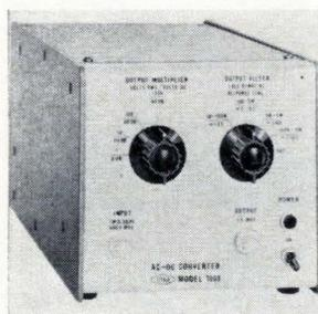
Suited for swept frequency measurements, model 1008 a-c/d-c converter has a 70-db dynamic range, a frequency response from 5 hz to 5 Mhz, and a 300- $\mu$ v sensitivity. It is applicable for audio and video measurements such as those encountered by telephone companies and filter manufacturers. Pacific Measurements Inc., 940 Industrial Ave., Palo Alto, Calif. [366]
