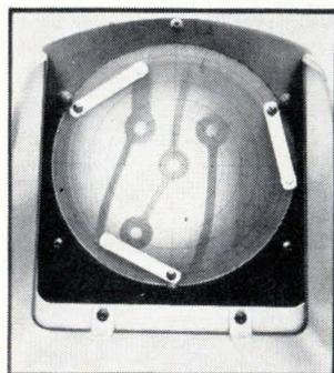
**Auxiliary.** Optical attachment projects circuit board being measured on the screen.
