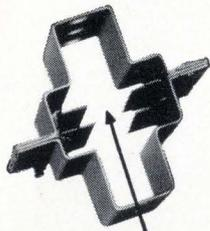
Cavity plate made of heavy-gauge carbonized nickel and subjected to special vacuum-firing process. Combination reduces level of occluded gas and minimizes gas emission during periods of high-overload-temperature.
