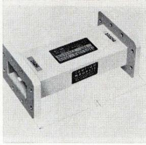
A line of waveguide isolators is based on a patented design that eliminates the external magnet. Series covers 5,925-7,125 Mhz frequency range. Units have 20, 30, or 40 db isolations with maximum losses of 0.5 to 0.8 db. Bilateral vswr is 1.15 maximum. Devices can be furnished with magnetic shielding. E&M Laboratories, 7419 Greenbush Ave., North Hollywood, Calif. [402]
