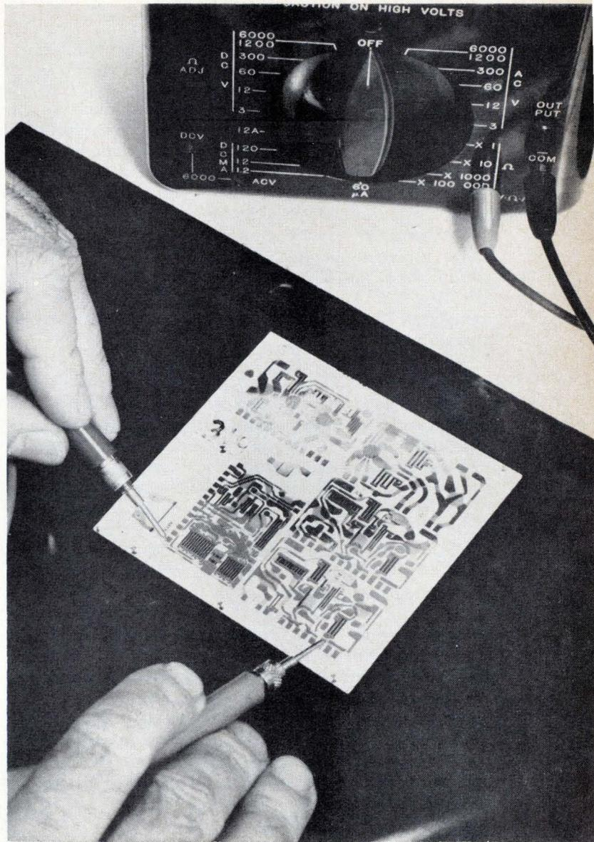
**Heaters.** Thin-film resistors can be deposited on hybrid circuit substrates to control their temperature by controlling power dissipation. These experimental circuits contain extra heating resistors.
