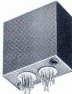
Two transformers each 600  $\Omega$  primary, 40K  $\Omega$  C.T. secondary 250 cycles to 5 KC within 1/4 db. 40 db isolation over band.
