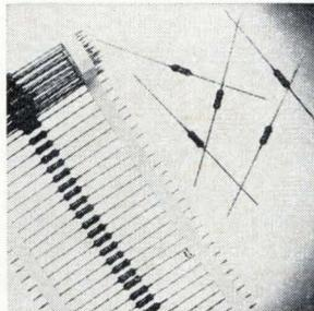
Metal alloy film resistor MAL-20 is a 1/2 watt (70°C) semiprecision device for use in color-tv, computers, and industrial instrumentation. It has temperature coefficients of 100 and 150 ppm/°C, and resistance tolerances of 2 and 5%. The unit meets or exceeds requirements of MIL-R-22684. It is epoxy coated and stamped and color-coded. Mallory Controls Co., Frankfort, Ind. [343]
