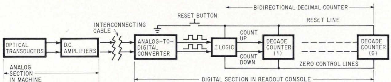
**System design.** Both the horizontal x- and y-axis of the machine sense probe movement with linear optical transducers and convert signals to digital form. The z-axis uses rotary position encoder to save space.
