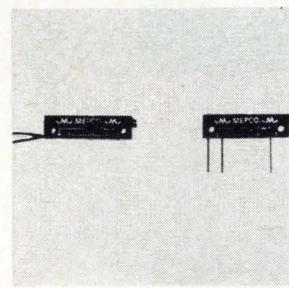
Fired-film trimming pots for the industrial market, designated Acutrim, have all-welded construction, with a stainless steel 1-piece lead screw and a slider that insures long resistance element life. They have infinite resolution, a range from 100 ohms to 1 megohm, and exceed requirements of MIL-R-22097, Characteristic B, Type RJ12B. Mepco Inc., Columbia Rd., Morristown, N.J. 07960. [354]
