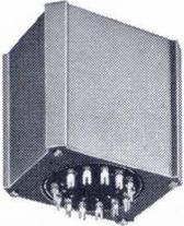
Transistor output; matches any PP transistor to 4, 8, 16  $\Omega$  speaker. Primary 48, 36, 12  $\Omega$  C.T.; 20  $\sim$  to 20 KC; 40 watts.
