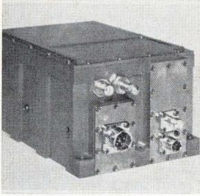
A uhf/f-m transmitter for aerospace telemetry applications delivers 20 w minimum at S-band frequencies in the 2.2- to 2.3-Ghz range. The 3620-01 withstands 20, 55 g shock, 20 g sine-wave vibration, and 30 g acceleration environments. Center frequency stability is within  $\pm 0.003\%$  under all environmental conditions. Electro-Mechanical Research Inc., Box 3041, Sarasota, Fla. [401]
