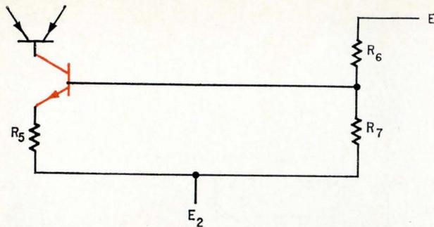
**Current sink.** Use of constant current source in place of large resistor in the common-emitter circuit improves common-mode rejection and simplifies monolithic fabrication.
