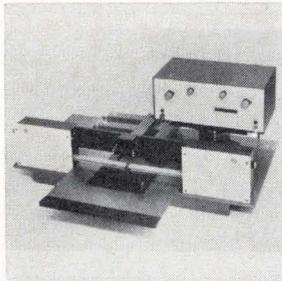
Pantograph reflow-soldering system RS-334 consists of a power supply, 2 reflow-soldering heads, a pantograph p-c board positioning mechanism, and an IC loading/placement fixture. It positions an IC on its mounting board and solders as many as 14 leads at once. Each soldering head has interchangeable electrode-tip configurations and sizes. Sippican Corp., Mattapoisett, Mass. [422]
