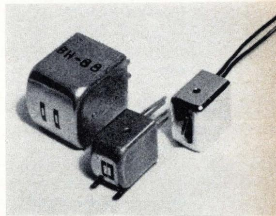
Japanese heads. Standard stereo, Cassette stereo, and film projector heads (from left to right) are being made with the new plating process.
