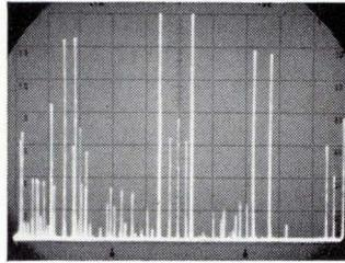
Normal wideband spectrum display of high-level multiple signals. (2 GHz spectrum width, 10 dB/cm vertical display.)
