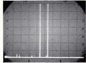
Virtual elimination of normal intermodulation products produced by strong multiple signals at the analyzer input.
