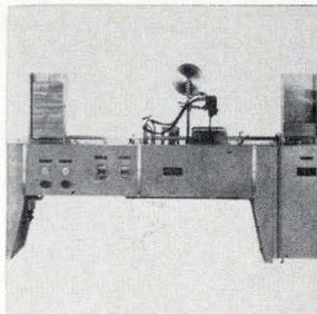
HD-3 remote masking-spray coater, TL-1 automatic tray-loading machine, and ML-1 magazine loader are for continuous automatic wet or powder application to axial-lead components. They handle from 3,000 to 10,000 components per hour, depending on sizes. After spray coating, the ML-1 stacks 40 loaded trays for baking or storage. Conforming Matrix Corp., Toledo, Ohio. [427]
