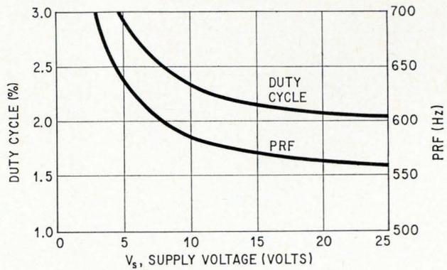
**Performance curves.** Supply voltage  $V_s$  may drop from 24 to 12 volts with little change in the output's PRF.
