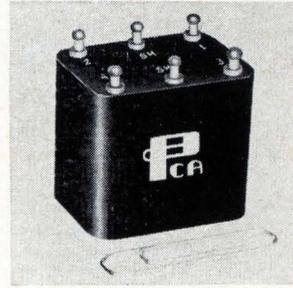
An interstage pulse transformer—1 cu in. in volume and weighing 75 grams—operates up to 50,000 ft, withstands thermal shock and h-f vibration to 50 g, and environmental temperature from  $-54^\circ$  to  $+110^\circ\text{C}$ . With a working voltage of 10 kv d-c, it has a 1:1 turns ratio, a 0.05- $\mu$ sec rise time, and meets MIL specs. PCA Electronics Inc., 16799 Schoenborn St., Sepulveda, Calif. [352]
