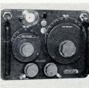
Impedance bridge 1606-B, adaptable to coaxial connectors, measures in the 400-khz to 60-Mhz range. Resistance range of the bridge is 0 to 1,000 ohms, and reactance range is  $\pm 5,000$  ohms at 1 Mhz. At other frequencies the reactance reading must be divided by the frequency in megahertz. Price is \$1,050. General Radio Co., West Concord, Mass. 01781. [375]
