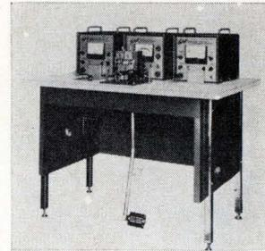
Model 1400 console enables the welding of insulated tape cable to itself or to connector terminals without prestripping the insulation. It includes 2 a-c power supplies, 1 d-c supply, an a-c/d-c controller, and a weld head with 4 electrodes (2 above and 2 below the items being welded). Copper-to-copper welds take 1/2 sec. Wells Electronics Inc., 1701 S. Main St., South Bend, Ind. [424]
