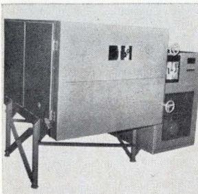
Temperature heating rate of  $-100^\circ\text{F}$  to  $200^\circ\text{F}$  in 2 hours and cooling rate of  $200^\circ\text{F}$  to  $-100^\circ\text{F}$  in 1 hour are featured in an environmental Thermaline vibration chamber that is insulated with nonsetting, nonhygroscopic Fiberglas/Foamglas. Control is maintained to within  $\pm 3^\circ\text{F}$ . Environmental Engineering Division, Bethlehem Corp., 225 W. 2 St., Bethlehem, Pa. [425]
