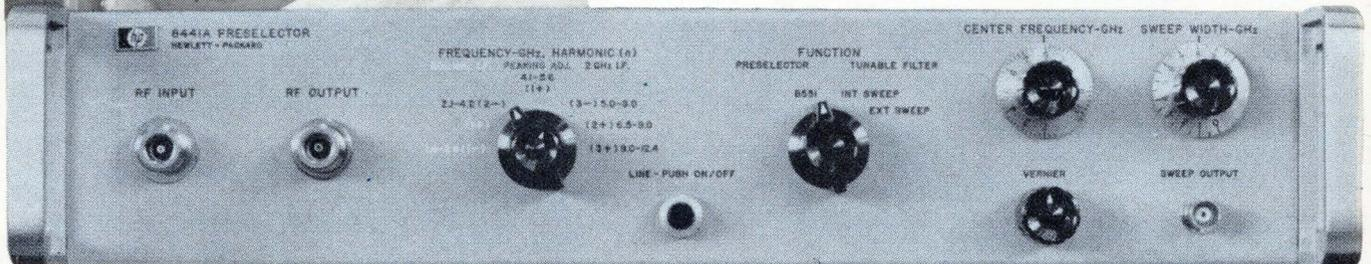
The new HP 8441A Preselector offers an effective solution to the cluttered-screen problems often encountered in broadband spectrum analysis. Used with the HP 851/8551 Spectrum Analyzer, the preselector covers 1.8 to 12.4 GHz with simple, straight-forward operation. Broadband and multiple signal displays are now far easier to interpret.
