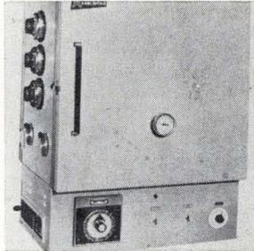
Test chamber Z0HP-3 is designed to provide stable life-test temperature conditions for in-chamber parameter measurements of semiconductor and axial-lead components mounted to p-c boards. It provides for life-test temperature environments from 100° to 400°F with a stability of  $\pm 0.25^\circ\text{F}$ , utilizing a laminar air flow. Associated Testing Laboratories Inc., 200 Rt. 46, Wayne, N.J. [423]
