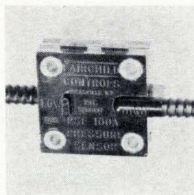
Pressure sensor PSF100A senses level changes in liquids, granular powder semisolids, equivalent to 1/2 in. or less of water column or pressure/vacuum and differential in the same range. It is virtually insensitive to shock, vibration, and acceleration. It is 1 x 1 x 1 1/32 in., and weighs less than 10 grams. Fairchild Camera & Instrument Corp., 225 Park Ave., Hicksville, N.Y. [367]
