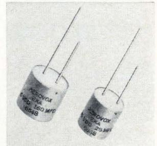
Plastic-cased electrolytic tubular capacitors with epoxy end sealing are designed for p-c transistor circuitry and miniature electronic assemblies. Type EKA units come in 11 different models with capacitance values from 5 to 250  $\mu$ f; and in 3 sizes, the largest being 1 $\frac{1}{32}$  x 3 $\frac{1}{4}$  in. D-c voltage ratings include 3, 6, 10, 15, 25, 35, and 70. Aero'ox Corp., New Bedford, Mass. [344]
