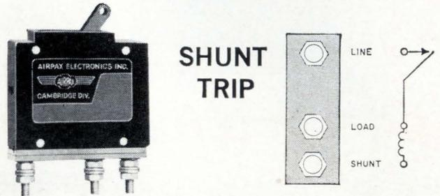
Shunt trip provides you with several possibilities. You can program an external shunt across the coil to change trip level for different operating modes of your equipment.
