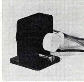
Reflex klystron oscillators series EM-1149 are useful as pump tubes for parametric amplifiers. The 5,000-hr warranty tubes, operating from 12 to 18 Ghz, are available in 2 versions. One offers an output of 1 w over a 500-Mhz tuning range; the other, 1.5 w over a 100-Mhz range. The 7-oz tube mounts in any position. Varian Associates, 611 Hansen Way, Palo Alto, Calif. [403]
