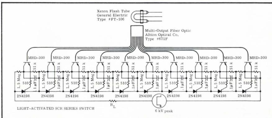
MRD300 combined with 2N4198 ELF® SCR (600 V) gives total  $t_{\text{on}}$  of 300 ns. Single light source coupled by multiple-output fiber optic bundle transmits light to photo transistors. Fast  $t_{\text{on}}$  is accompanied by gate isolation advantage.
