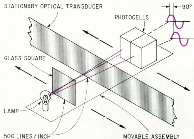
**Optical transducers.** A variable amount of light passed through a grating of opaque lines impinges on photocells to produce approximately sinusoidal signals spaced 90 electrical degrees apart.
