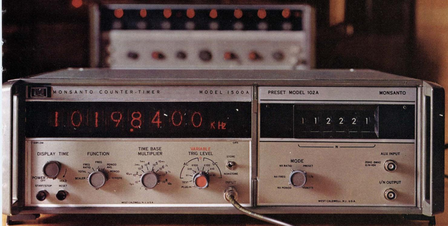
AVAILABLE PLUG-INS: TWO FREQUENCY CONVERTERS (50 MHz TO 500 MHz; 100 MHz TO 3 GHz); PRESCALER (dc TO 1 GHz); PRESET UNIT (20 Hz TO BEYOND 10 MHz); VIDEO AMPLIFIER (1 mV SENSITIVITY, 10 Hz TO 200 MHz); TIME INTERVAL UNIT (100 ns RESOLUTION); NON-COMMITTED PLUG-IN.
