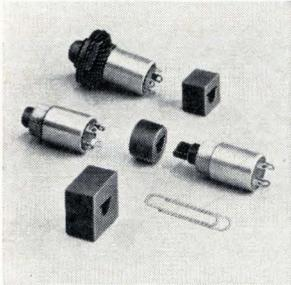
Designed for fast computer circuits, switches are moisture-proof and have less than 1  $\mu$ s contact bounce after transfer. B5200 and BW5200 series are rated at 3 amps resistive, 1 amp inductive, and 1 amp lamp-load at 28 v dc or 120v a-c. They are available in 3 circuit arrangements with 18 mounting styles. Controls Co. of America, 1420 Delmar Drive, Folcroft, Penn. [341]
