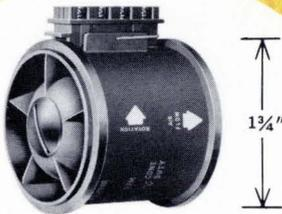
**VANEAXIAL FANS** — Rotron-pioneered Axi-max® fans feature time-tested reliability in severe environments. These tiny fans cool tightly packed airborne and ground-based electronics equipment with minimum size and weight: • 22-157 cfm (400 Hz) • 1 3/4" to 3" diameter • MIL-E-5272C qualification • 4-14 oz. weight • 1 1/4" to 3" wg static pressure. Diameters from 1 3/4" to 3".
