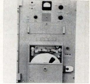
Ten-channel monitoring-recorder system PI-8010 meets MIL-E-16400 and will operate for 24 hours on a 10½-in. reel of ¼-in.-wide tape. Audible monitoring of any recorded channel is achieved by switch selection. Bandwidth capability is 2.7 khz; a cueing system has forward and rewind modes. Precision Instrument Co., 3170 Porter Dr., Palo Alto, Calif. [384]
