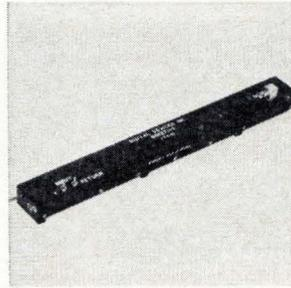
An ultralinear variable magnetostrictive delay line provides continuously variable delays from 2 to 35  $\mu$ sec at frequencies up to 2 Mhz. Unit operates in temperatures from  $-40^\circ$  to  $85^\circ\text{C}$  and survives shocks of 600 g. Delay is varied by a shaft; normal performance is 167 ns/turn with linearity to better than 0.25%. Digital Devices Inc., 200 Michael Dr., Syosset, N.Y. [351]
