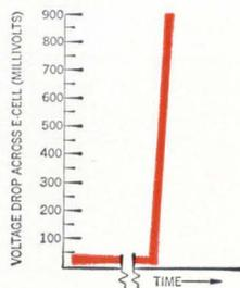
\* The Bissett-Berman E-CELL™ is a unique "liquid state" electrochemical timing and integrating component now being manufactured in high volume on fully automatic production lines. E-CELLs are designed for single or repetitive use in generating time delays ranging from seconds to months, or integrating events from one to infinity, and consume only nanowatts. Patents applied for.
