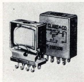
Military relay type PF has contact ratings up to 10 amps, with operate and release time of 7 msec max. Initial circuit resistance is 10 milliohms max., 20 milliohms max. after more than 100,000 operations at 10 amps, 28 v d-c. Unit operates from  $-65^\circ$  to  $+125^\circ\text{C}$ , withstands vibration of 20 g at 10 to 2,000 cps. C.P. Clare & Co., 3101 Pratt Blvd., Chicago. [353]
