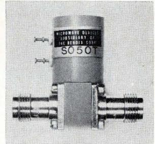
Shutter switch model S050T operates from 2.4 to 11 Ghz with a vswr of less than 1.30. Insertion loss is under 0.4 db, and isolation exceeds 30 db in the normally open position at 11 Ghz. Switching time is 0.01 sec, operating life greater than 100,000 cycles. The switch weighs 3 oz, is  $1\frac{5}{8} \times \frac{3}{4} \times 1\frac{1}{8}$  in. Bendix Microwave Devices Inc., Farmington, Conn. 06032. [408]
