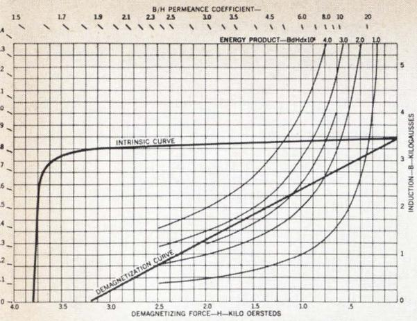
With a coercive force of 3200 oersteds, Indox 7 has a higher resistance to demagnetization than any commercially available magnetic material except costly platinum-cobalt. It also has a high peak energy product and high intrinsic coercive force.
