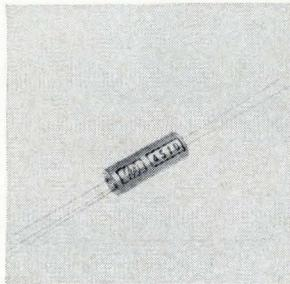
Photocontrolled resistor type 5082-4510 uses a cadmium-sulfoselenide photocell for stability in a changing temperature environment. Photocell resistance, when illuminated, changes typically by a factor of 1.5 with a variation in temperature from 25° to 65°C. Units cost \$8 each in small quantities, and \$6.80 for 10 to 99. Hewlett-Packard Co., 1501 Page Mill Rd., Palo Alto, Calif. [438]
