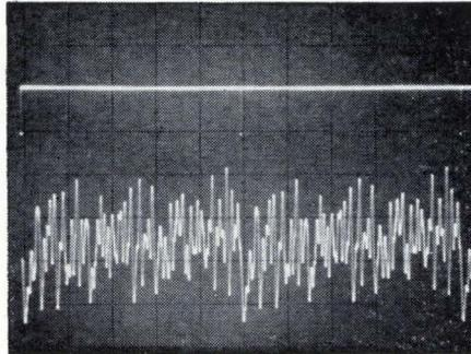
The Hewlett-Packard 3722A Noise Generator now lets you harness noise so that it becomes a defined and calibrated input to your system. It allows you to synthesize and reproduce at will noise signals of constant noise power with a probability density function (pdf) in the classical Gaussian construction. This unique new instrument uses computer techniques to synthesize noise patterns of selectable length that are thoroughly defined and repeatable.
