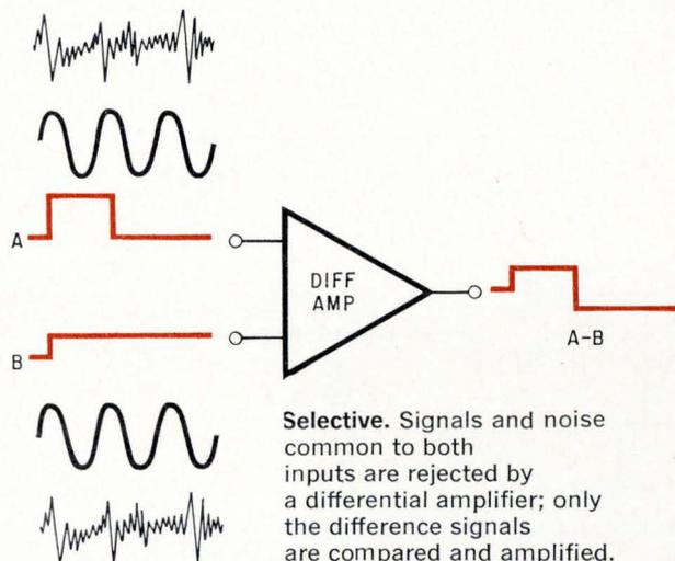
**Selective.** Signals and noise common to both inputs are rejected by a differential amplifier; only the difference signals are compared and amplified.
