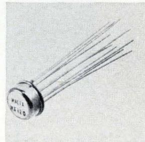
Hybrid IC, d-c wideband amplifier HX610 is offered in a 10-lead TO-5 can. It has built in by-pass capacitors and needs no external components when used as an amplifier with a voltage gain of 26 db. Maximum output voltage swing with no load is 20 v peak-to-peak at 100 Mhz, derating to 2.5 v p-p at 100 Mhz. Hallex Inc., 139 Maryland St., El Segundo, Calif. [443]
