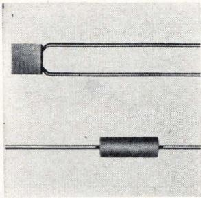
Series TT ceramic capacitors in encapsulated radial and axial configurations, have tolerances of  $\pm 0.25\%$ ,  $\pm 0.5\%$ , and  $1\%$ ; and a capacitance range from 1 pf to 200,000 pf as standard. Applications include delay lines, a-d conversion, precision filtering, timing circuits, and ratio matching. Electro Materials Corp., 11620 Sorrento Valley Rd., San Diego, Calif. 92121. [349]
