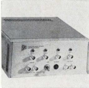
Analog multipliers 610T(A) and 610T are for use in high-speed data-reduction systems. The 610T(A) accepts 2 signals in the range of 0 to  $\pm 5$  v and its output is 1/5th the algebraic product; the 610T accepts signals of 0 to  $\pm 10$  v and its output is 1/10th the algebraic product. Bandwidth is 500 khz minimum. GPS Instrument Co., 188 Needham St., Newton, Mass. [386]
