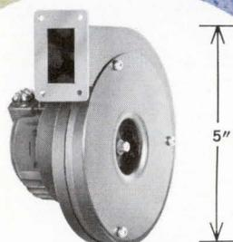
**RADIAL WHEEL BLOWERS** — These blowers meet specialized cooling and air sampling requirements demanding higher pressure and lower flows than conventional squirrel-cage blowers: • 13-39 cfm • Working static pressures to 5" wg • 50/60 Hz and 400 Hz, single or three phase • MIL spec • High altitude Altivar® motors available. • Long-life ball bearing induction motors.
