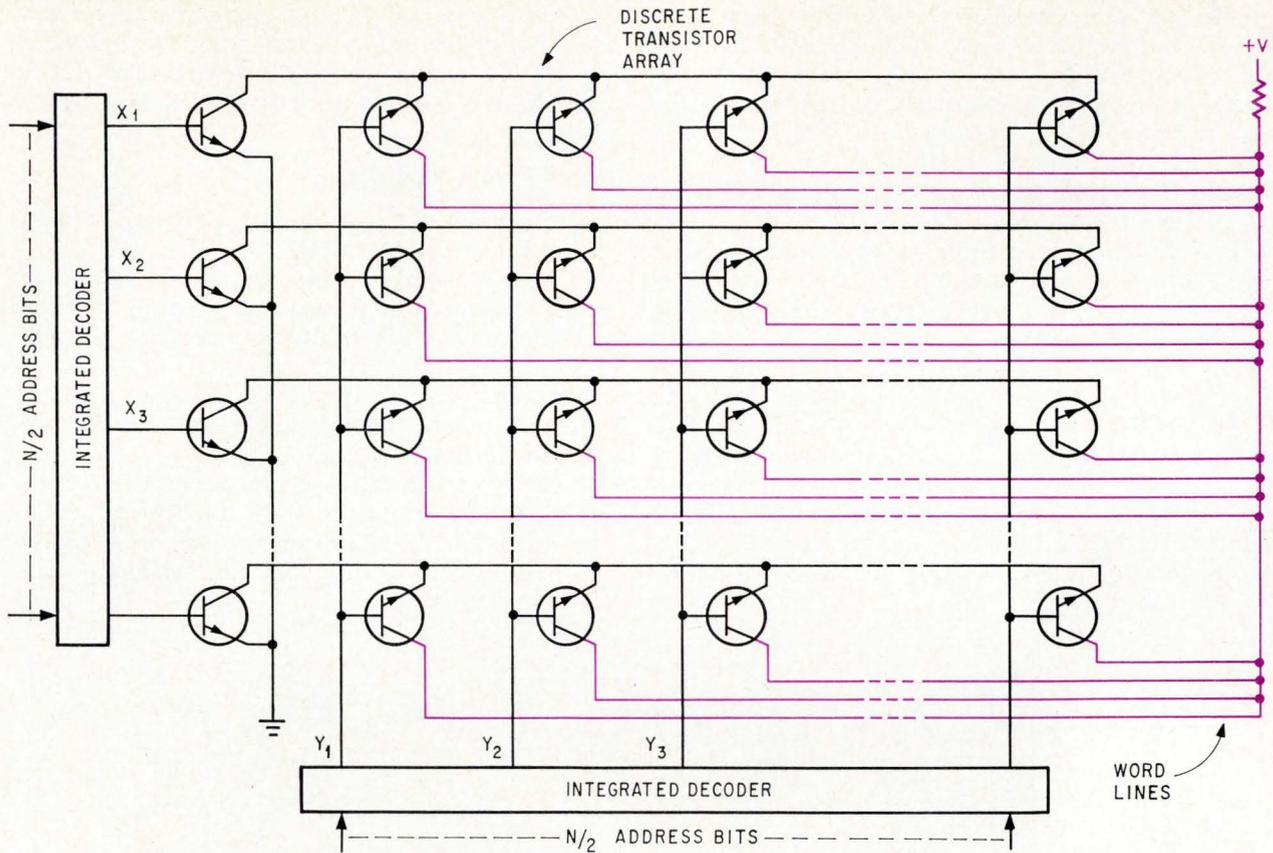
**Common connection.** A positive signal at  $X_1$  forward-biases the first current-sink transistor. This provides a ground connection for the top row of transistor AND gates. A positive signal at  $Y_1$  permits current to pass through only the first gate. Thus line 1 is selected. The word lines are in color.
