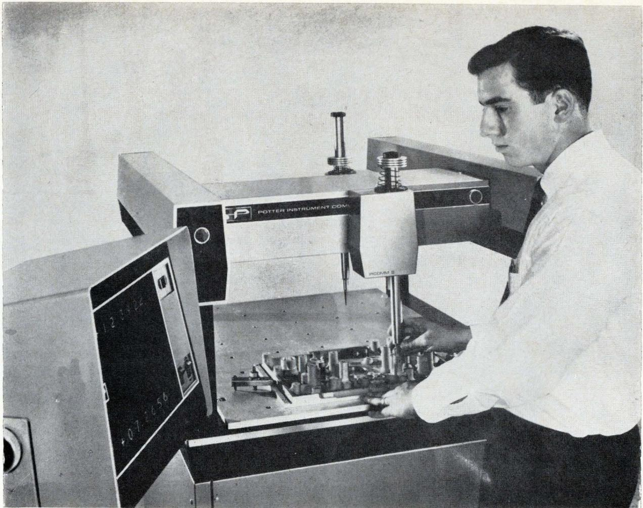
**Measuring the part.** Probe is placed into machined hole on tape transport panel and its position is automatically displayed on digital readout.
