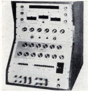
Guidline 9930 d-c current comparator potentiometer features a 7-figure readout without critical resistors. Linearity is 0.05 ppm over full range, and long term drift less than 0.1 ppm per year. The unit's resolution is only 1 part in  $2 \times 10^7$  of full scale, and standard cell dial resolution is 0.1 ppm. Cost is \$7,890. Hallmark Standards Inc., 145 Library Lane, Mamaroneck, N.Y. [361]
