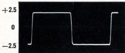
SIMULTANEOUS SINE AND SQUARE-WAVE outputs pack real power (up to  $\frac{1}{2}$  watt into 50 ohms). Photos show open circuit output voltages at 1 MHz.
