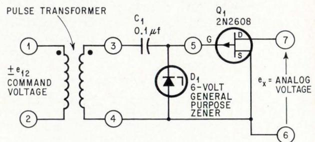
**Switching action.** Voltage at point 5 is either 6 or zero volts, turning  $Q_1$  off or on, respectively.
