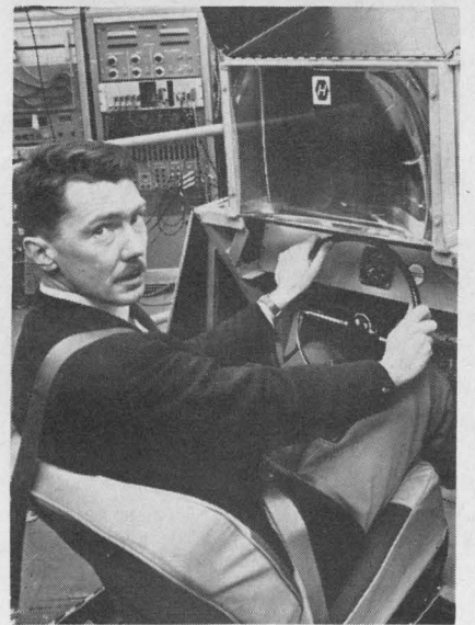
Long look. Driver, seated before a collimating lens, sees unending line of "fence posts" stretching outward to infinity.
