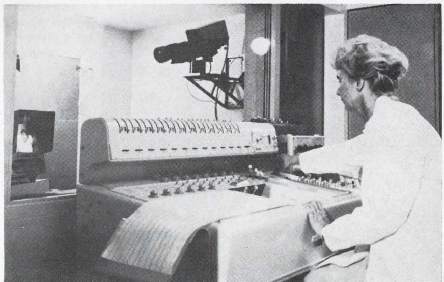
Together. Synchronized system displays picture of electroencephalogram curves alongside that of patient, enabling an attendant to tell immediately if wave variation is significant.
