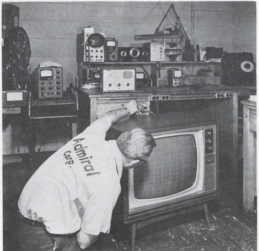
Black art. Factory serviceman makes so-called pincushion correction on a color set to assure the proper vertical and horizontal linearity; few technicians bother with this key adjustment during the initial setup.
