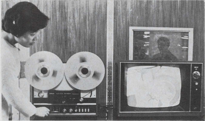
Priced right. Akai fixed-head video tape recorder will go on U.S. market in December at list price of about $300. Receiver-monitor adds $150 to the price. The recorder uses 1/4-inch tape.
