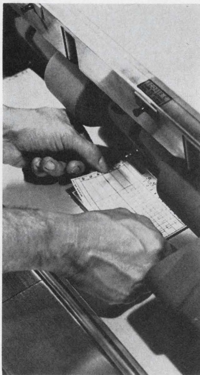
Strike. Bowler inserts scorecard into Brunswick’s computerized automatic scorer, which tallies, prints, and then projects score on a screen.
