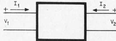
Two-port network. Parameters V_1 , I_1 , V_2 , and I_2 represent the input and output voltage and current of the network.
