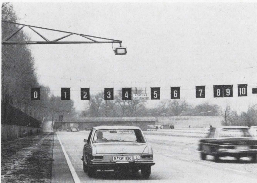
Checkpoint. Doppler radars measure speed and braking distance at highly instrumented Daimler-Benz test track at Stuttgart-Unterturkheim.
