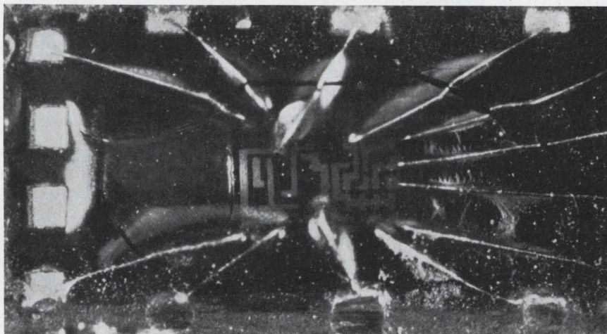
Fracture. Stress caused by shrinkage is serious enough to snap the interconnection wires on this plastic-packaged IC. Note the crack (dark oval) around the package.
