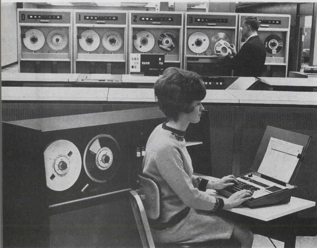
Quick trick. With Honeywell's Keytape, data can be transcribed directly onto computer-ready magnetic tape through a keyboard.
