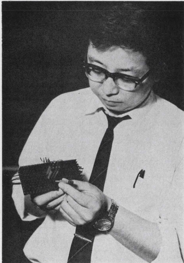
Plug-ins. Lamps are inserted in blocks for final assembly. However, since lamp ratings are different, red, green and blue lamps are not interchangeable.
