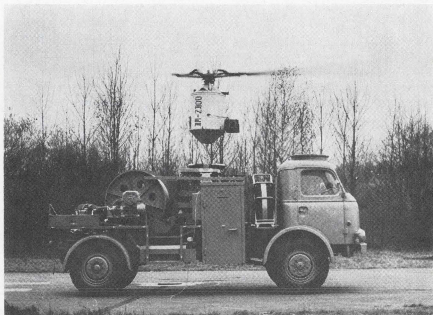
Ready to rise. West German kibitzing capsule for electronic gear rides its carrier to launching point.
