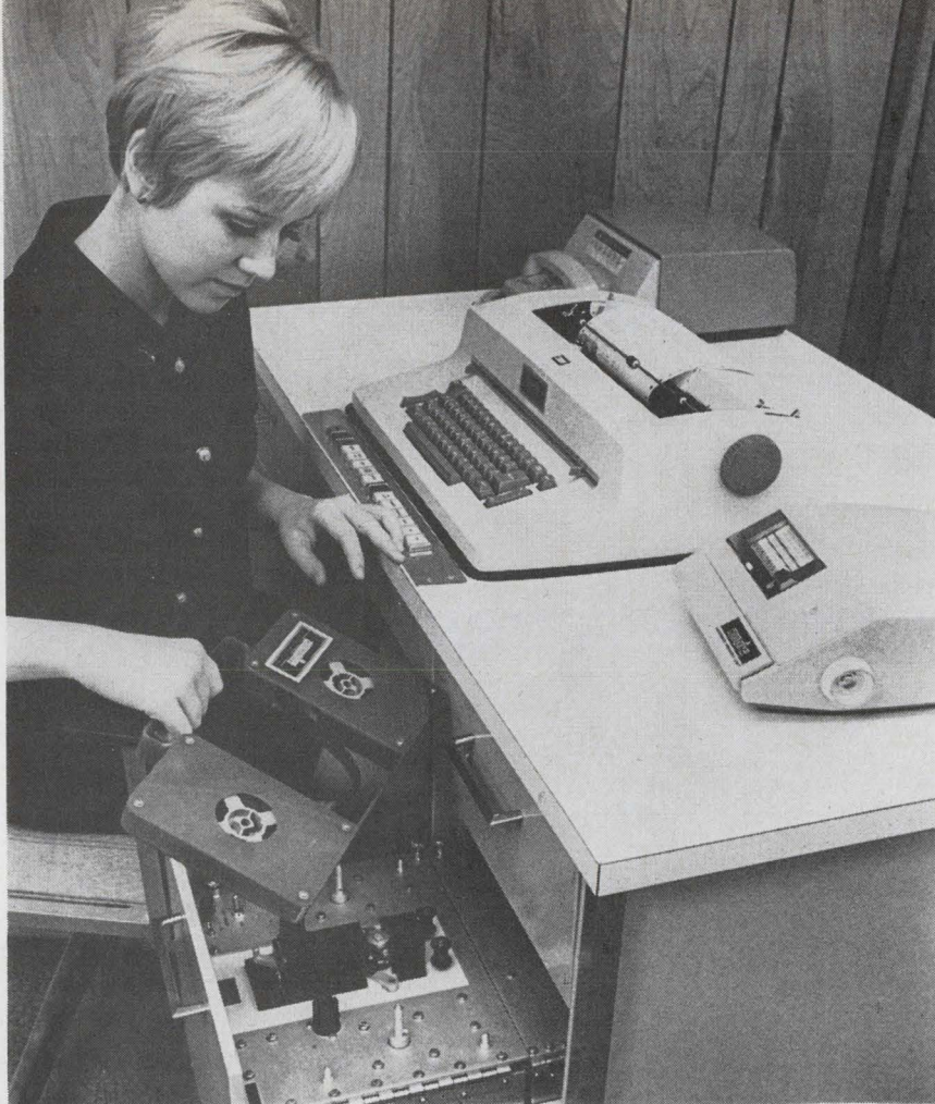
In and out. The removable magnetic tape cartridge in Communitytype's data communication system has capacity of 180,000 characters or 30,000 words.
