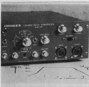
Variable delay pulse generators series 2306 feature bipolar outputs to 50 v, and less than 1 nsec rise and fall time. Repetition rates for all models are variable by front panel control from 1 hz to 1 Mhz, or may be externally triggered to 1 Mhz. Overshoot and undershoot is less than 5% for amplitudes over 2 v. Gralex Industries Inc., 28 Di Tomas Ct., Copiague, N.Y. [361]
