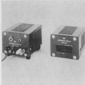
Dual output power supply NPS-300 features separate positive and negative power outputs. Each output is adjustable to between 12 and 18 v d-c at any load between 0 and 30 ma each. Low ripple and noise with fast response time allows unrestricted use in sensitive circuitry. Regulation is to  $\pm 0.05\%$  for load and line. Philbrick/Nexus Research, Dedham, Mass. [386]
