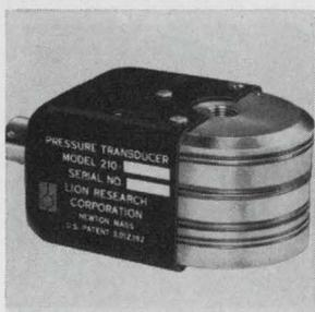
Dual-range pressure transducers series 200M feature a linearity of better than 1% of full scale. The primary range is the highest pressure range to be measured (0.05 to  $\pm 5$  psi); the secondary range is obtained by an internal amplifier and can be as much as 10 times lower, or typically 0.005 psi full scale. Lion Research Corp., 60 Bridge St., Newton, Mass. [366]
