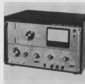
Modulation meter model 409 provides wide carrier ranges—a-m: 3 to 1,200 Mhz; f-m: 3 to 1,500 Mhz—and measures percentages of amplitude modulation in 3 ranges, and f-m deviation up to  $\pm 600$  khz in 6 ranges. A-m measurement accuracy is better than  $\pm 3\%$  to 5 khz; f-m, better than  $\pm 5\%$  to 50 khz. Winslow Tele-ronics Inc., 1005 First Ave., Asbury Park, N.J. 07712. [364]
