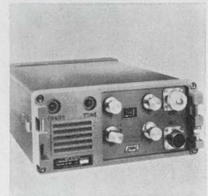
Ten-watt portable single-sideband radiotelephone and radiotelegraph unit operates up to two independent and two dependent channels in the 1.6 to 15 Mhz range. It can be powered by "D" batteries, alkaline cells, or nickel-cadmium batteries which may be recharged from a 12-volt auto electrical system. Kaar Electronics Corp., 1203 W. St. Georges Ave., Linden, N.J. 07036 [428]
