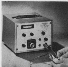
Go/no-go noise limit tester 60-2300 can be used to inspect precision or trimmer, wirewound or film potentiometers. The unit contains a constant current source to energize the wiper and a high input impedance adjustable limit detector to monitor wiper voltage. A panel light indicates when a preset limit is exceeded. Solatron Enterprises, Venice, Calif. [363]
