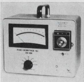
Lightweight vibration monitor model VM-10M can be used with any piezoelectric accelerometer with sensitivities from 1 mv/g to 100 mv/g. Features include high input impedance of 1,000 megohms, 6 full-scale acceleration ranges of 1, 3, 10, 30, 100 and 300 g, and a constant 10 mv/g output. Price is \$395. Agac-Deritron Inc., P.O. Box 358, Alexandria, Va. 22313. [365]
