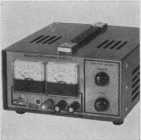
Variable voltage bench supply model BP-118 has an output of 0 to 34 v at 1.5 amps. Regulation is mv or 0.01% with ripple a low 250  $\mu$ v. Voltage and current output are continuously monitored by two taut-band meters. The unit meets MIL Specs and is completely short-circuit proof. Price is \$118. Power/Mate Corp., 163 Clay St., Hackensack, N.J. 07601. [385]
