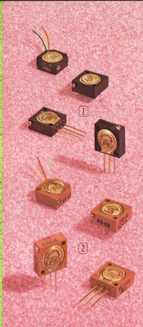
1. **SERIES 255.** RJ-22 styles with infinite resolution.  $\pm 5$ , 10, 20% tolerances to meet all your needs. ¼ watt @ 70°C. 100 $\Omega$  to 1 meg.
