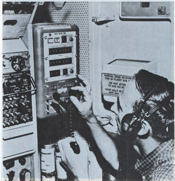
Less talk, more action. Prototype digital communications systems like this Bendix equipment flying on Pan American aircraft transmit routine flight and engine-performance data to crt displays or teletypewriters, cutting voice traffic.
