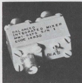
Integrated mixer model MWT-9375 employs three-arm branch hybrid design that saves weight and space. The device operates at a center frequency of 9,375 Mhz with a 10% bandwidth. Input vswr is 1.50 to 1 maximum and input to local-oscillator isolation is 15 db. Maximum noise figure is 7.5 db with a 1.5 db i-f. Raytheon Co., 152 Floral Ave., Murray Hill, N.J. 07974. [402]
