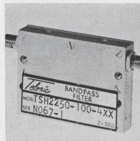
Miniature bandpass filter model TSH is for telemetry applications in the 2.2 to 2.3 GHz transmission band. It exhibits a wide stop band with rejection greater than 40 db from d-c to 1.980 GHz and 2.475 to 8 GHz. Rejection skirts are typically similar to 0.1 db Chebyshev ripple. The unit measures 1 21/32 x 1 5/32 x 5/16 in. Telonic Engineering Co., Box 277, Laguna Beach, Calif. [407]
