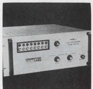
Analog-to-digital converter model HS-810 will assign up to 10 million 8-bit binary numbers/sec to wideband analog signal. Codes available are straight or offset binary, 1's or 2's complement, or Gray. It has a maximum error of 0.2% ±½ least significant bit and a maximum aperture time of 0.4 nsec. Computer Labs, 1109 Valley Park Dr., Greensboro, N.C. 27403. [428]
