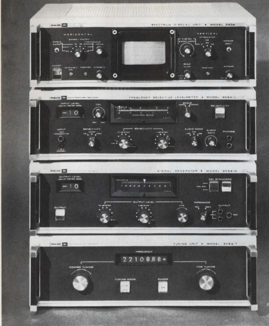
Three 4-kHz channels of L3 carrier multiplex system. Center channel has teletype subcarriers. Model 360A is in 12-kHz sweep width mode, sweeping from 6.780 to 6.792 MHz.
