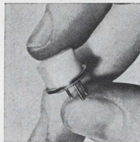
Rapid installation T0-5 and T0-18 Teflon transistor sockets eliminate chassis hole chamfering and loose parts. Called Beltline, the sockets use a belt or band of metal around the outside diameter. Moderate pressure forces the socket through the belt and chassis hole, and the Teflon expands to lock the socket in place. U.S. Terminals Inc., 7502 Camargo Rd., Cincinnati [343]
