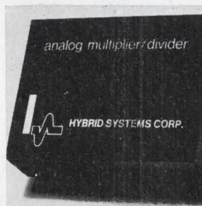
Analog multipliers models 103 and 104 offer full scale accuracy better than 0.1% for full 4 quadrant operation. The transfer function of the 103 is +XY/10, whereas the 104 is -XY/10. Both units may be used to multiply, divide, square, and square root by appropriate pin interconnections. Price (1-9) is $325. Hybrid Systems Corp., 95 Terrace Hall Ave., Burlington, Mass. [386]
