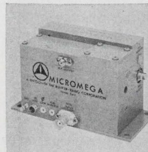
Phase-locked microwave source offers low-noise performance at selected bands from 3.6 to 14.3 Ghz. Key specifications include: harmonic rejection, greater than 60 db in-band, greater than 50 db out-of-band; frequency stability, to \pm 5 ppm; output power, 10 or 50 mw minimum; f-m response, 25 khz to greater than 10 Mhz. Micromega, 4134 Del Rey Ave., Venice, Calif. [405]
