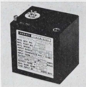
Static inverter model N2D converts 28 v d-c to 400 hz sine wave voltages of either 115 or 26 v a-c. With continuous full load operation at 160° F, it supplies an output power of 20 v-a. Modular design provides a package as small as 2½ x 3 x 3¼ in. which weighs less than 2.1 lbs. Price is $218. Abbott Transistor Laboratories Inc., 5200 W. Jefferson Blvd., Los Angeles 90016 [381]
