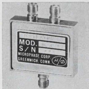
Y-function circulators series 5000 are manufactured using the latest thin-film techniques. They cover the range from 1 to 12.4 Ghz in 10% bandwidths. Isolation is 20 db minimum, insertion loss 0.5 db maximum, and vswr is low. Units are 1.50 x 1.25 x 0.50 in. and weigh less than 1.5 oz. Prices (1-5) are from $200 to $250 each. Microphase Corp., 35 River Road, Cos Cob, Conn. [401]
