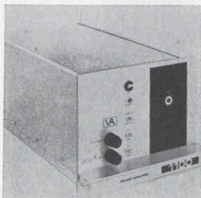
Power amplifier series 1100J is a fully-professional plug-in unit designed for the most exacting control room and sound reinforcement applications. It is equipped with input transformer and pre-amplifier. Output is conservatively rated at 75 w rms at less than 0.5% harmonic generation. United Recording Electronics Industries, 11922 Valerio St., N. Hollywood, Calif. 91605. [385]
