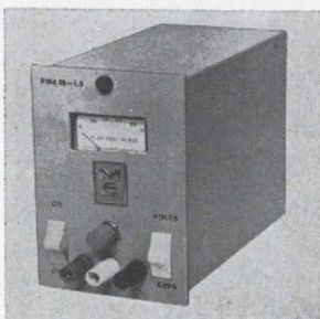
Miniature silicon power supplies series PMA feature self-restoring overload or short circuit protection by a solid state, cutback, current-limiting circuit. Standard units have outputs from 10 v/1.5 amp to 100 v/0.2 amp. Load regulation is 0.02%; line regulation, 0.01%; ripple, less than 1 mv rms. Mid-Eastern Industries, 660 Jerusalem Road, Scotch Plains, N.J. 07076 [387]
