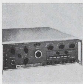
Servo system analyzer model 1999 is for analysis and test of servo-mechanisms and complex control systems by observing phase and amplitude response with respect to various frequencies and wave shapes. Harmonic distortion is less than 0.5%. Phase accuracy is \pm 1^\circ from 0 to 360°. Frequency accuracy is \pm 1\% . Servo Corp. of America, 111 New South Rd., Hicksville, N.Y. [362]
