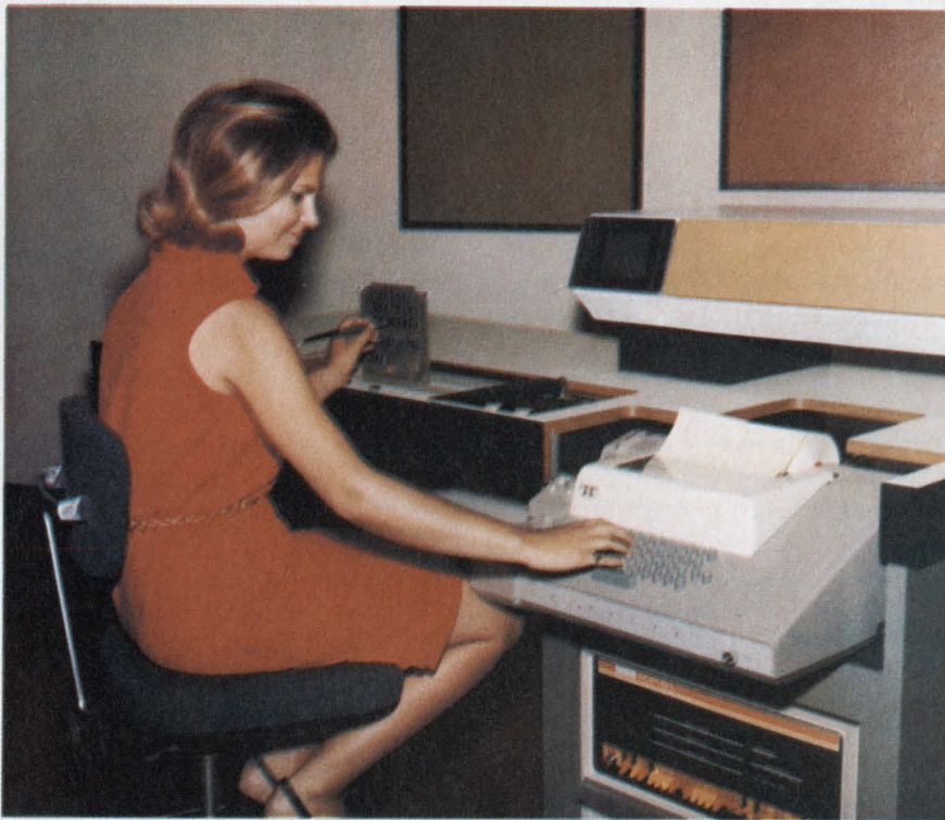
Test station. Logic module analyzer system includes computer (lower right), alphanumeric display, and teletypewriter printout.
