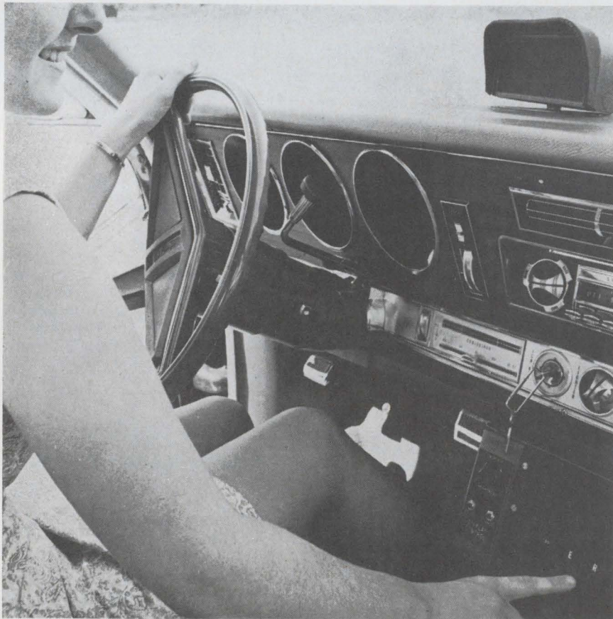
Helping hand. GM-developed elements for electronic route-guidance system include encoder with wheels for dialing destination and dashboard display.
