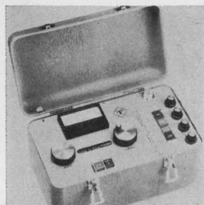
Manual balance digital indicator MDX-11 is used with bonded strain gage force and pressure transducers with 2 mv/v or 3 mv/v output signals. Full scale output is 100,000 counts with a 30% overrange capability. A course control knob of 12 additional steps of 10,000 counts each is included. Accuracy is 0.05%. Transducers Inc., E. Rivera Rd., Santa Fe Springs, Calif. [366]
