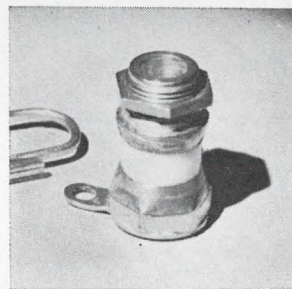
Alumina insulated bushing assembly AB1 provides electrical isolation for variable air dielectric trimmer capacitors mounted on conductive chassis or other surfaces. It has a resistance rating of 10 9 megohms, and can be used with any standard air trimmer with a 15/64 in.-64 threaded bushing. Price in lots of 100 is $2 each. Voltronics Corp., West St., Hanover, N.J. [343]
