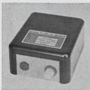
Line-operated, regulated, h-v power supplies series ARA-106 have an output from 4 kv to 18 kv. Ripple is less than 0.1%. They are designed for use with crt's, image pickup, display and phototubes, and as a general-purpose high voltage source. Operating temperature is -20^{\circ} to 75^{\circ} C. Advanced High Voltage Co., 8635 Yolanda Ave., Northridge, Calif. [381]
