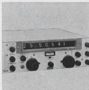
H-f receiver model RA6218 features an electronic counter with a 7-digit display, locked to a built-in high stability crystal frequency source, enabling the operator to read the receiver tuned frequency to within 10 hz. Frequency range is 1 to 30 Mhz. The unit measures 5\frac{1}{4} x 19 x 17 \frac{1}{2} in. Racal Communications Inc., 8440 Second Ave., Silver Spring, Md. [387]
