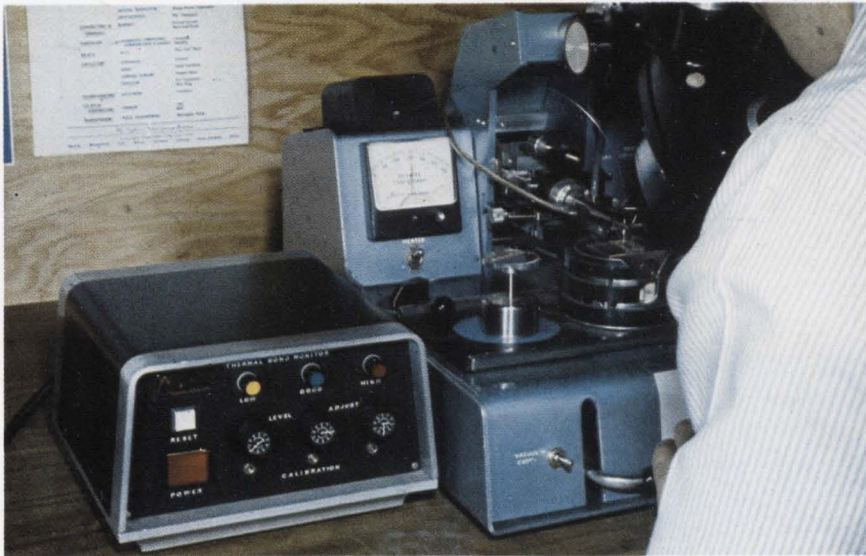
Beacon. Lights on the control console indicate which of three levels of temperature has been reached. Each threshold detector can be set to respond at temperatures ranging from 200°C to 1,000°C.
