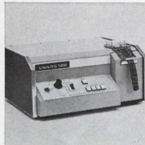
Digital data recording system Unilog 100 offers a programmer, code converter and paper tape perforator complete in one package. All control functions and the word format are arranged by simply jumper-wiring the output connector. Data can be in decimal or BCD form represented by either contact closures or voltage levels. Eldon Associates Inc., Industrial Ave., Palo Alto, Calif. [426]
