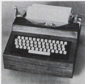
Input/output device for computers called Teletype, measuring 13 x 18 x 7 in., and weighing 25 lbs, is interchangeable with the KSR33 Teletype. The printer input and keyboard output is serial 8 bit ASCII code. The Teletype operates at a speed of 10 operations/sec (100 wpm). Electronic Information Systems Inc., Rural Route 3, Boulder, Colo. 80302 [425]
