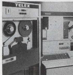
Multiformat read-only tape drives 4853 and 4863 are available with 1600 characters per inch capability for computer output microfilm systems. The 4853 offers a 75 inch per second tape speed and a maximum transfer rate of 120 kilobytes. The 4863 is faster at 112.5 inch per sec with a maximum transfer rate of 180 kilobytes. Telex Computer Products Division, Tulsa, Okla. [4071]
