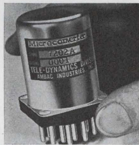
Microconverter 7202A accepts computer levels and converts them to drive commercial communications equipment. The compact unit isolates input power and ground returns from the output by optically coupling input signals through a light-emitting diode and light-sensitive resistor. Price is under $100 in small lots. Tele-Dynamics, Virginia Dr., Ft. Washington, Pa. [4031]
