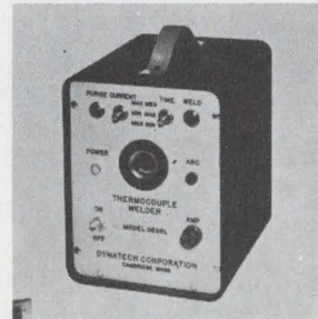
Thermocouple welder 116SRL welds wires from 55 to 20 Awg in any material, including copper, platinum, and others. A tungsten inert gas arc is energized to the specified temperature for the correct length of time by the power supply unit which incorporates 3 position switches for weld time and weld current. Dynatech Corp., 17 Tudor St., Cambridge, Mass. [427]
