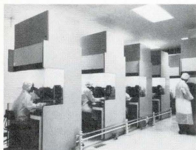
SUPER-CLEAN AIR . . . In vertical laminar-flow hoods designed to provide additional air filtering, wafer photo resist is exposed to ultraviolet light after precise mask alignment.
