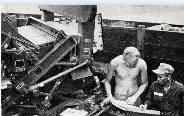
8. Losing its cool. U.S. and Vietnamese technicians ponder antenna and circuits of AN/MPQ-4, frequent victim of the hot season.
