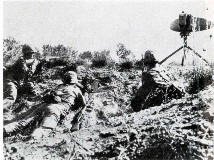
6. On guard. An AN/PPS-5 doing its thing for the infantry. The lightweight radar can spot a walking man at 5,000 meters.
