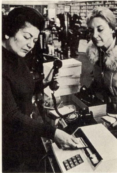
Cash call. IBM's credit authorization terminal uses acoustic coupler attached to telephone's mouthpiece.
