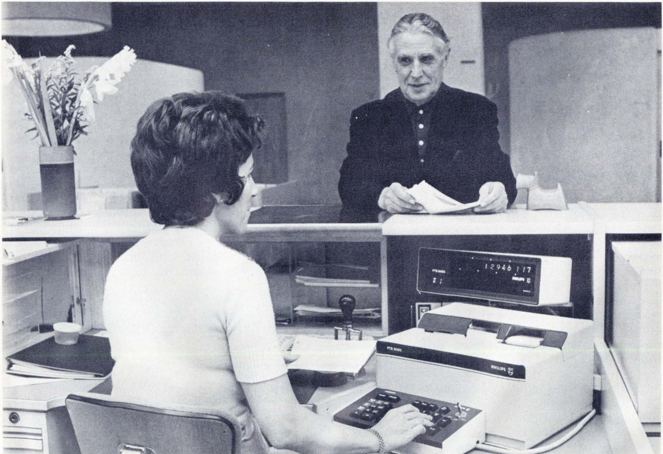
First of its kind. Cashier terminal in Svenska Handelsbanken's on-line teller system is initial installation in what will be a $12 million system. Transactions are registered and displayed and account information can be called from local, regional, and central files.
