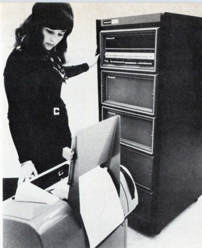
6. Honeywell System 700. Central processor has a 78-instruction repertoire, a real-time clock, and other features. Its high performance is due in part to its use of a read-only-memory overlay.
