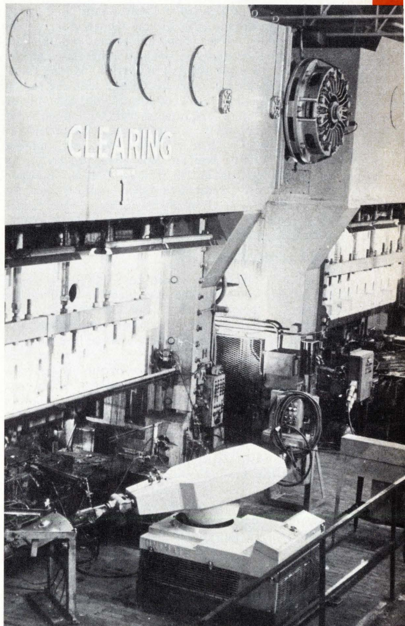
Safety first. Unimate robot feeds parts from a conveyor belt into dies of 2,000-ton stamping press, a hazardous job for a human operator.
