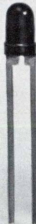
CM4-48 GaAsP, small package similar to T-1, heavy duty leads for wire wrapped terminals.
