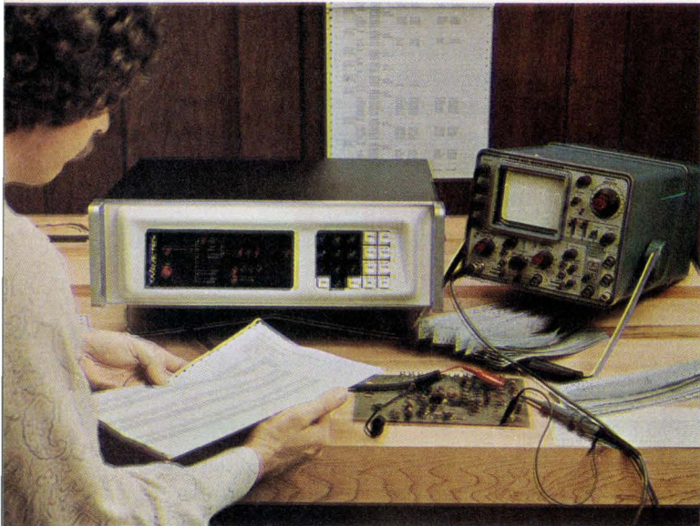
Programmable. Wavetek's model 152 function generator can be programmed by a remote data bus, making it a natural for automated test applications, or by the push buttons shown on the front panel.
