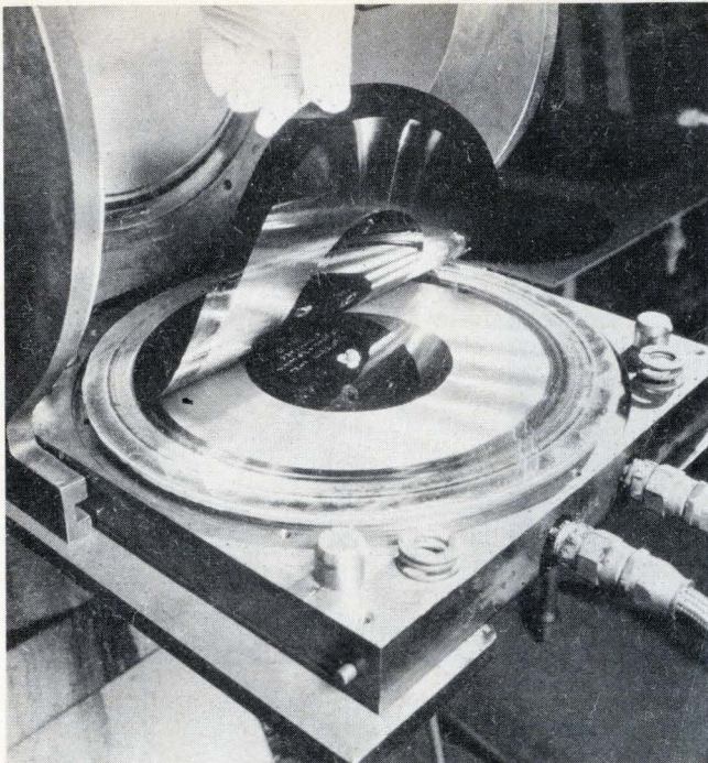
3. Floppy TV. Zenith's video disk comes off the press at the company's research lab for display on a laser-type optical player.
