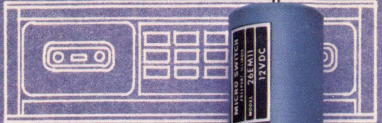
IDEALLY SUITED FOR DIGITAL CASSETTE RECORDERS AND CARTRIDGE DRIVES, THE 26 EM MOTOR USES A HOLLOW ROTOR TO PROVIDE THE LOWEST POSSIBLE ROTOR MASS, RESULTING IN VERY LOW INERTIA. DIRECTLY INTERCHANGEABLE WITH MOTORS MADE OUTSIDE USA.
