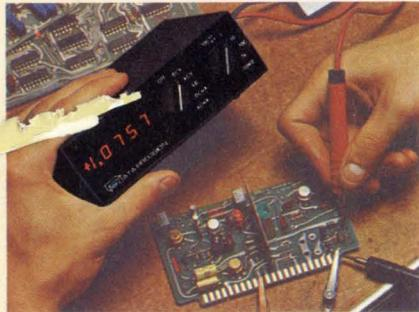
Measuring just 5½" x 1¾" x 3½", and weighing only 1.3 pounds, our 248 is the only rechargeable portable 4½-digit DMM that brings you the advantage of True RMS voltage measurements from 10 microvolts to 500V and current from 10 nanoAmps to 2A. With a maximum crest factor of 5 at nominal range input and 2½ at the 100% over-
