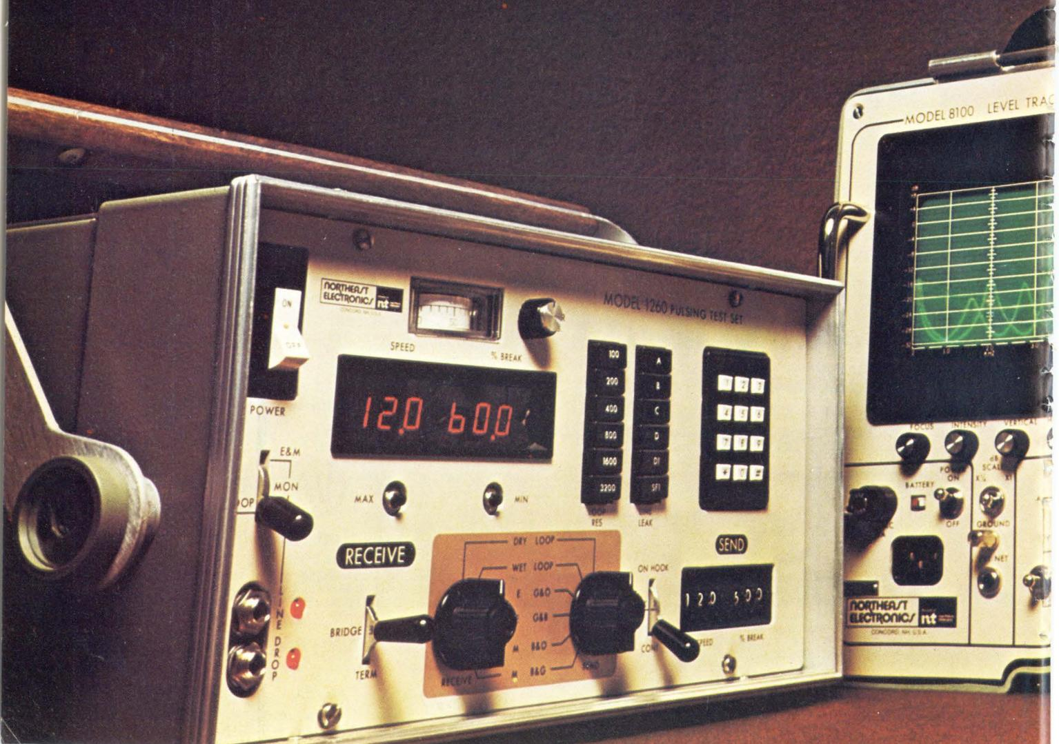
rate instrument ( $\pm 0.1$  pps,  $\pm 0.5\%$  on percent break), TTS 1260 has a convenient digital readout and is built to withstand rugged use. It's the instrument you need for extreme accuracy, low price plus the unbeatable combination of Northeast craftsmanship and reliability. Operates on 48V central office battery. "A" relay included. Price: \$1950.
