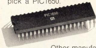
The PIC 1650 is the first "real" Programmable Intelligent Computer on a single chip.
