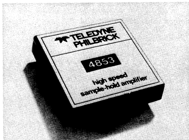
6. Fast and accurate. Philbrick's 4853 is suitable for use with 12-bit converters at speeds up to 20 kHz. Input voltage range is \pm 10 V, input impedance is 2 k \Omega , and aperture time uncertainty is \pm 1 ns.
