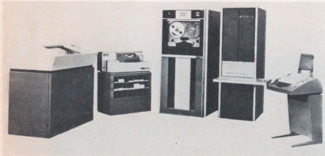
THE FIRST COMMERCIALY AVAILABLE MINI. The PDP-5 was introduced in September, 1963. It was the first 12-bit mini (the PDP-8 was a very similar mass-produced version). Selling price was about $25,000.
