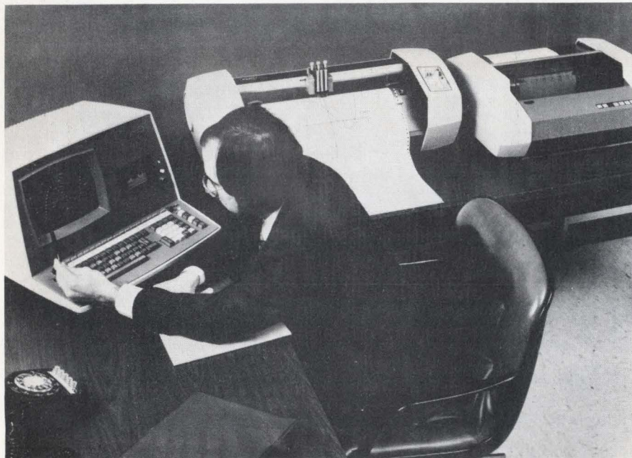
THE 5100 ALTERNATIVE. Wang's 2200 PCS can be combined with the company's new micro-based drum plotter or 120-cps matrix printer.
