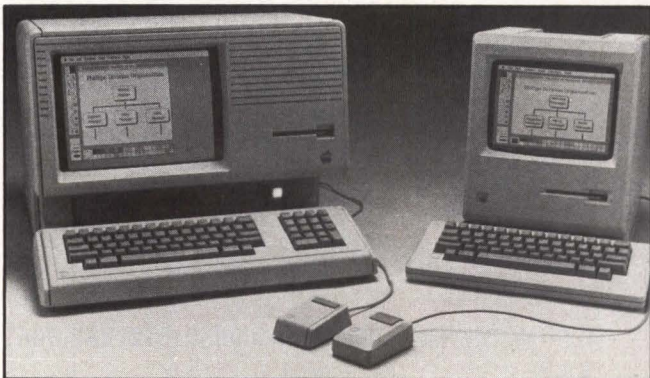
Apple's Lisa and Macintosh computers sport high-resolution graphics, interactive mouse interfaces and menu-driven operation.
