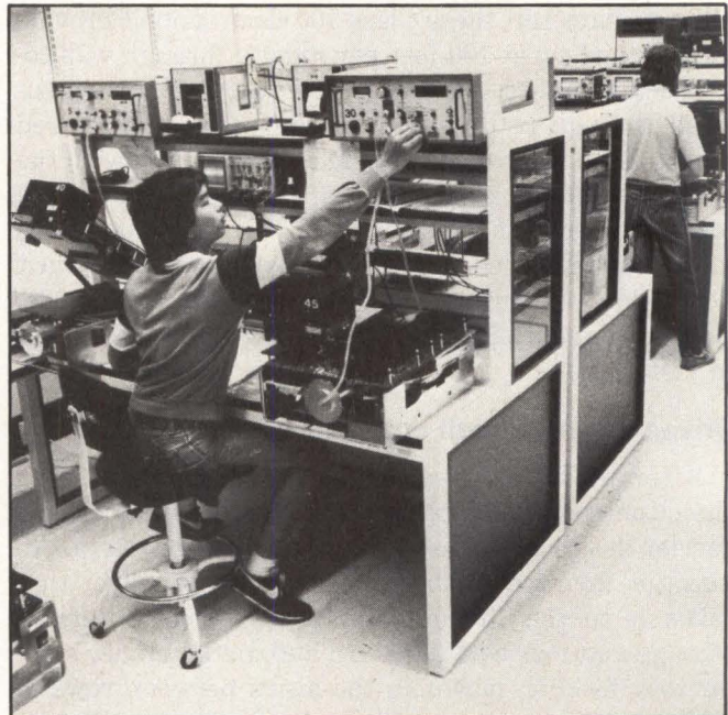
Workers perform contamination tests on the head/disk assembly before putting it into a frame with the printed-circuit board assembly and sending it into the automated test system for run-in and final testing.
