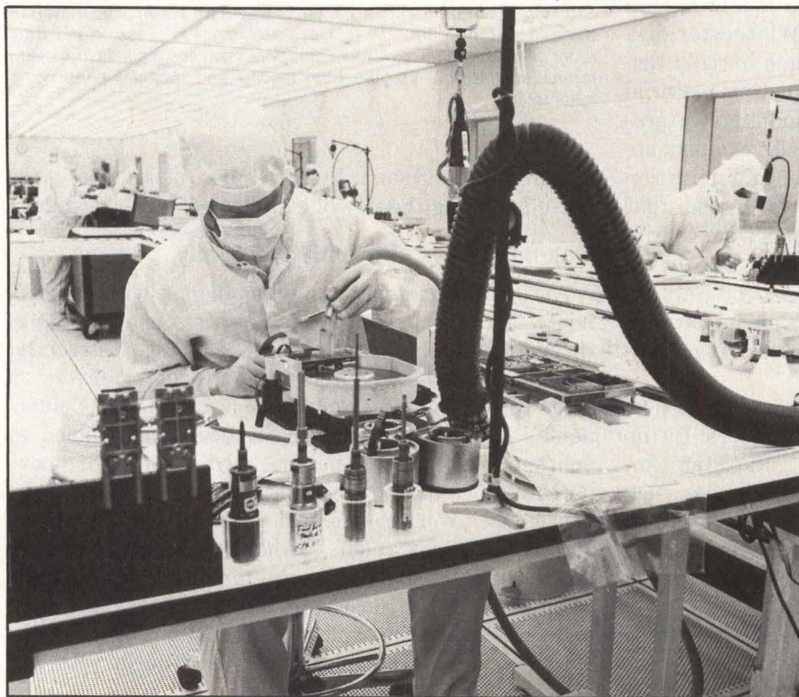
Inside the clean room, a worker completes a head/disk assembly. Delicate parts move from station to station on conveyors, minimizing accidental dropping and jarring.
