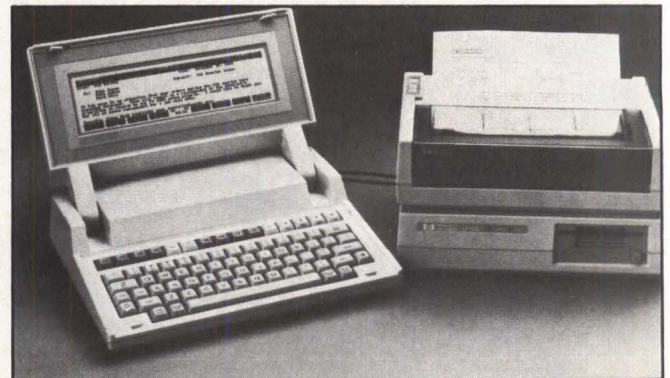
HP's Portable weighs 9 pounds, features a 16-line-by-80-character display, built-in application software like word-processing and spreadsheet programs, and terminal-emulation capabilities.
