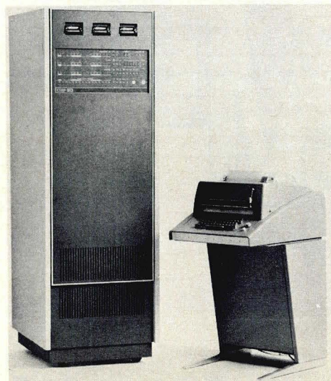
Fig. 1. The CSP-30, a new high-speed (100 ns full-cycle time) computer for signal processing applications, shown here with magnetic cassettes and KSR-35 I/O.
