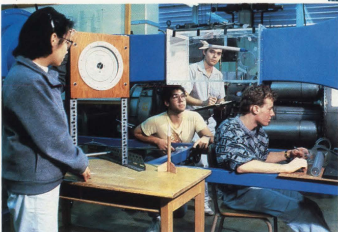
(Left) A subsonic wind tunnel (with model rocket) for tests up to 100 mph is available for Aeromechanical students.
