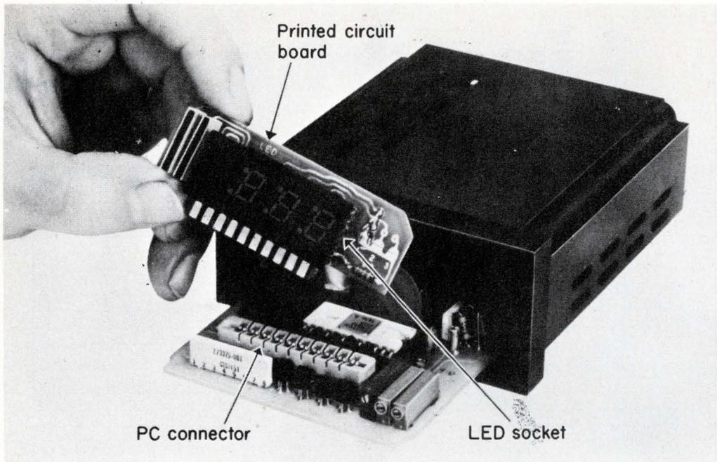
**A typical display application** is this 3 1/2-digit DPM. The LED displays are mounted on a vertical printed circuit board that is then plugged into the main board. To be realistic, the cost of the display must include the cost of this additional PC board, the PC connector, and the sockets for the individual displays.
