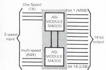
The block diagram shows two ASI modules which form a complete 14-bit 2-speed converter. No external mixing logic or programming is required. For further information contact astrosystems, inc.
