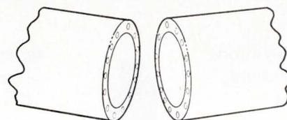
Sandia Labs, with the collaboration of Bendix Corp., developed this connector for a military application. Fourteen of these single-contact connectors, mounted around the ends of two 8-inch dia. cylinders, electrically interconnect the two cylinders and meet the following design requirements: Continuous operation for years at low dc voltage and current; contact resistance no higher than 30 m $\Omega$ ; plus stringent mating requirements.
