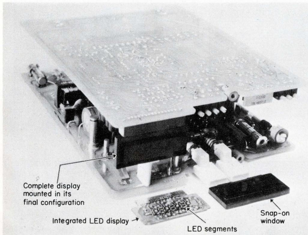
**One approach to reducing display costs**, used in this multimeter, integrates the actual LED segments and the mounting hardware. The display also includes a snap-on window which serves both as a protective cover during handling, and a viewing window after installation.
