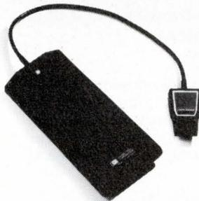
**10529A Logic Comparator** — This device steals stimulus from the circuit under test to exercise a reference IC of the same type. Outputs are compared and differences displayed via LED's in the unit itself, one for each pin, localizing the malfunction to the node. Ten seconds or less completes an IC test, even for dynamic errors as brief as 200 nsec. \$375.
