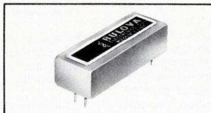
*Group delay crystal filters* offering perfect phase linearity for optimum data transmission are also available from Bulova. Overshoot is kept to 40 db (1%) below the steady state value. The filters provide distortion-free selectivity, at a maximum speed, and have a reduced error rate. Bulova's complete line of crystal filters meet all transmission specifications from 4 KHz to 150 MHz.
