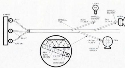
three individual signals. Electro Fiberoptics engineers are now trying to determine just how many different colors can be "multiplexed" over a single line. The possibility of combining the two concepts displayed is impressive: half a dozen 60-MHz signals could be transmitted over a spaghetti-sized cable that costs less than pennies a foot.
