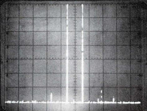
High Level Model M1K: With a +23 dBm  $f_L$  drive level and with  $f_{R1}$  and  $f_{R2}$  at 0 dBm, the Model M1K virtually eliminates all two-tone products from the 70 dB spectrum.
