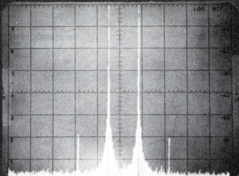
High Level Model M9D: With only a +20 dBm  $f_L$  drive level, the Model M9D suppresses the third order product by 60 dB and the fifth order product by more than 70 dB.
