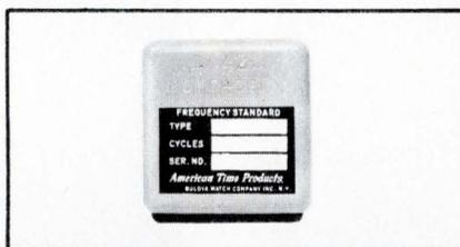
The news in *subminiature fork oscillators* is a unit which uses less than 5 ma. The oscillator, developed by Bulova and designated the FS-11-1, takes up about  $\frac{1}{2}$  cu. in. of space and weighs one ounce. Their units have accuracies up to  $\pm 0.0005\%$ , 90% reliability for 200,000 hrs. and logic circuit compatibility.
