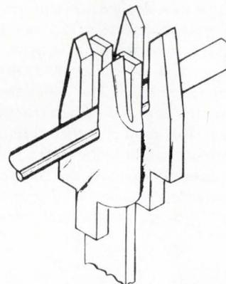
A new point-to-point daughter-board wiring system can be applied by hand or with a tape controlled machine. The inherent ease of wire removal and replacement makes this system especially suited for prototype wiring.
