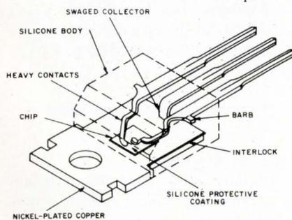
configurations, and thermal-cycling capability) and illustrations show the internal structure of the basic package, lead-configuration options, and device performance ratings. RCA Solid State Div., Box 3200, Somerville, N.J. 08876.
