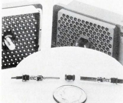
into a cup and lock into the connector block. From the rear or wire side, the seal is now a pressure-sensitive membrane, much like the cup of an air or hydraulic cylinder, which increases its sealing capability as pressure differences between the inside of the con-
