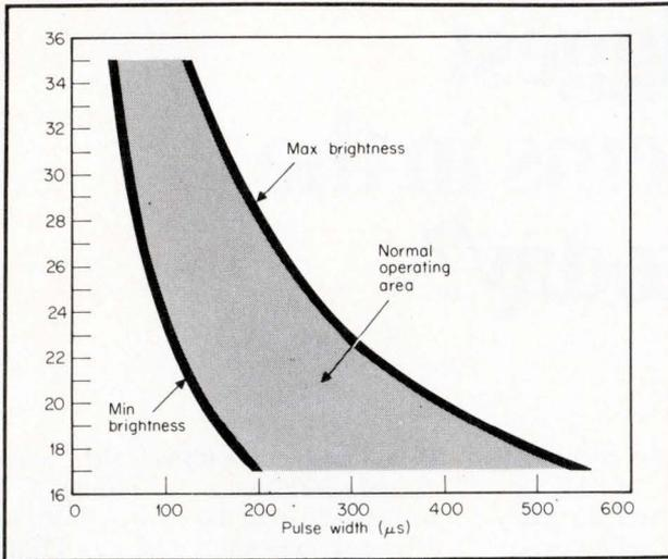
**Display pulse width vs voltage.** The Hoffmann display subsystem typically operates at 27 V and 175  $\mu$ s pulse width every 6,400  $\mu$ s.
