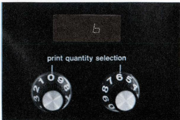
**Prototype.** Operation of this LED display is the same as on a Xerox 4000 copier. The counter indicates copies selected until the "start-print" button is pushed. Then it resets to zero and counts until that number is reached.
