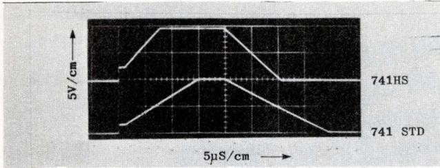
This high-speed version, the 741HS, boasts a 4 to 1 improvement in the standard 741 slew rate, plus improved input offset ( $I_{OS}$ ) and input bias ( $I_b$ ) currents.
