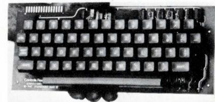
The model 7100 low-cost ANSI typewriter keyboard features a dynamically scanned MSI electronic encoding system and redundant gold contact BI-PAC switches. All circuitry and key-switch modules are on a single PC board. Features include full ASCII coding (shifted, unshifted, control and control/shift), 2-key roll-over interlock, and low power consumption (less than 300 mA.). \$49 in 5000 quan., stock to 8 wk. Jim Antrim, Controls Research Corp., 2100 S. Fairview, Santa Ana, CA 92704.
