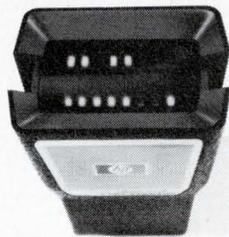
**10528A Logic Clip** — Eliminating the cumbersome voltmeter route, this unique device clips directly onto an IC and 16 LED's tell you the state of all 14 or 16 pins instantaneously. No cables, no power connections. Auto-seeking of  $V_{CC}$  and ground. Only \$125.
