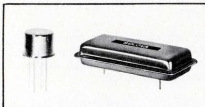
A new series of *highly miniaturized coldwelds* having a broader frequency output is now available. The units — developed by Bulova — feature tolerances as close as 3 ppm of nominal on initial adjustment, and aging rates up to 3 pp  $10^8$  per week. In the TO-5 can, for example, with a frequency range of 500 KHz to 160 MHz, Bulova coldwelds have a tolerance of  $\pm 0.015\%$  (from  $-55^\circ\text{C}$  to  $+105^\circ\text{C}$ , or to specs.) Aging is  $1 \times 10^{-7}$ /week after 4 weeks.
