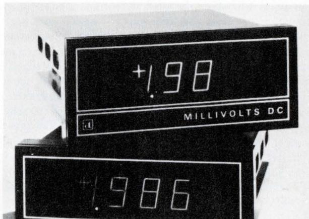
Data Technology's entry is the under \$100 DPM sweepstakes offers full-scale readings of 199 or 1999 and your choice of unipolar or bipolar input. Originally developed for LED displays, Data Technology reports that they changed to the Sperry gas discharge display as a result of a customer preference poll.
