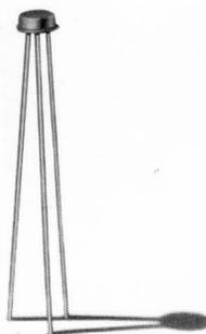
Our 2N5066 has a 4-ohm typical (8-ohm maximum)  $R_{ON}$ . We have to admit, it does have an offset voltage, but it's only 300 microvolts typical (1 millivolt maximum). The off-current is still 1 nano-amp maximum, and it takes less than 1 volt to turn it on. The device does draw some current in the on state (less than 1 milliamp), but that's OK in most cases, because the signal source impedance is usually less than 1 ohm.
